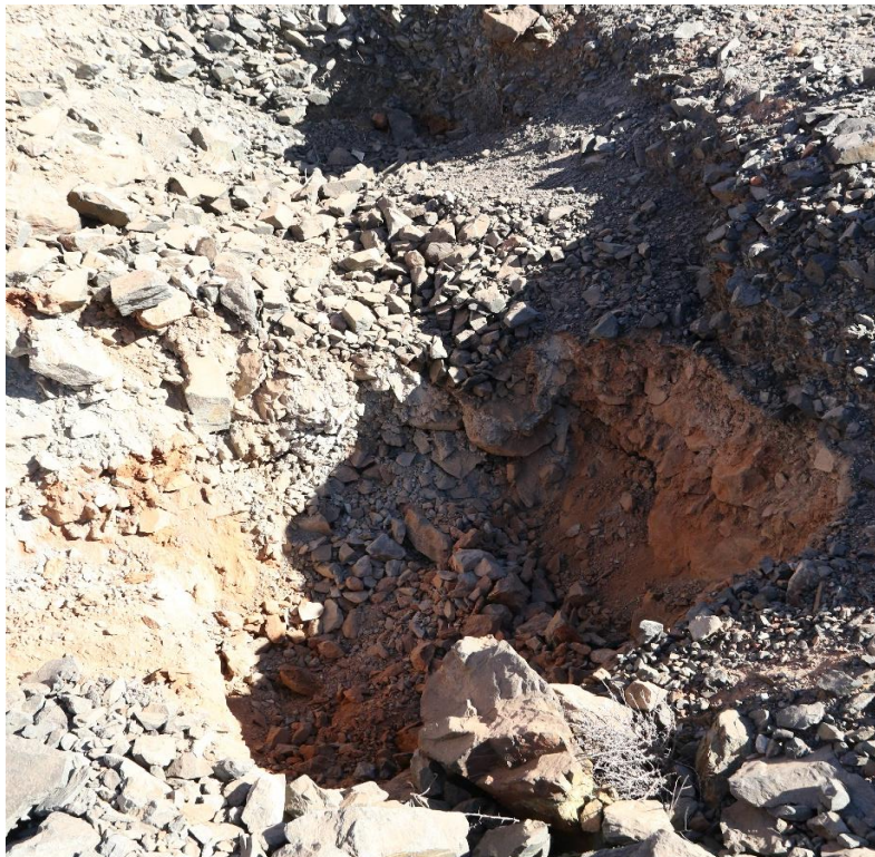
Photograph 21: Trench exposing natural ground either edge of subsidence envelope
