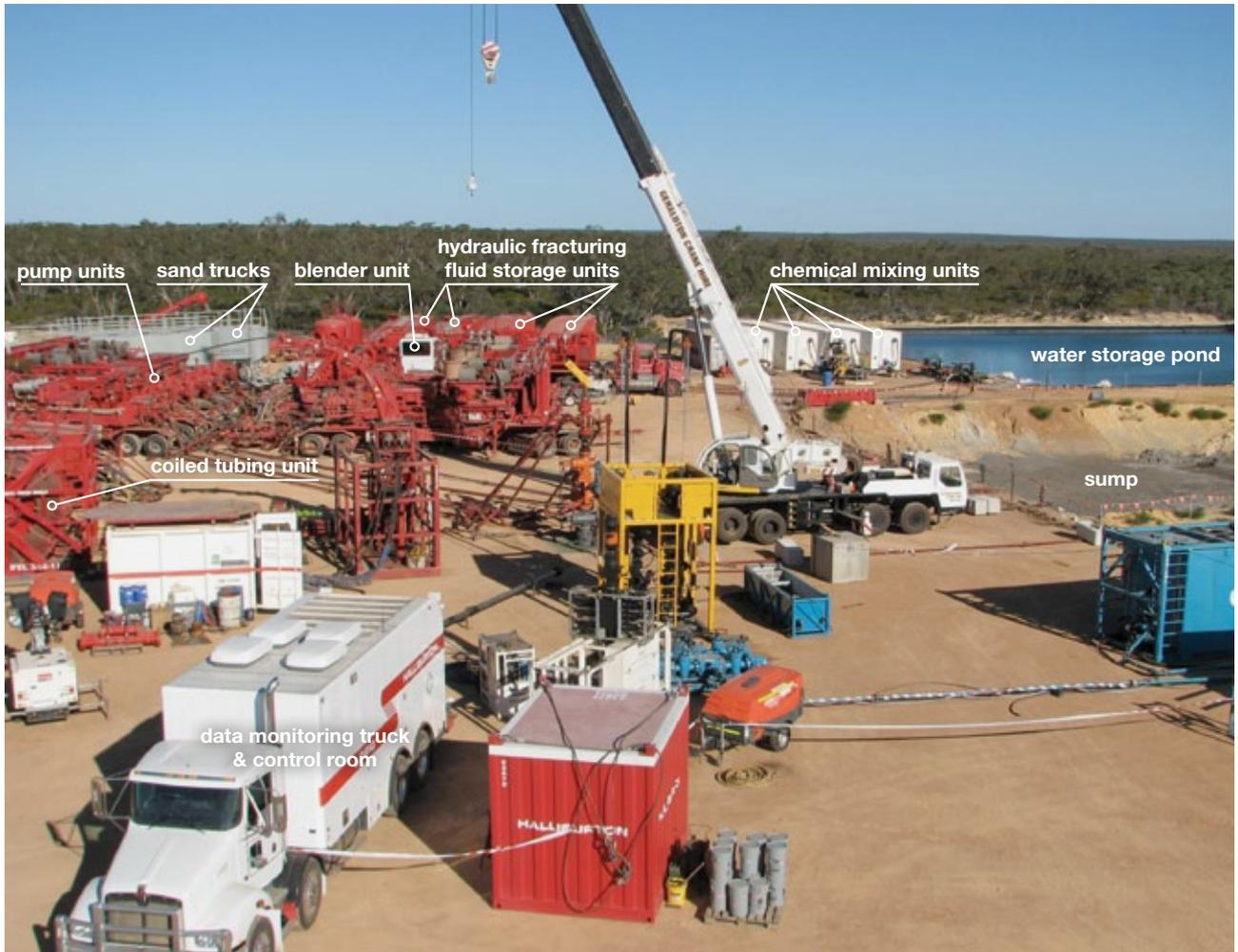
**Figure 4:** Hydraulic fracture stimulation equipment at the Arrowsmith 2 well site in the northern Perth Basin (courtesy of Norwest Energy Ltd)
