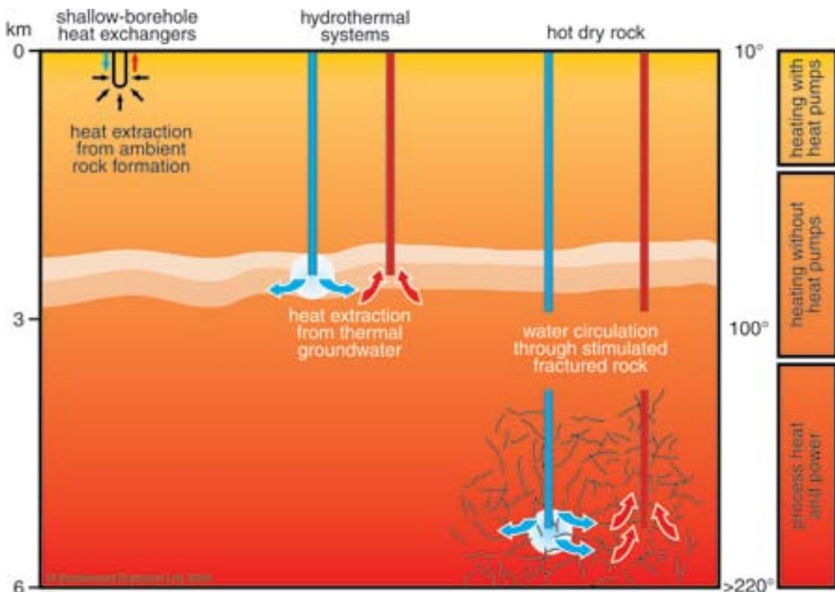
Figure 29. Types of geothermal resources from the Earth's heat. All systems show extraction wells (red) and injection wells (blue) (Courtesy of Geothermal Explorers Ltd)
