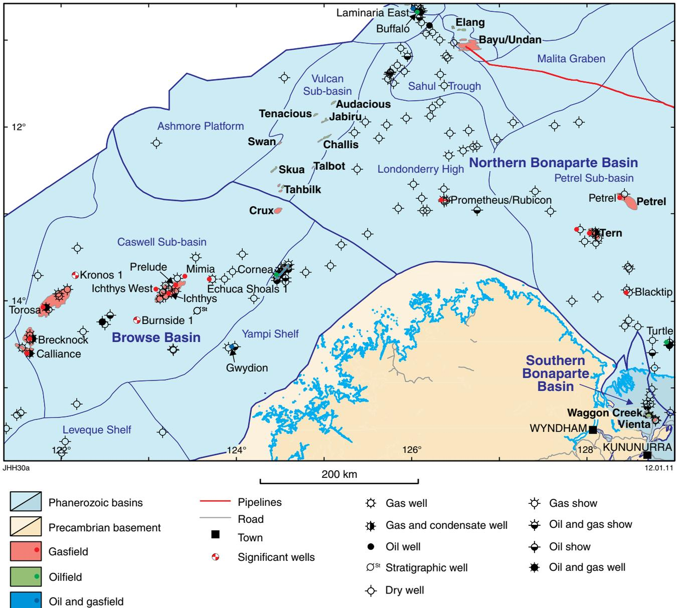
Figure 11. The Bonaparte Basin, showing tectonic units, exploration wells, pipelines and petroleum fields
