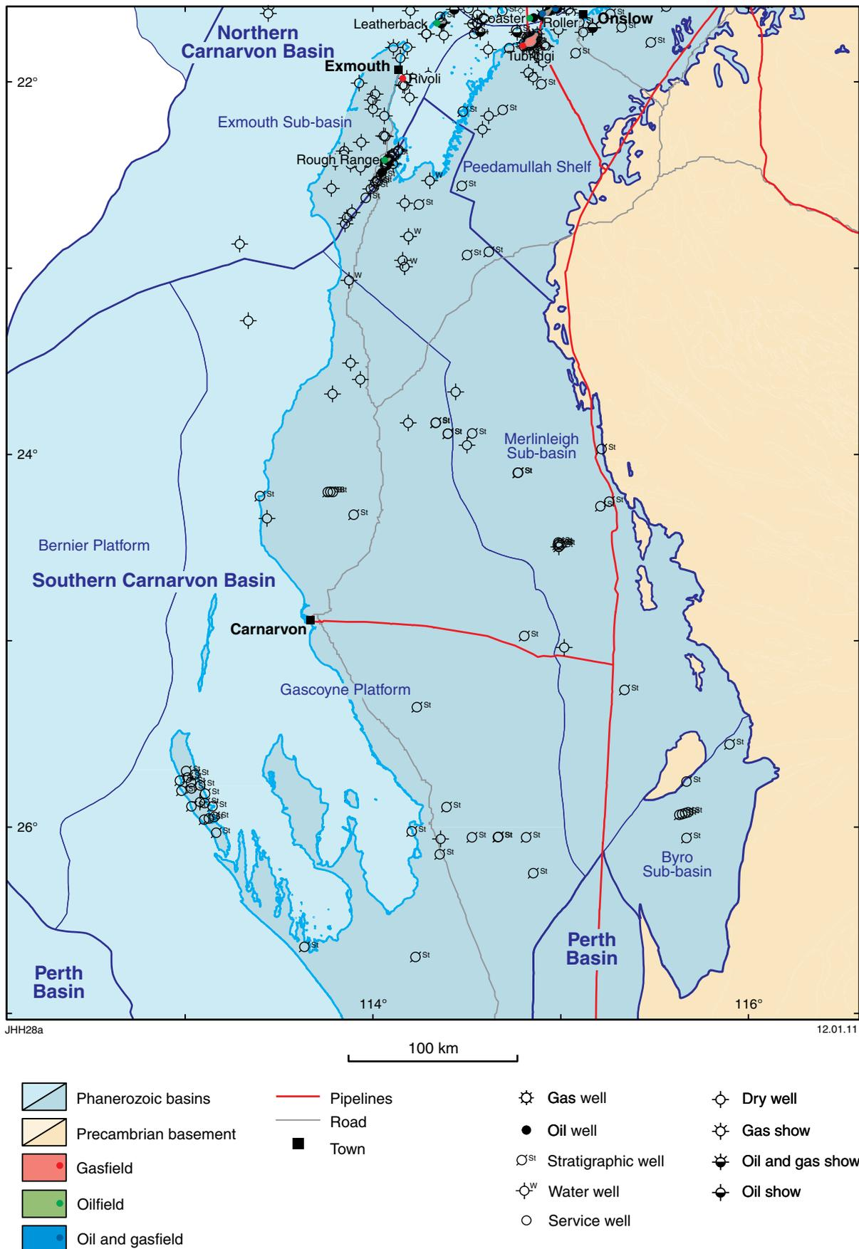
Figure 21. The Southern Carnarvon Basin, showing tectonic units, pipelines, fields and petroleum wells
