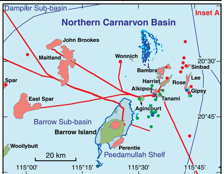
Figure 19. The Northern Carnarvon Basin, showing tectonic units, pipelines, fields and petroleum wells
