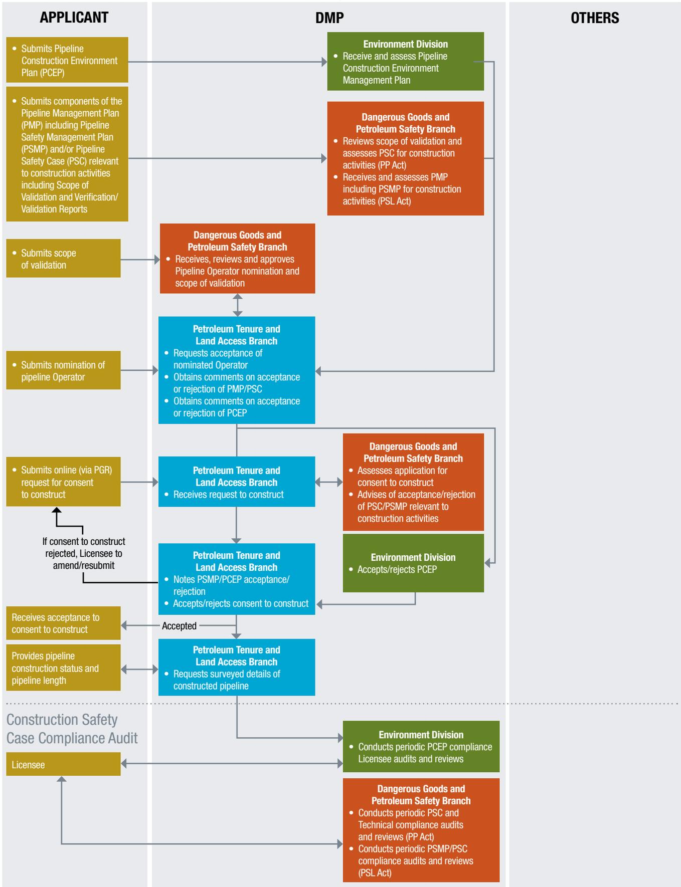
Figure 47. Pipeline Consent to Construct Approval Process
