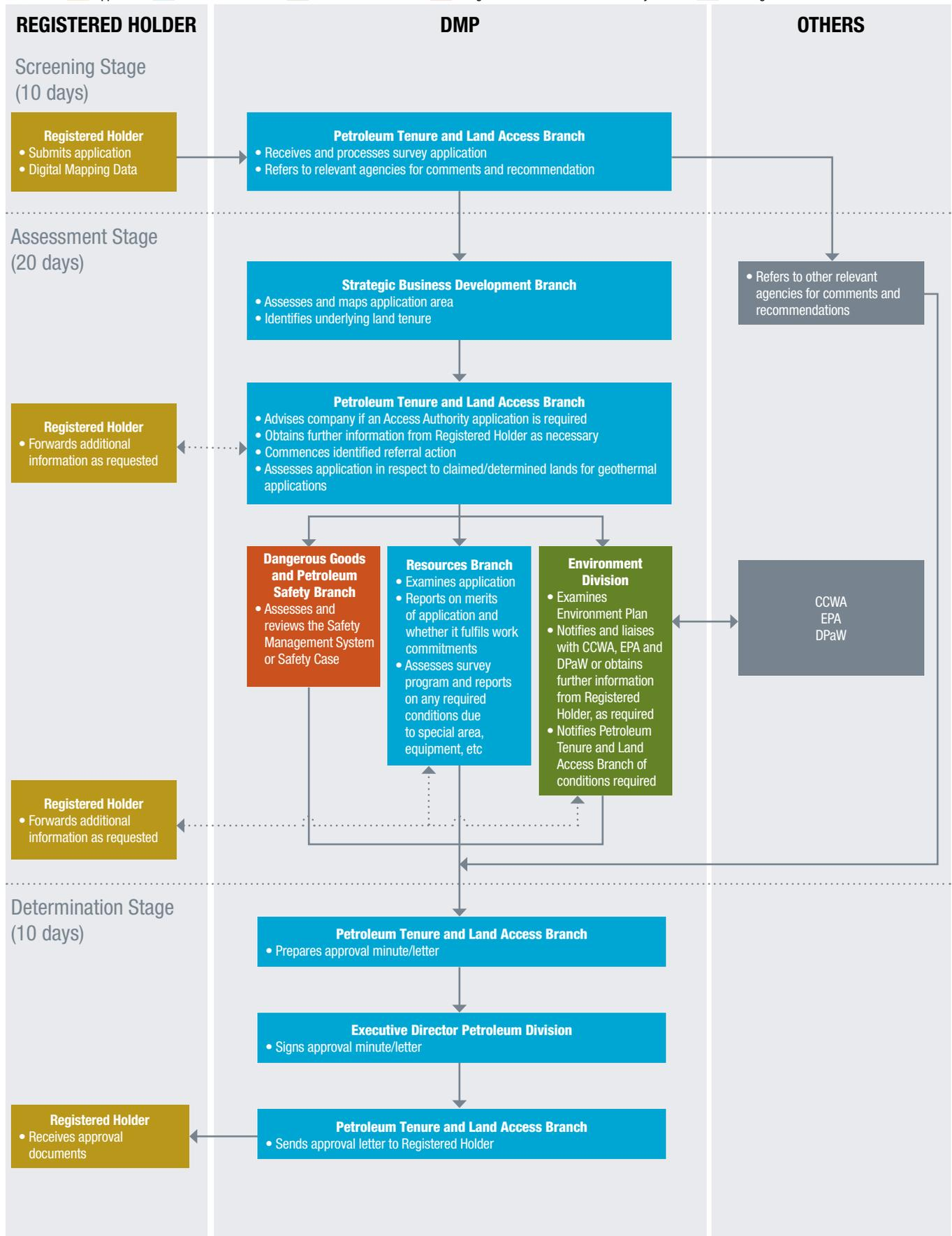
Figure 44. Petroleum/Geothermal Survey Application Approval Process
