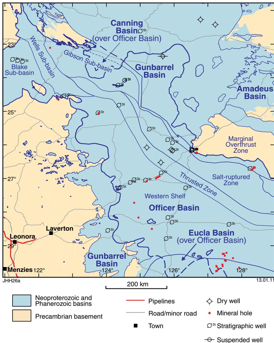
Figure 23. The Officer Basin, showing tectonic units and exploration drillholes of interest
