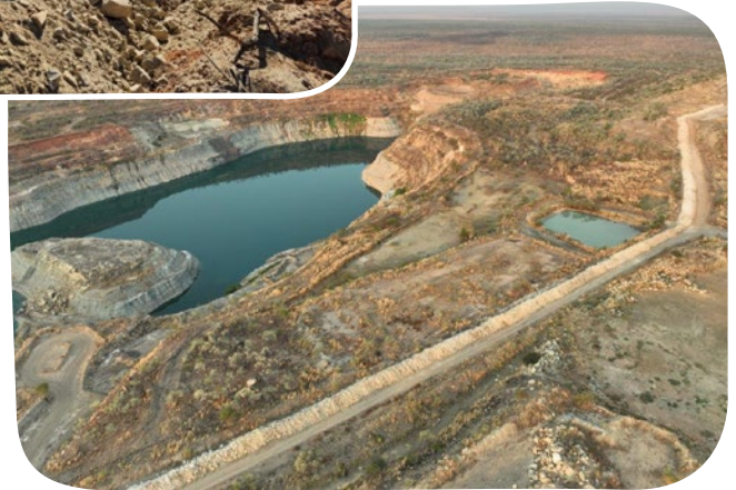
Safety bunds established around the pit voids.
