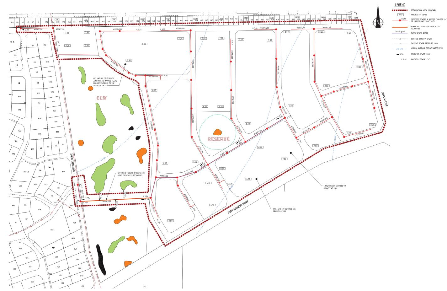
Figure 18. Concept Sewer Layout (Porters)
