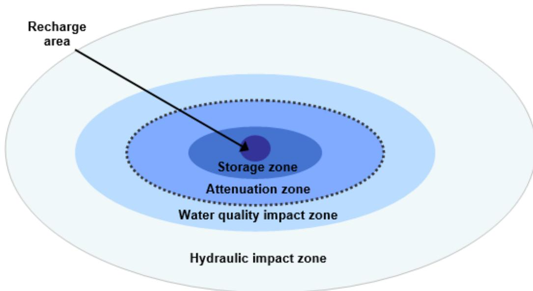
*Figure 3. Schematic diagram of a MAR management zone (Australian Guidelines for Water Recycling, Managed Aquifer Recharge, NRMCC, EPHC, NHMRC, 2009)*
