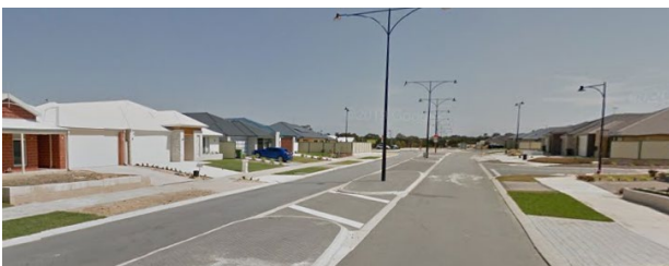
Figure 8. Residential streetscape in Hammond Park where hardscaping dominates due to insufficient space for street trees and numerous breaks in the median for access to crossovers
