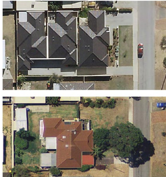
Figure 9. Infill development (Spearwood) demonstrating reduced landscaping and increased hardstanding with redevelopment (top photo)
