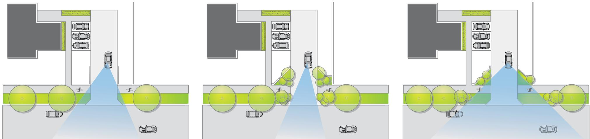
*Inadequate truncations are provided resulting in poor sight lines.*
