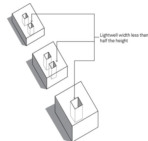
**Figure G2.2b** Lightwell width to height ratio
