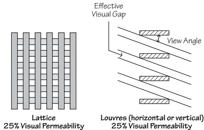
**Figure 61** Example of screening by which visual permeability can be limited. Note that a view angle of 45 degrees to the side is the limit of the cone of vision as defined in the R-Codes Volume 1, and no screening is required outside these limits
