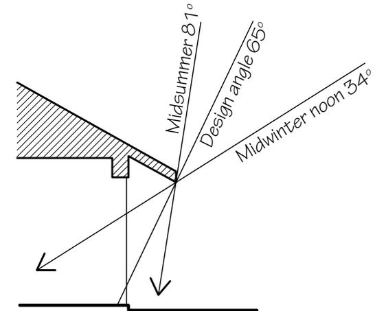
**Figure 70** Calculated eaves overhang on north side, Perth
