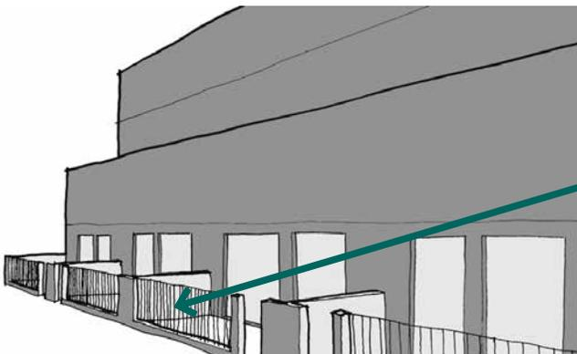
Fencing is permeable and allows visual connection with the street while providing security and delineating private and public property.
