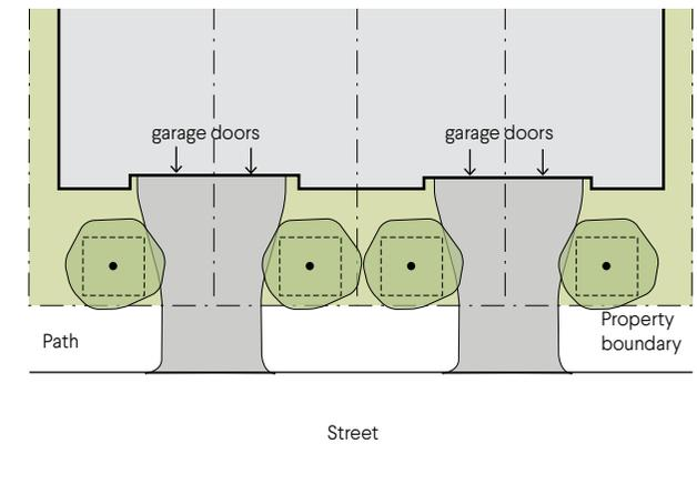
**Figure G3.7a** Pairing of vehicle access points
