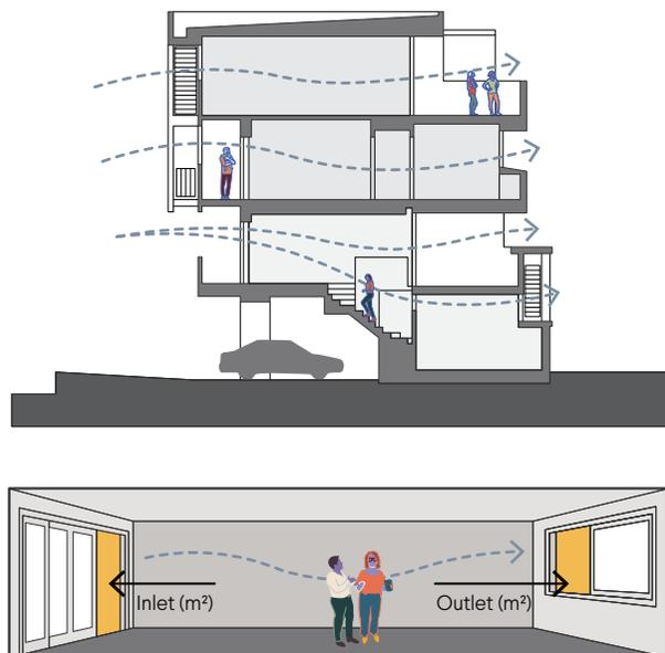
**Figure G2.2a** Natural ventilation for passive cooling
