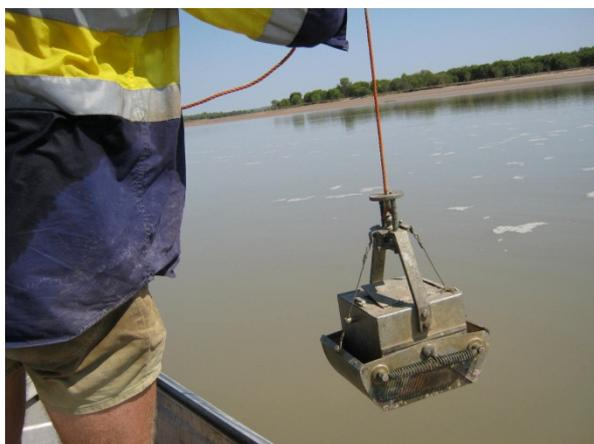
**Plate 1.** Collecting sediment samples at EST03 with an Eckman-Birge grab sampler.
