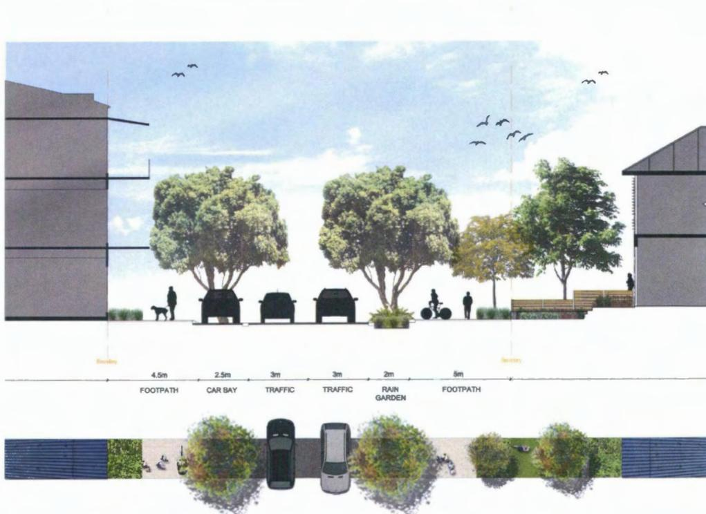
Figure 39\_Section through a Local Street (without the BRT)
