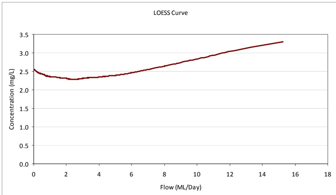
**Figure C-3:** Total nitrogen LOESS curve with and without measured data
