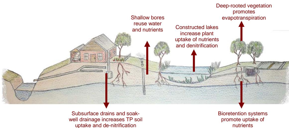
**Figure 6-7:** Processes that reduce nutrients by means of infiltration and evaporation in 'new' catchments
