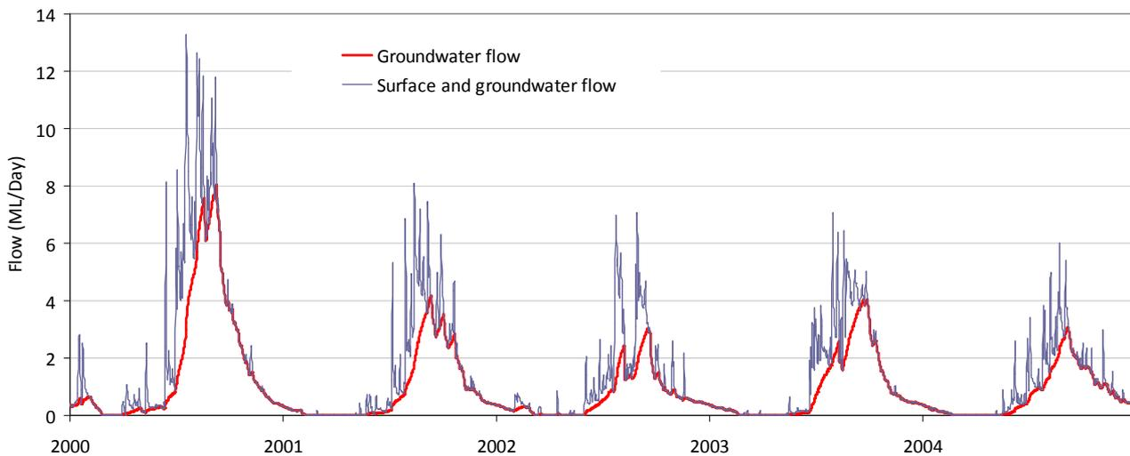
**Figure 5-8:** Baseflow separation results for the daily streamflow for Bartram Road buffer lake inflow gauging station (616083) for the years 2000 to 2004
