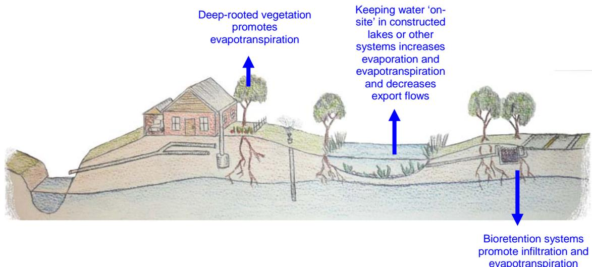
**Figure 6-6:** Processes that reduce flow by means of infiltration and evaporation in WSUD catchments
