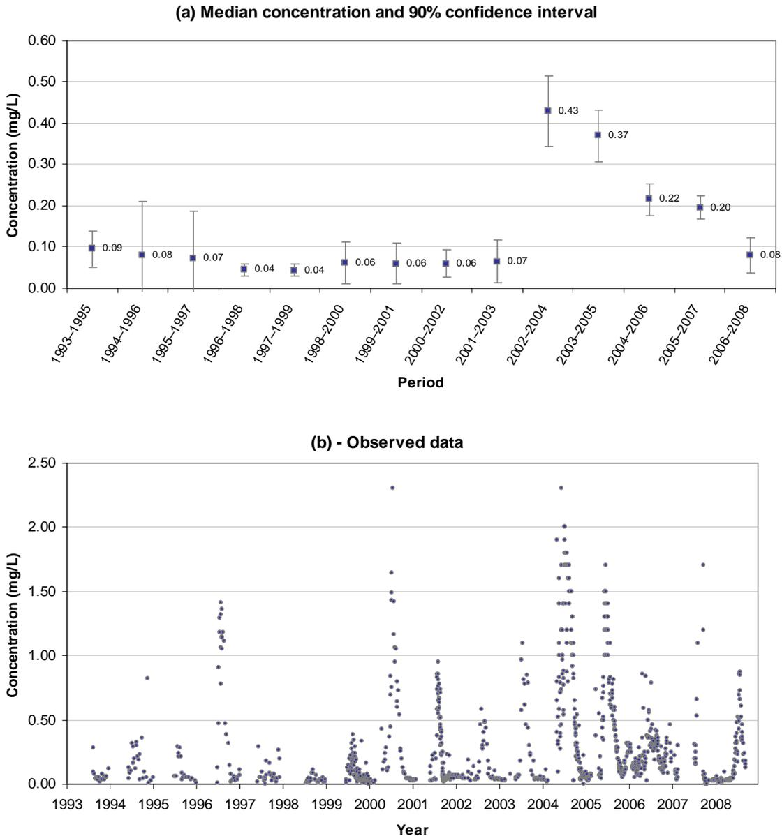
**Figure 5-5: Three-year median NO<sub>x</sub> concentrations and 90% confidence intervals (a), and observed NO<sub>x</sub> concentration data (b)**
