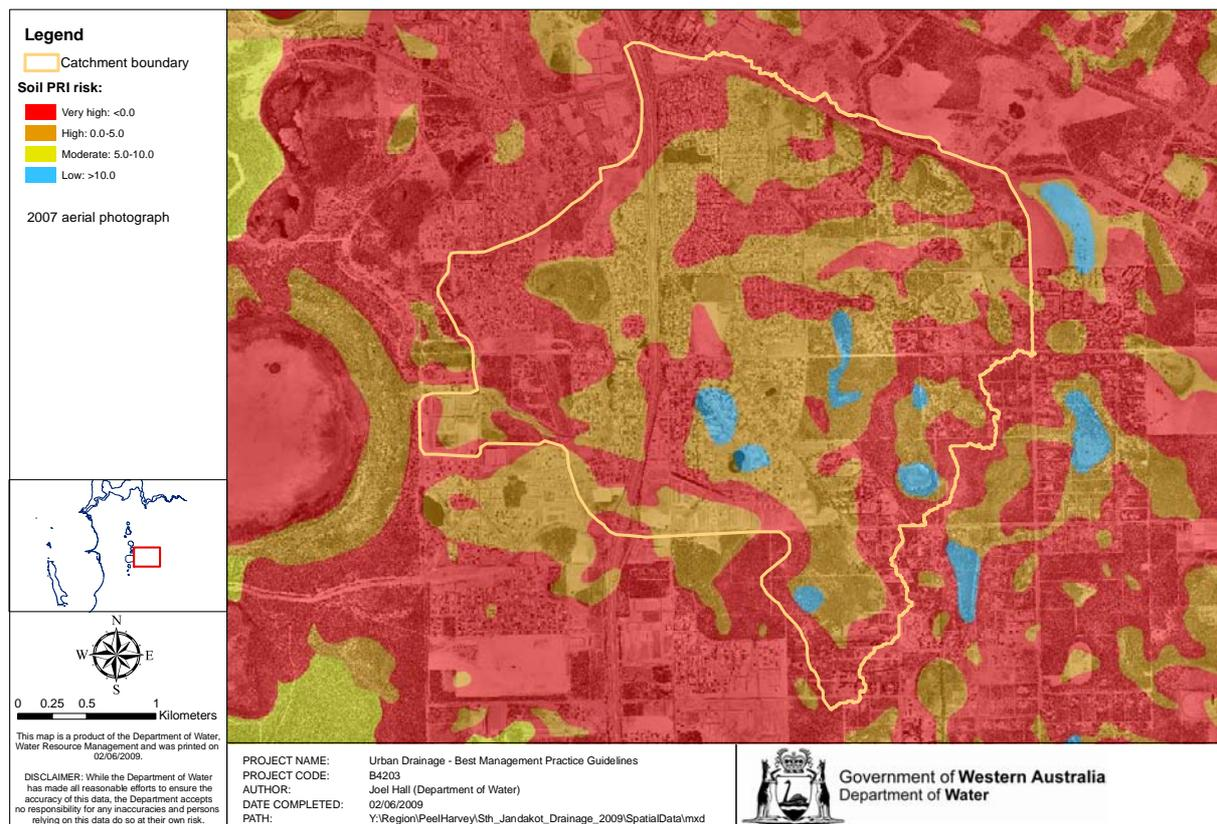
Figure 3-12: Soil phosphorus retention index (PRI) map of the Bartram Road catchment
