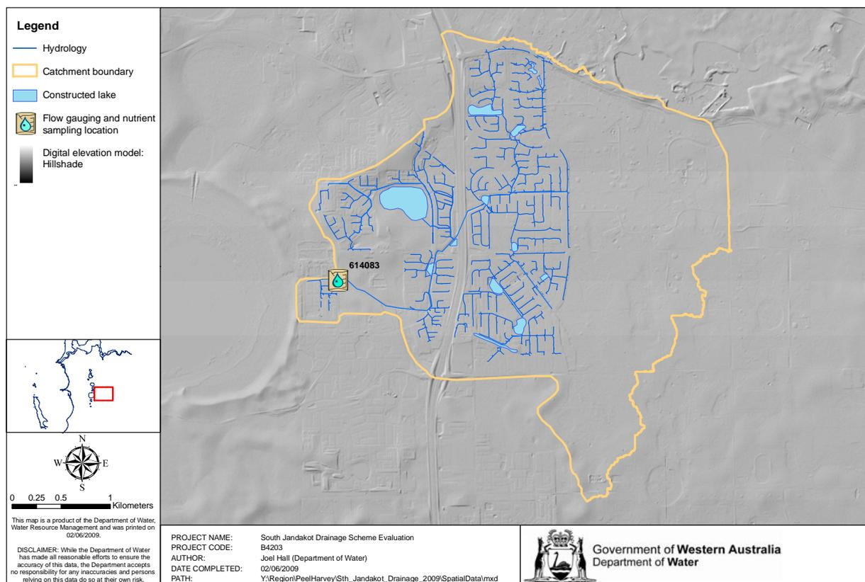
**Figure 3-2: Drainage network and topography of the Bartram Road catchment**
