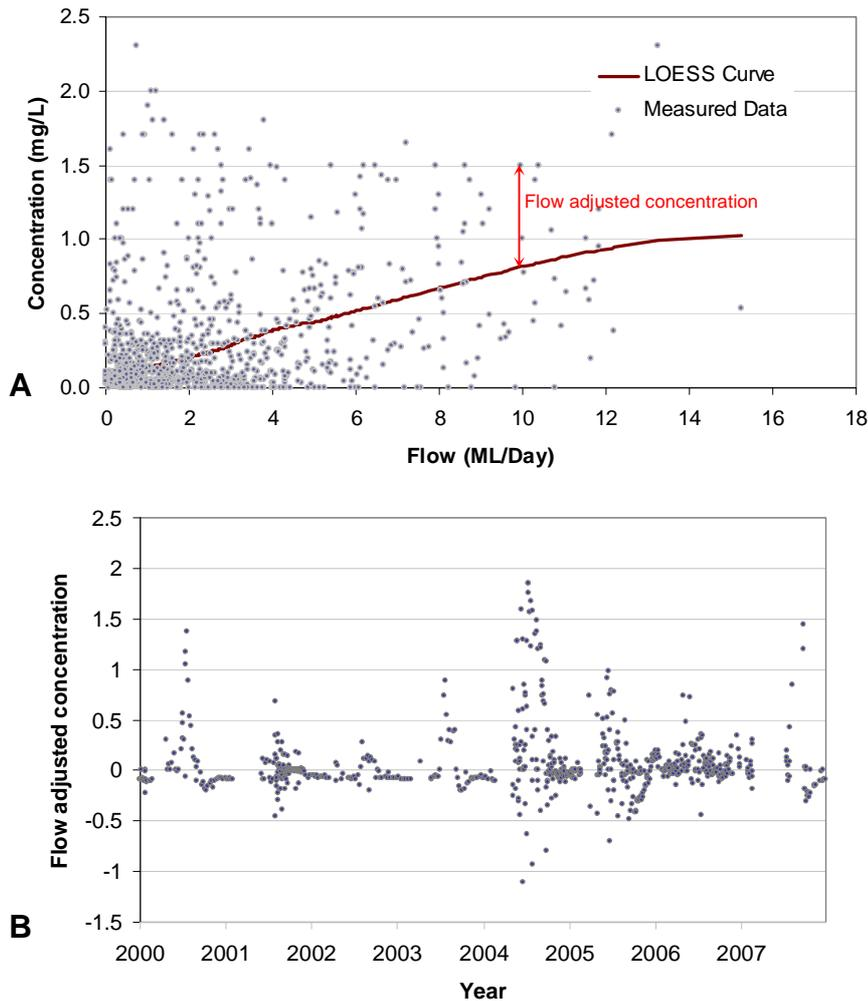
**Figure B-3:** The flow response plot shows whether a relationship exists between discharge and nutrient concentration (A). The flow-adjusted concentrations (or residuals) are the difference between observed and modelled (LOWESS) concentrations (B)
