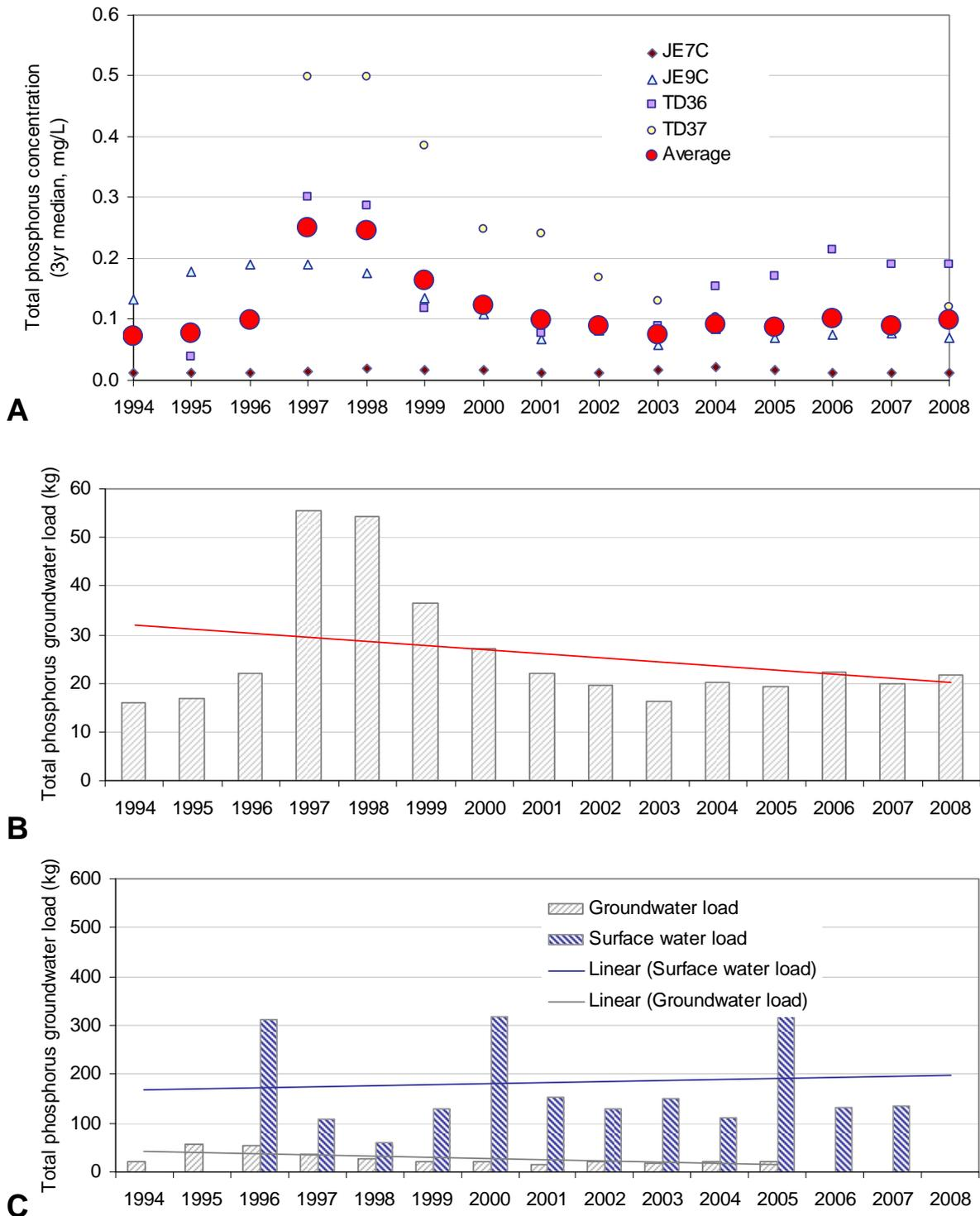
**Figure 5-14:** Three-year median concentration from each of the bore locations (A), the calculated annual groundwater load (B) and the comparison between surface water and groundwater loads (C) for total phosphorus
