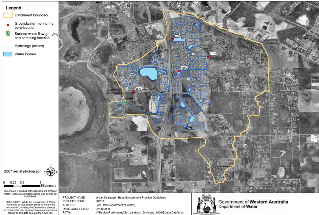
**Figure 3-14:** Groundwater monitoring bore locations and the surface water flow gauging and nutrient sampling location in the Bartram Road catchment
