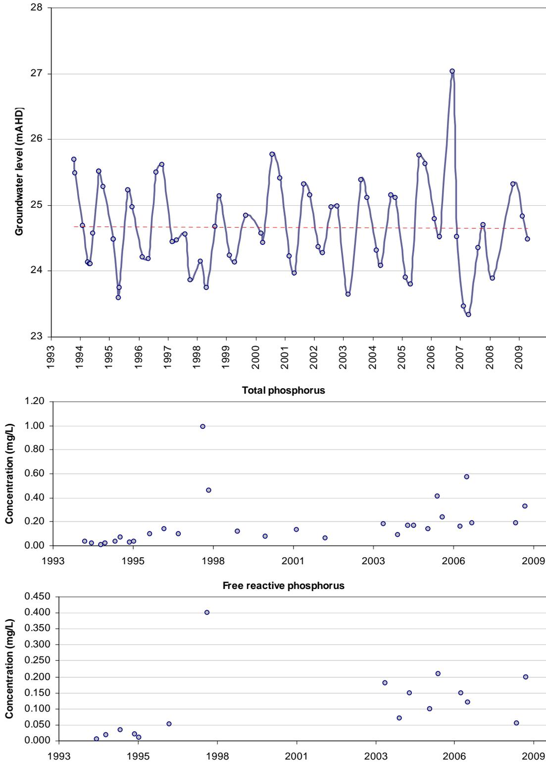
Figure E-5: Water level, TP and SRP concentration time-series for TD36
