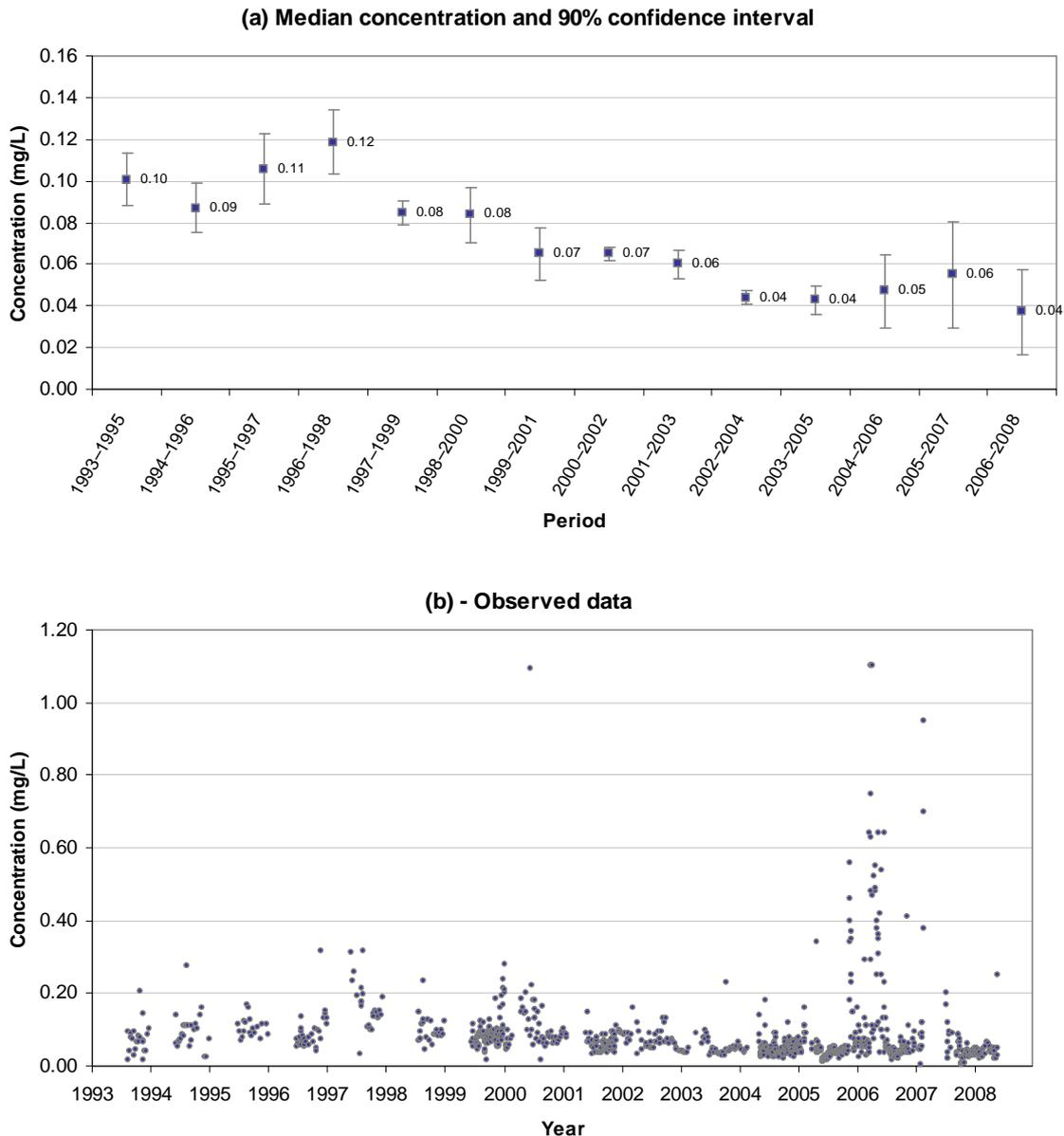
**Figure 5-6:** Three-year median  $\text{NH}_4/\text{NH}_3$  concentrations and 90% confidence intervals (a), and observed  $\text{NH}_4/\text{NH}_3$  concentration data (b)
