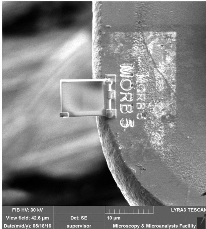
*Figure 3-11 Typical TEM lamellae cut using the focused ion beam (FIB) facility at the Microscopy and Microanalysis Facility at the John de Laeter Centre, Curtin University. The lamella is ~5 micrometres in size, and a few 10s of nanometres thick.*
