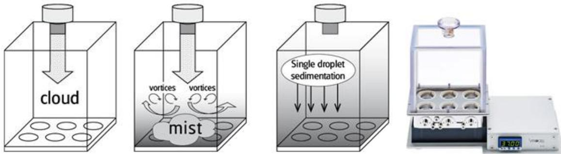
Figure 3-14 Cloud chamber – showing the condensation/coagulation of a cloud of aerosol.
