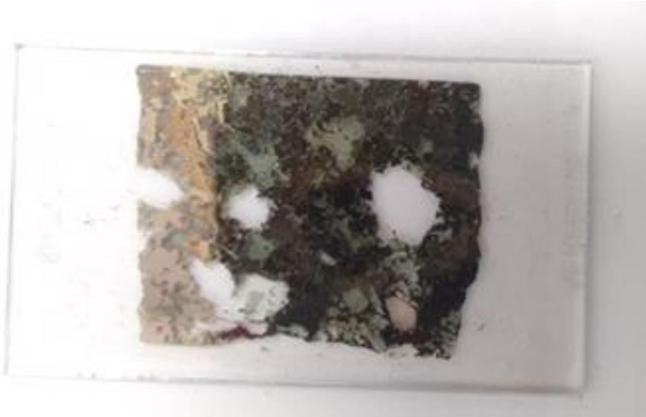
Figure 3-9 *40 × 20 mm thin section of rock used for optical microscopy, SEM, EPMA, and as a source of needles and foils for TEM and APT.*
