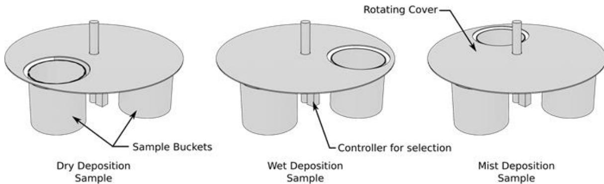
Figure 3-16 The '3 Bucket' deposition sampler.
