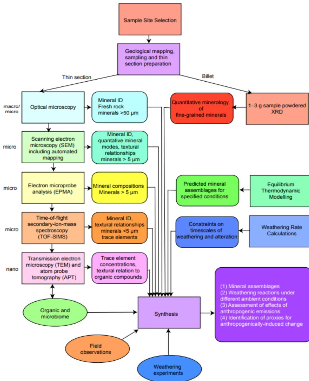
Figure 3-8 Overview of the inorganic geochemistry workflow.
