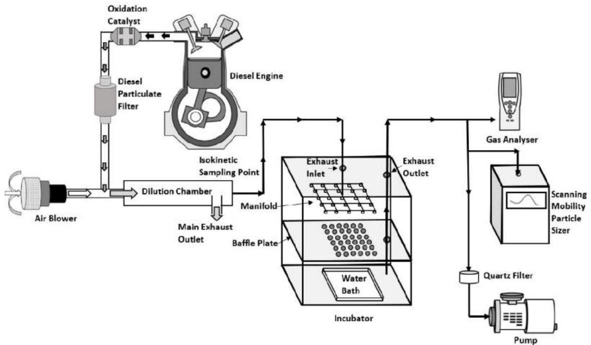
Figure 3-15 Exposure system for gaseous and particle deposition. Can be operated with a range of air pollutants in addition to combustion engine exhaust (Landwehr et al., 2019).
