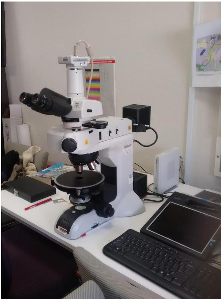
*Figure 3-10 Nikon Eclipse LV100N optical microscope for identification of minerals in the fresh rock and preliminary investigations of the weathered rind.*
