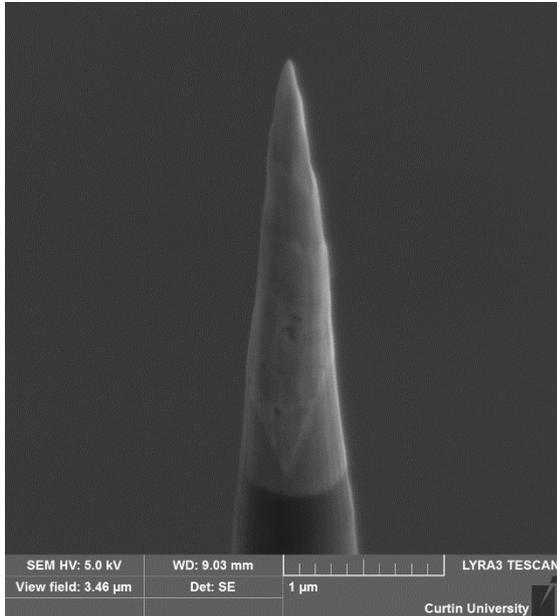
*Figure 3-12 Typical atom probe needle cut using the focused ion beam (FIB) facility at the Microscopy and Microanalysis Facility at the John de Laeter Centre, Curtin University. The needle is <2 μm long.*
