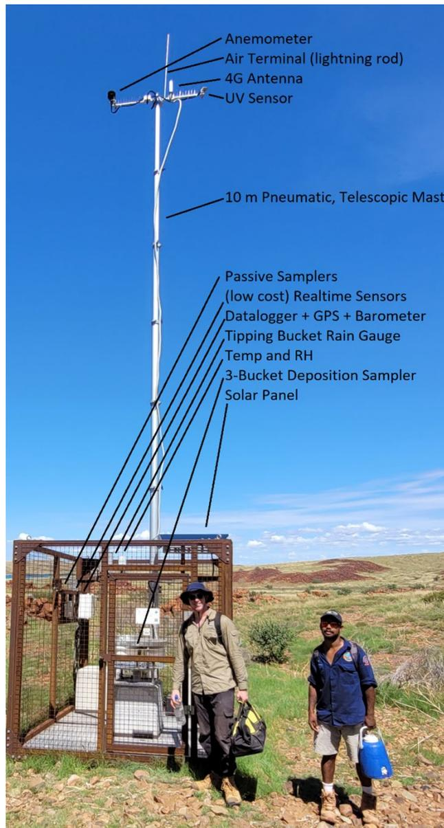
Figure 5-2: *Passive AQM (AQ12) showing key components of the monitoring system. Ronald Fellows-Smith and MAC Ranger Kasziem Bin Sali shown post installation of electronics*
