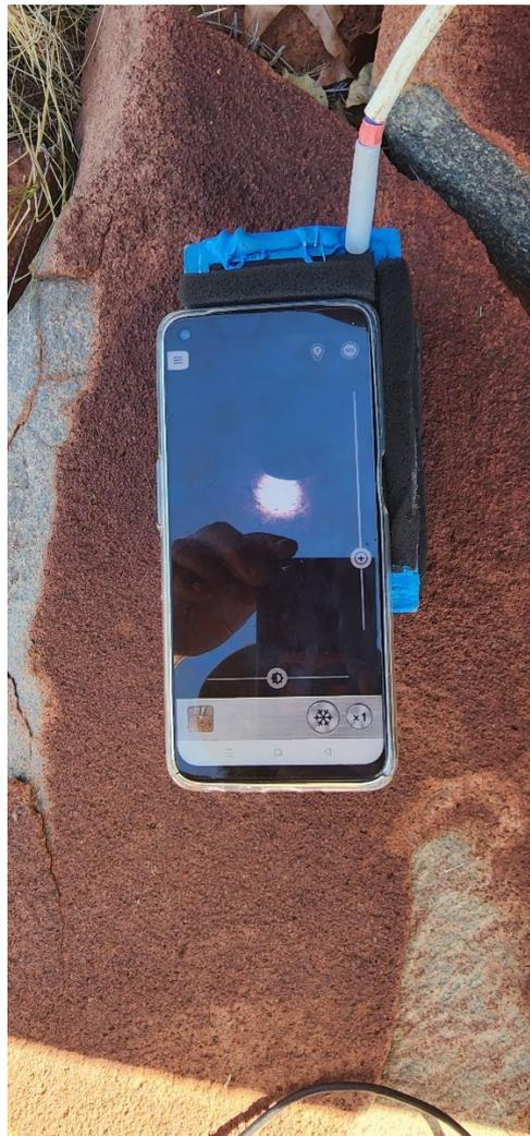
*Figure B-6: MAC Ranger Kasziem bin Sali aligns the spectrometer probe by comparing the macro features visible on the active camera at left with the reference location viewed on the static image in the right- hand phone.*
