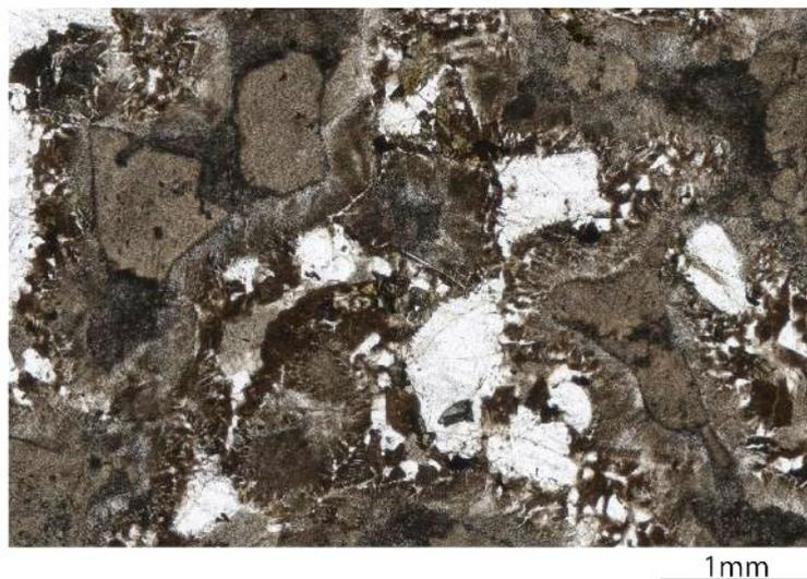
Figure 4-23: Photomicrograph in plane-polarized light of granite sample RS02\_GRT showing sericitized plagioclase (light brown). A coronitic texture of chlorite (and biotite?) surrounding plagioclase of the rock is also visible.
