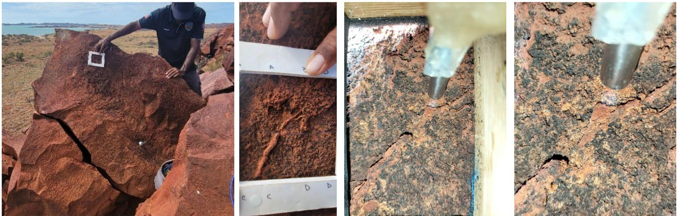
*Figure B-5: An abridged sequence of images that locate the grid cell on the whole rock, leading to the final macro images of the probe and light source. Note that the first macro image has stray light entering, blocked out prior to taking a reading.*
