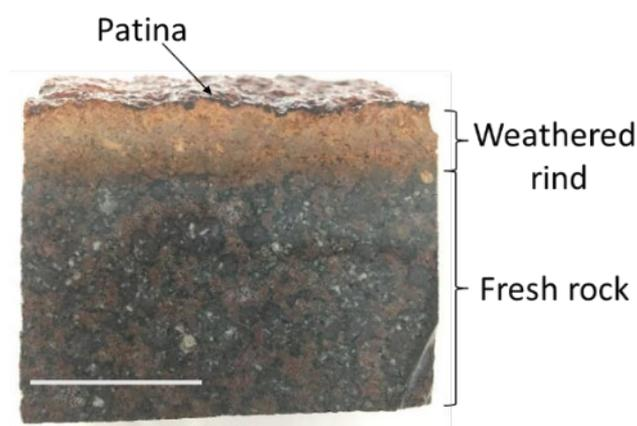
Figure 4-21: Cross section of the granophyre sample EX02\_GPH showing the three-layer structure of the rock from Donaldson (2011). Scale bar is 20 -mm.
