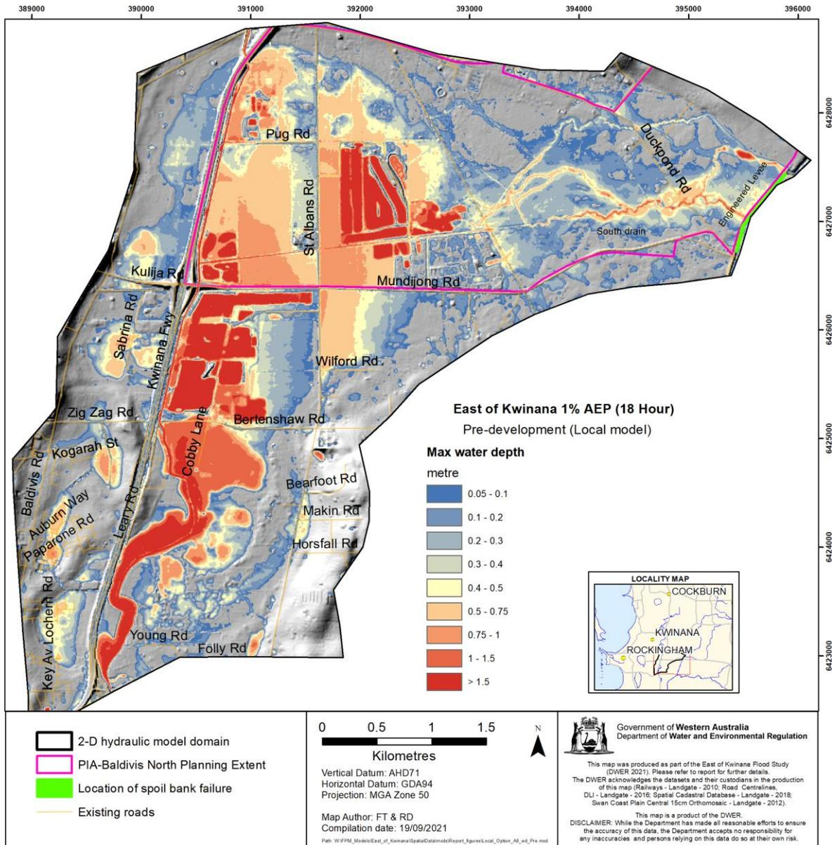
Figure 11 Local model 1% AEP pre-development flood map
