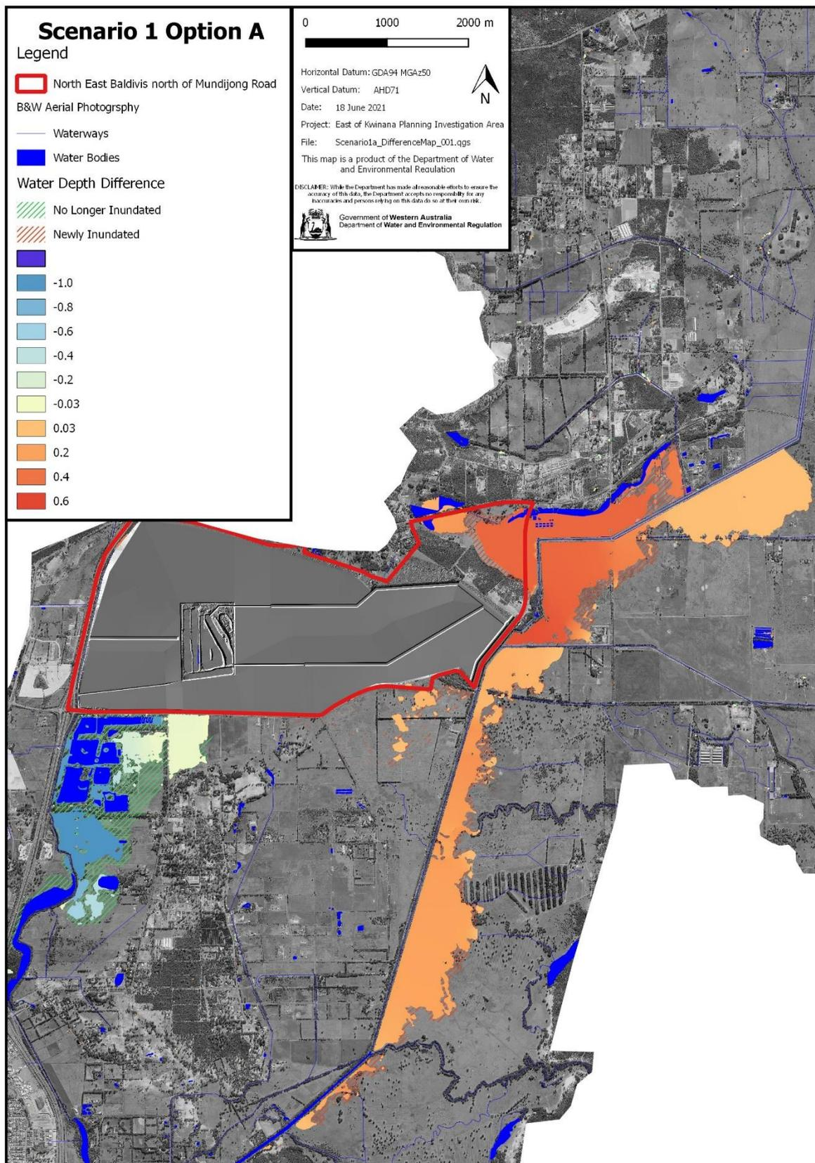
Figure 15 Scenario 1 (Option A) water depth difference map
