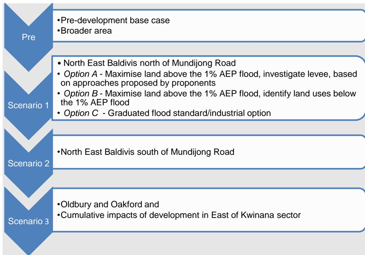
Figure 4 Flood modelling framework for investigating East of Kwinana
