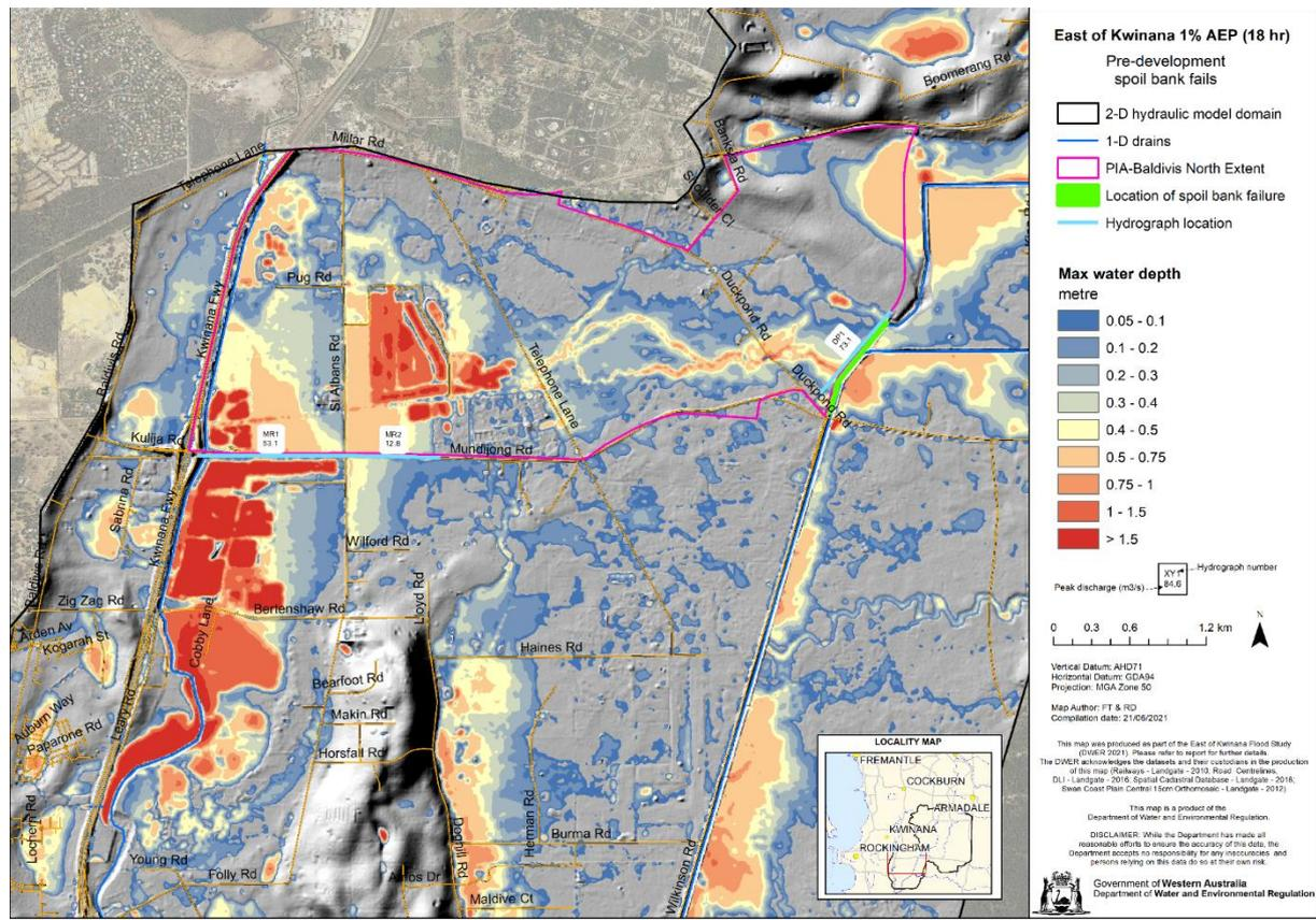
Figure 10 Pre-development 1% AEP flood map (spoil bank fails)
