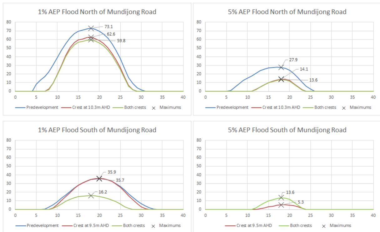
Figure 42 Scenario 2 North East Baldvis potential 1% AEP inflows with integrated development
