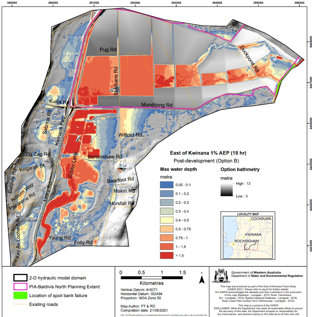
Figure 24 Scenario 1 Option B Plus flood modelling results
