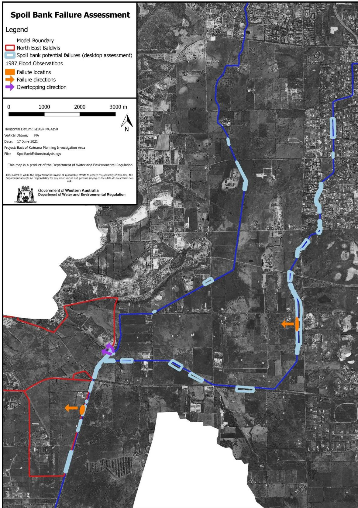
Figure 8 Spoil bank failure assessment and failures observed in 1987 flood
