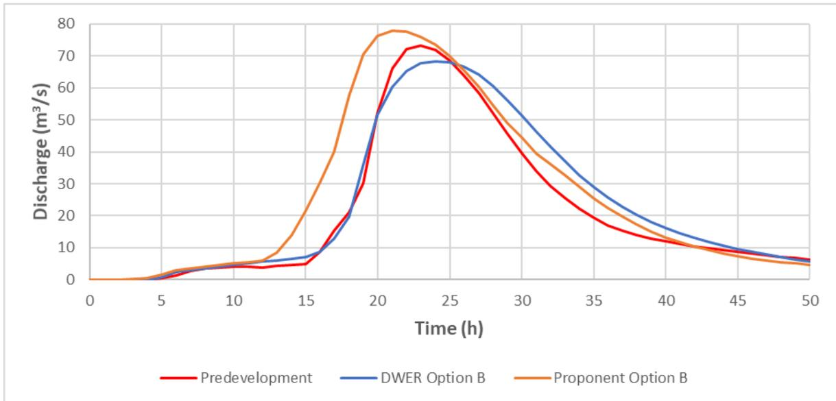
Figure 25 Proponent-driven Option B total discharge at Mundijong Road
