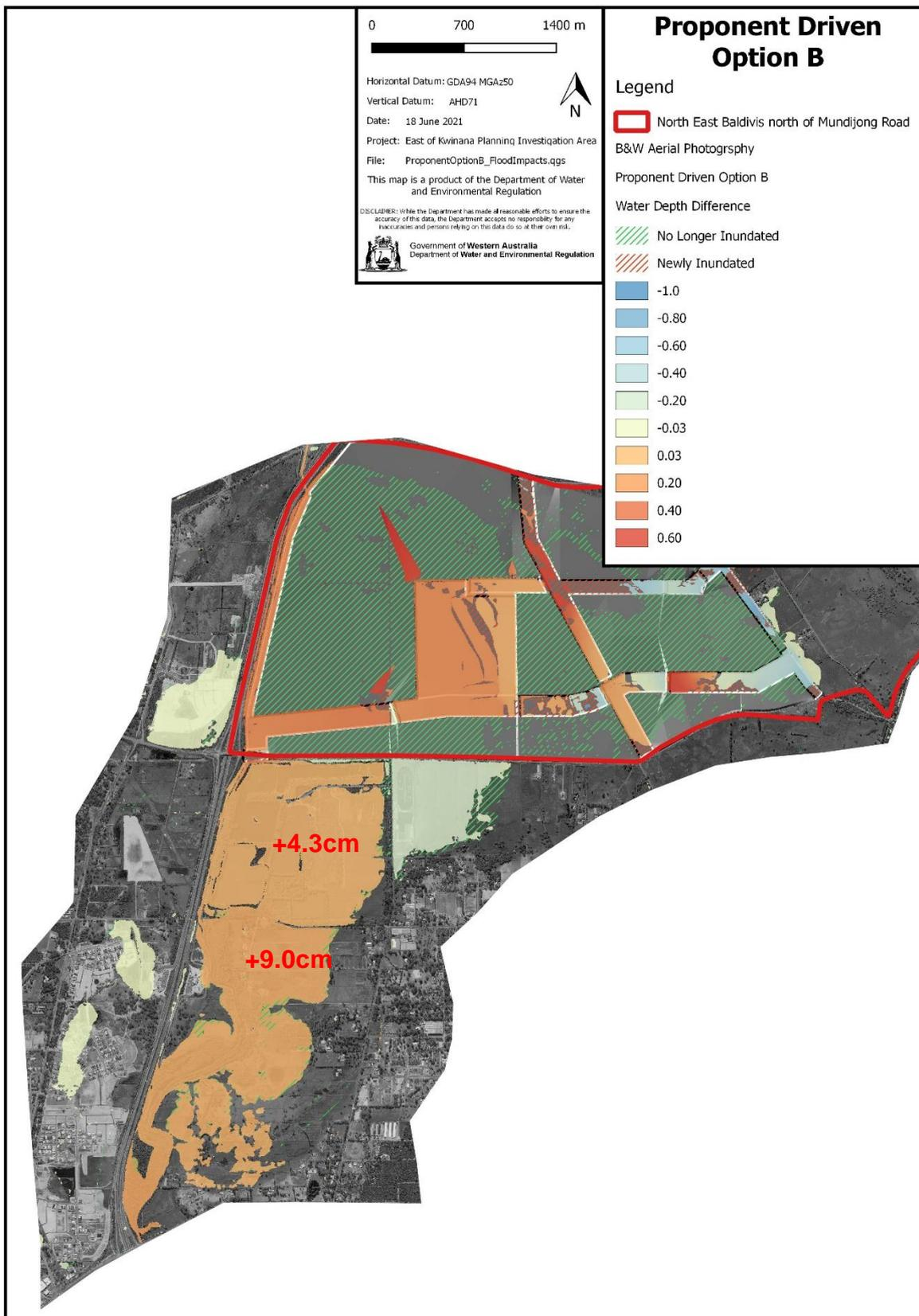
Figure 27 Proponent-driven Option B flood impacts
