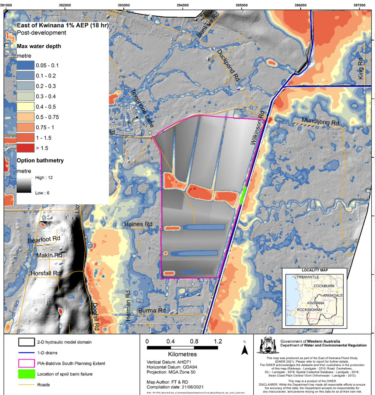
Figure 45 Scenario 2 post development flooding
