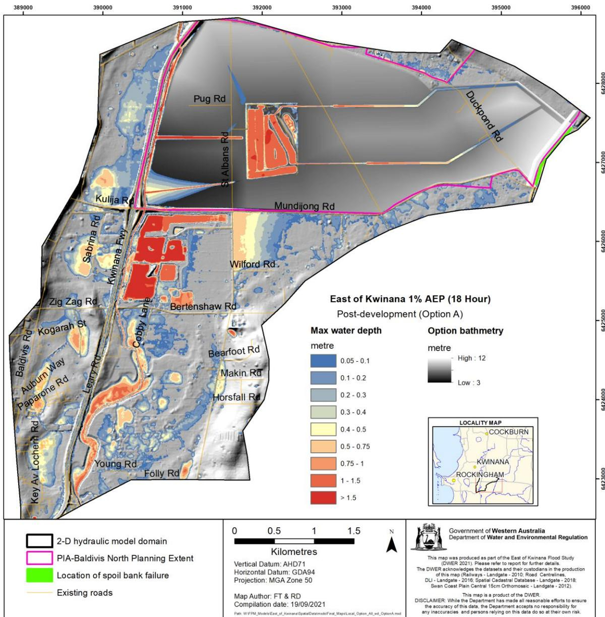
Figure 14 East of Kwinana 1% AEP Scenario 1 Option A local flood map
