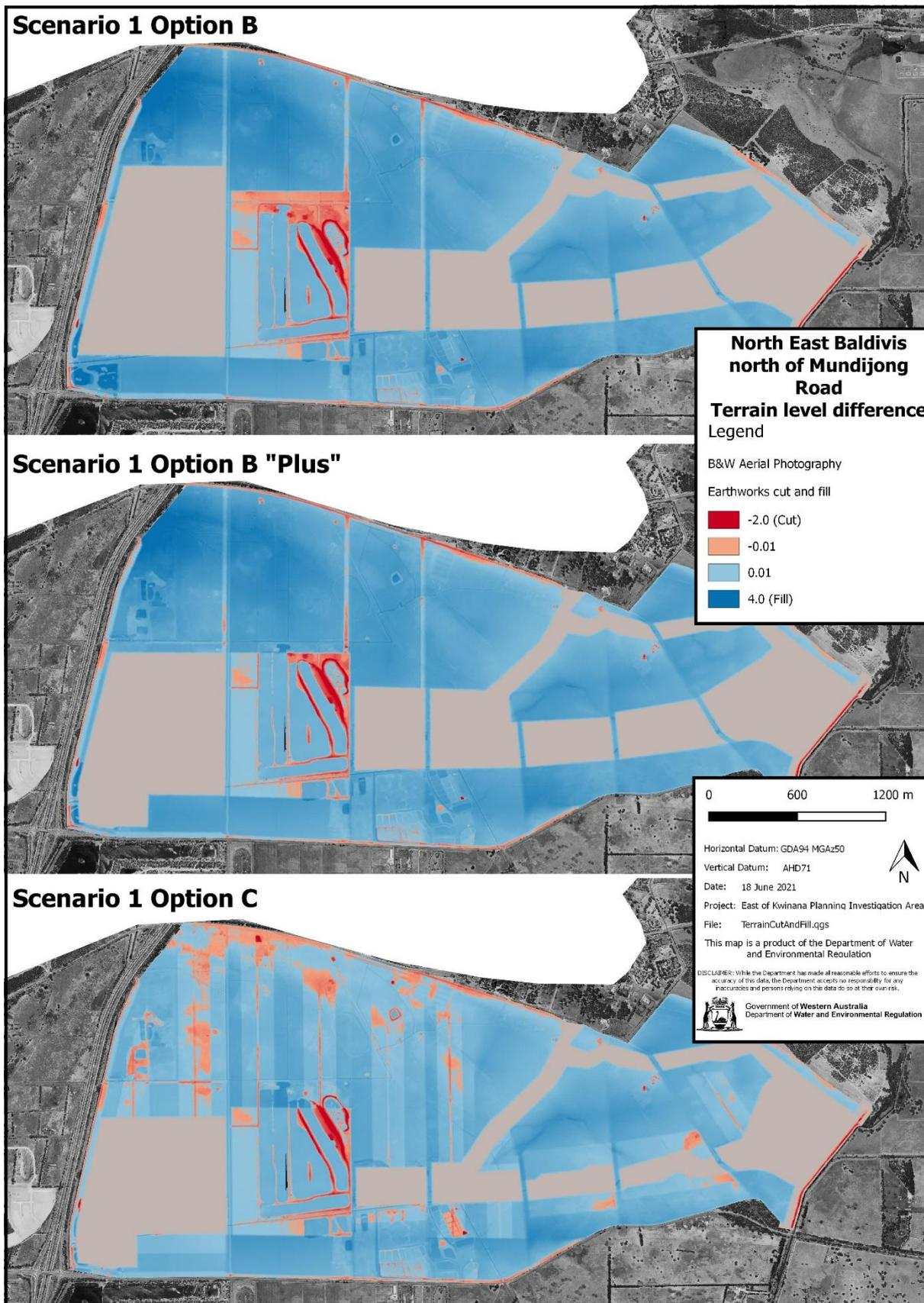
Figure 40 Scenario 1 Options B and C terrain level difference map
