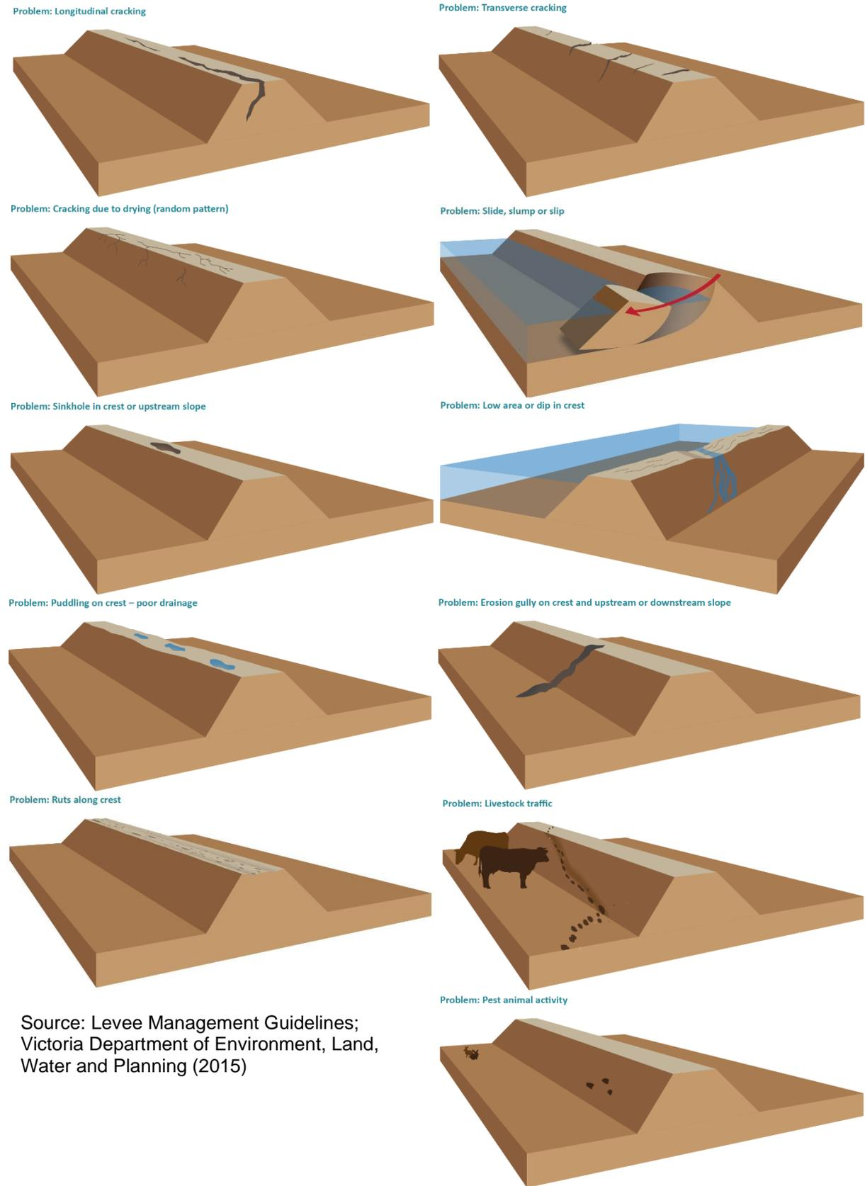
Figure 7 Additional common problems and failure mechanisms with levees
