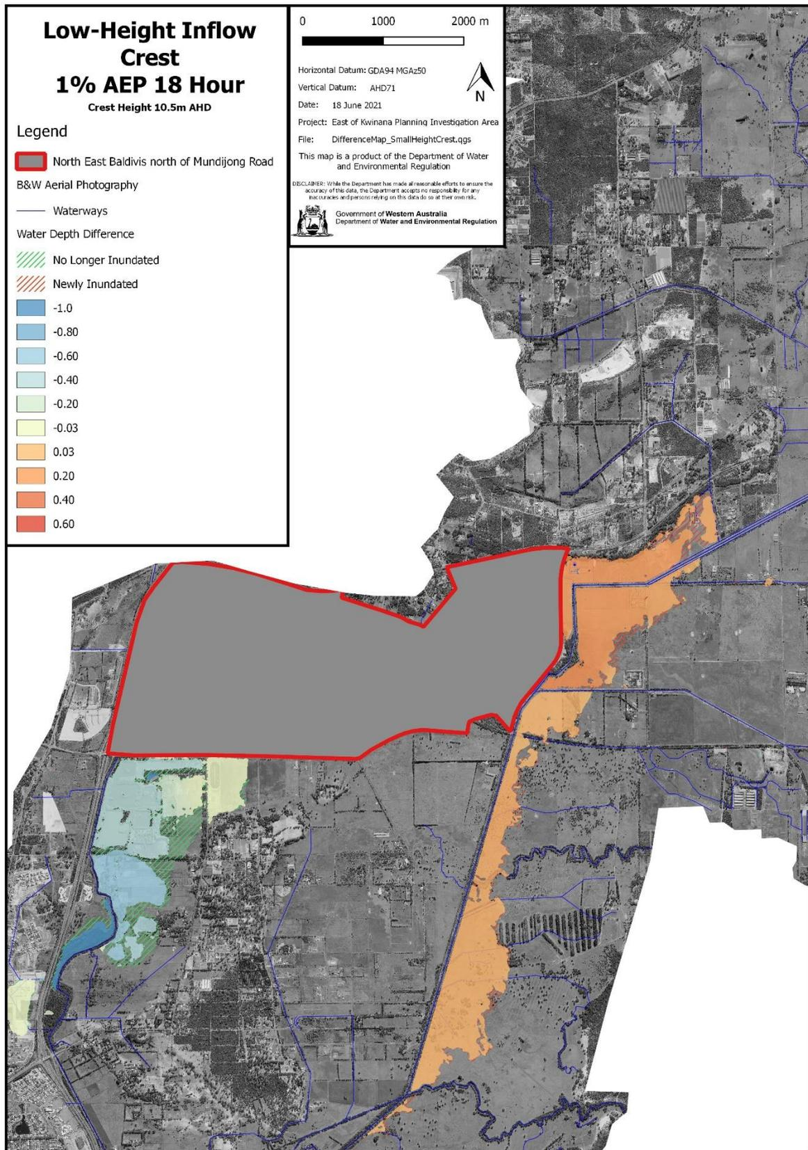
Figure 37 Pre-development 1% AEP flood low-height inflow crest at 10.5m AHD
