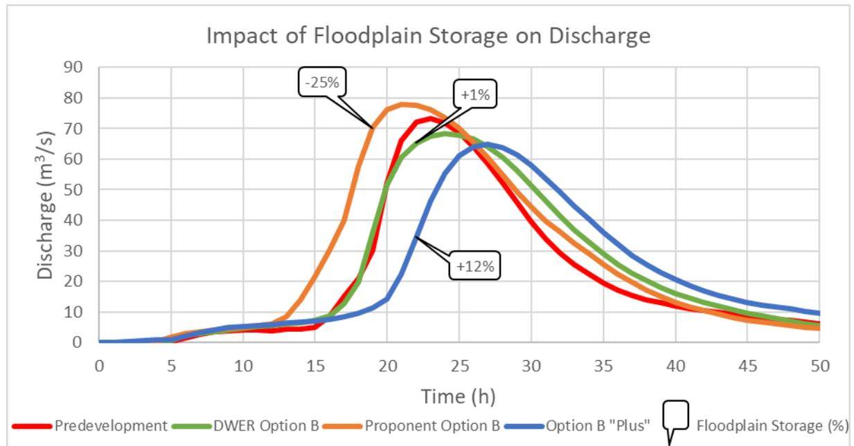
Figure 28 Impact of floodplain storage on discharge
