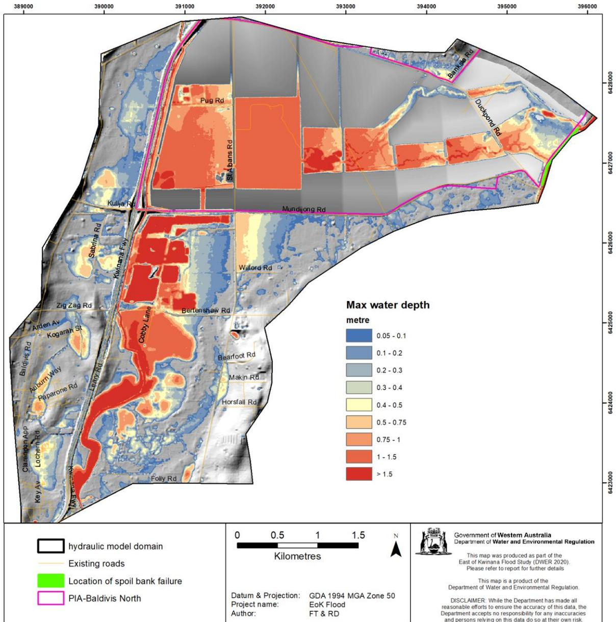
Figure 7-10 Maximum flooding water depth in Option B under 1% AEP 18-hour rainfall
