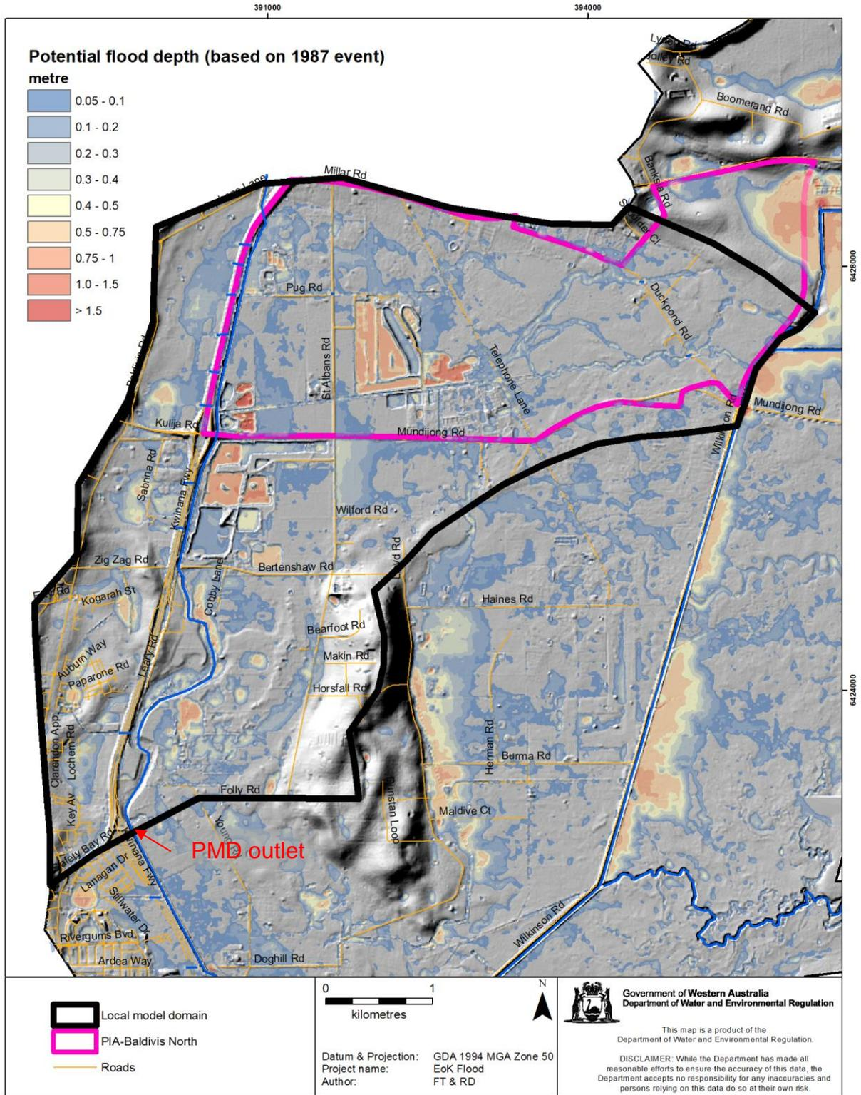
Figure 5-17 The local flood domain and the North East Baldivis north of Mundijong Road precinct and the 1987 modelling flood water level from the regional model
