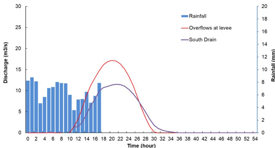
Figure 7-5 Hydrographs at the Levee and South Drain in Option A+
