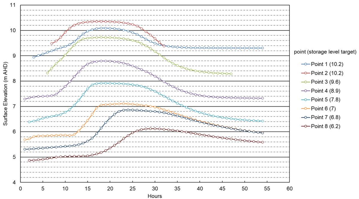
Figure 7-12 Hourly records of floodwater surface elevation in Option B at different sampling locations (point location are given in Figure 7-9)
