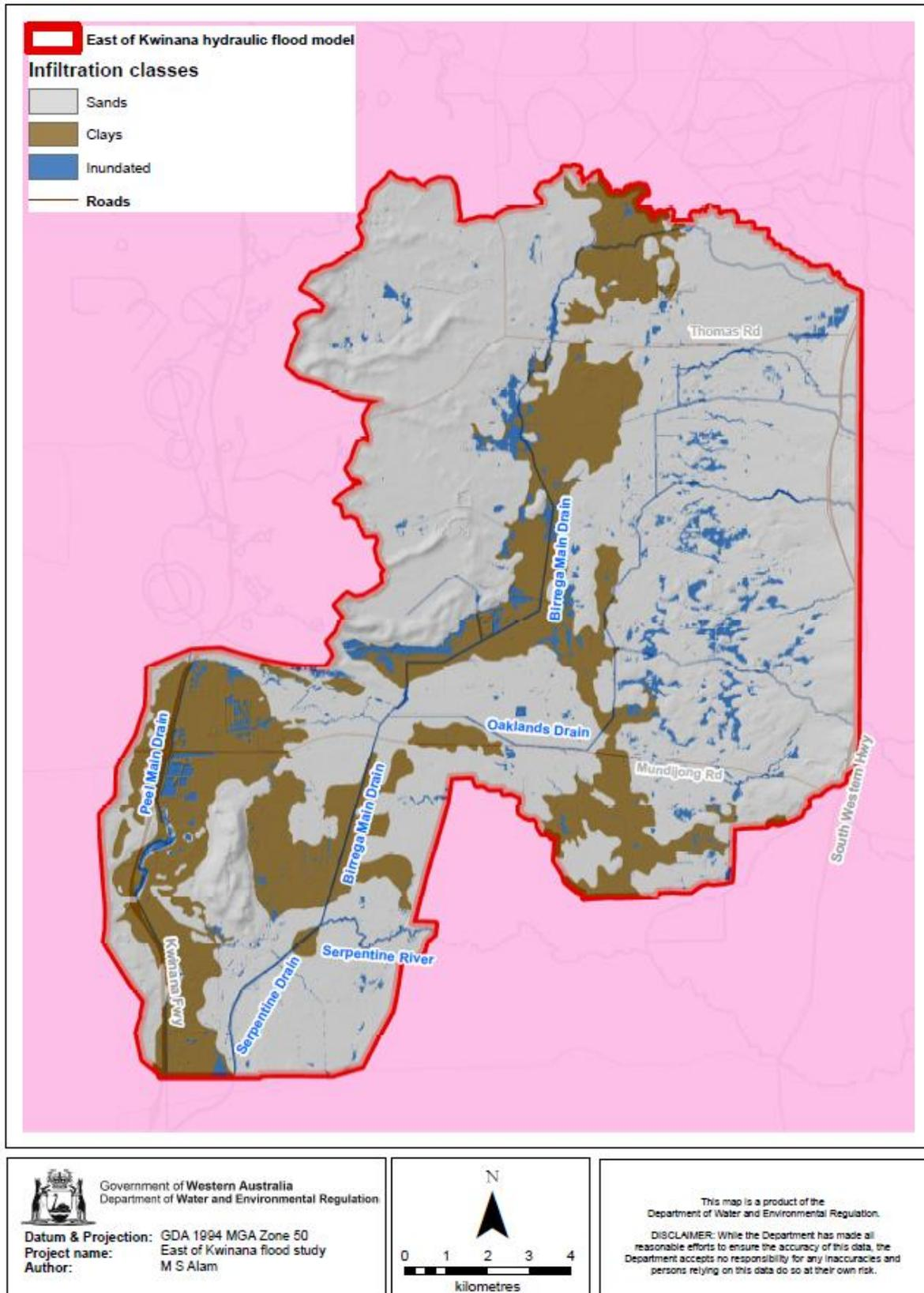
Figure 5-7 Infiltration map considered for the calibration and design runs; an infiltration rate (mm/day) of 70 (grey), 5 (umber) and 0 (blue) was considered for sand, clay and groundwater inundation areas
