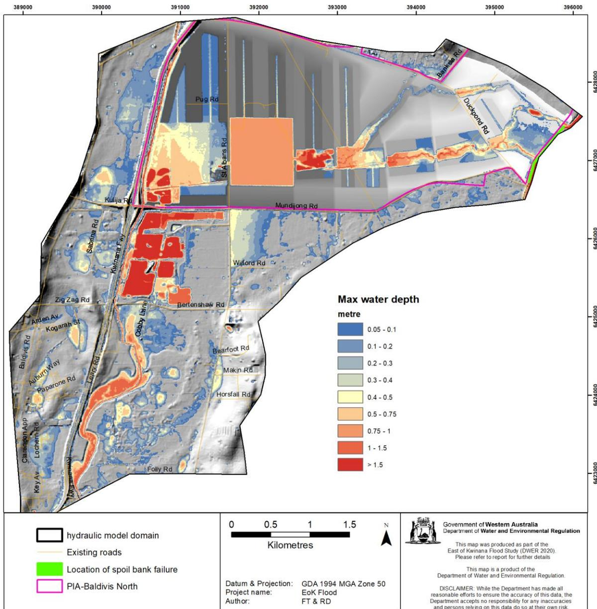
Figure 7-23 Maximum flooding water depth in Option C under 5% AEP 18-hour rainfall
