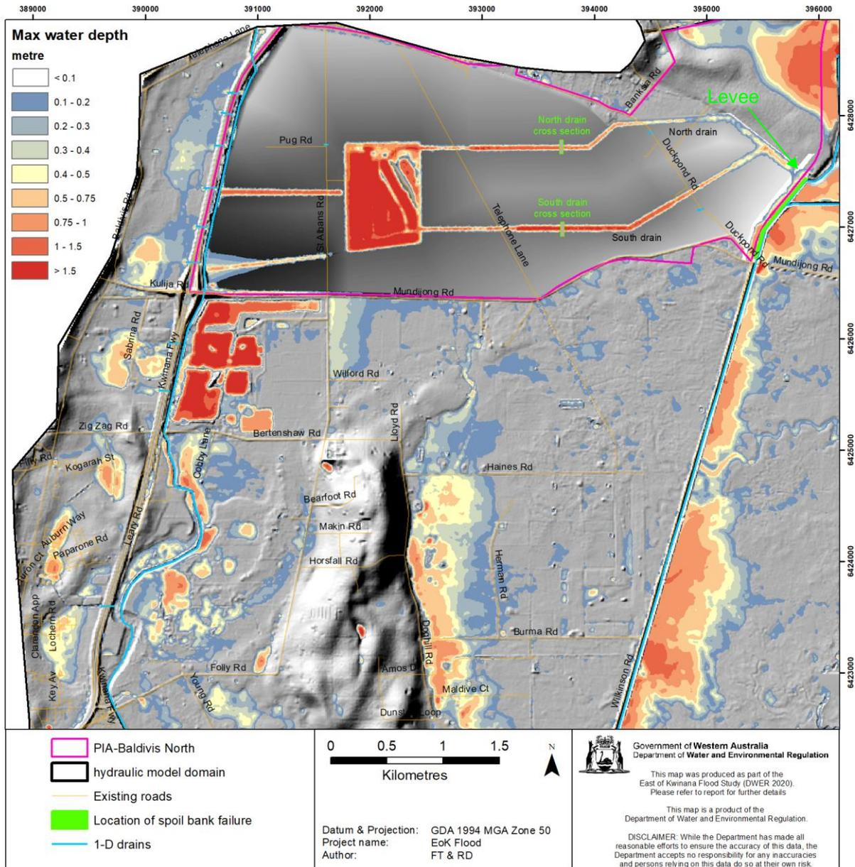
Figure 7-6 Maximum flooding water depth in Option A+ under 1% AEP 18-hour rainfall (based on the regional model). Option A+ is designed to allow a maximum of 17 m<sup>3</sup>/s discharge from the Birrega Main Drain under 1% AEP.
