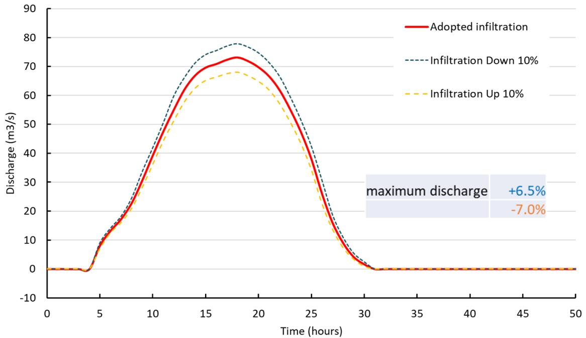
Figure 6-15 Sensitivity check on infiltration at 1% AEP 18-hour Tp1 by comparing the discharge at DP (refer to Figure 6-11 for the location)
