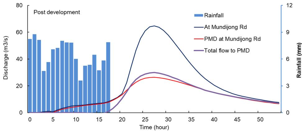
Figure 7-18 Selected discharge hydrographs in Option B+ under 1% AEP 18-hour duration rainfall
