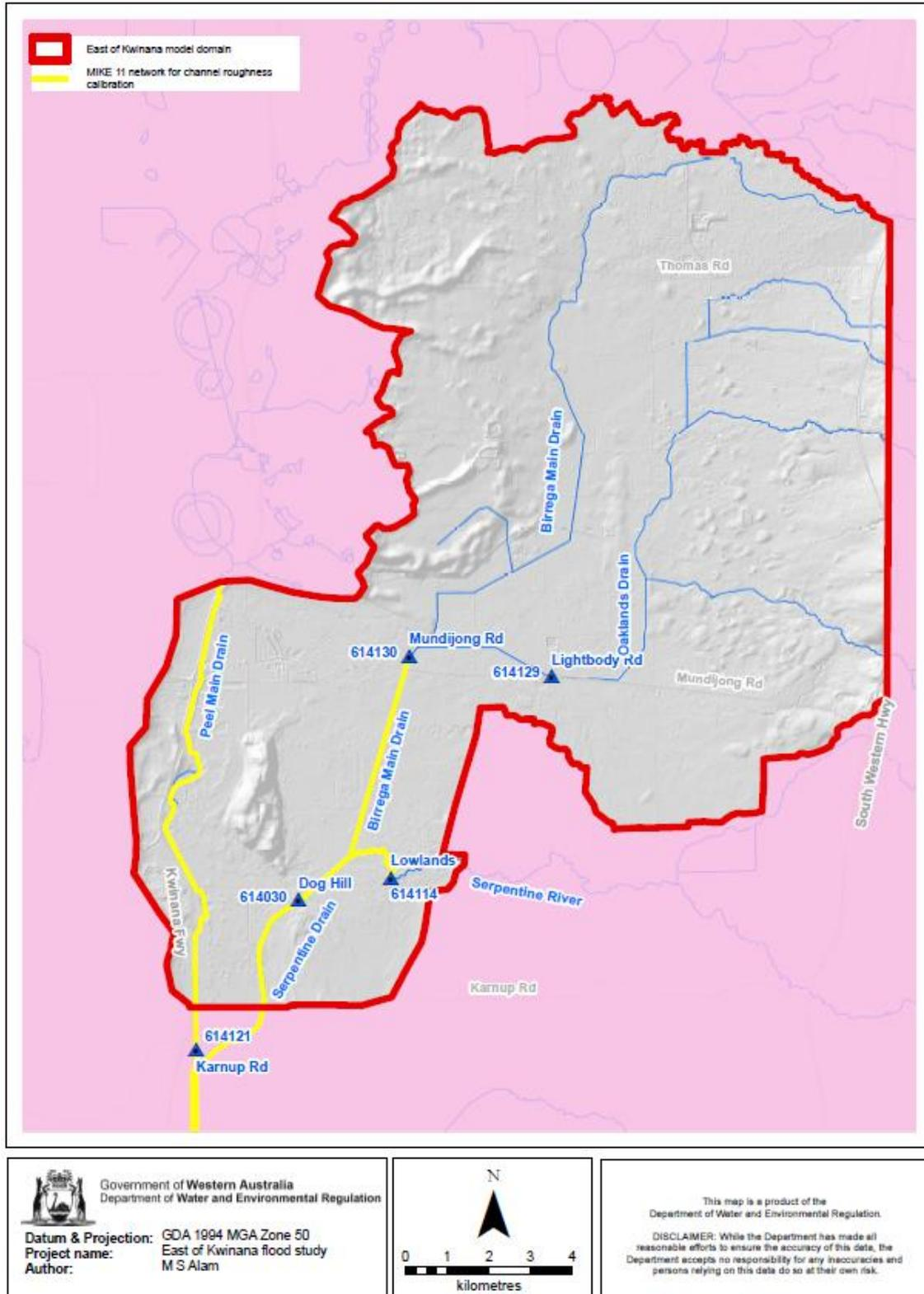
Figure 5-12 Channels considered for the calibration of channel roughness coefficient
