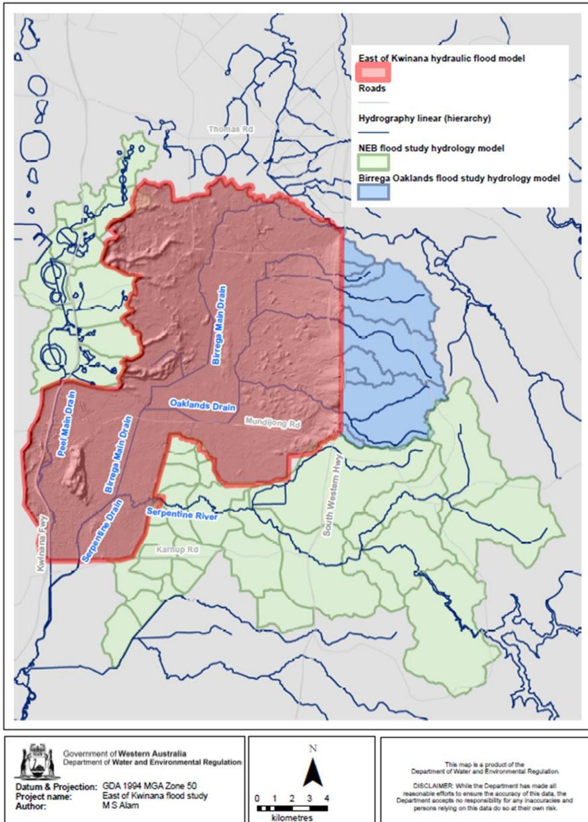
Figure 1-3 The East of Kwinana hydraulic model and the contributing upper North East Baldvis and Birrega and Oaklands hydrology catchment domains
