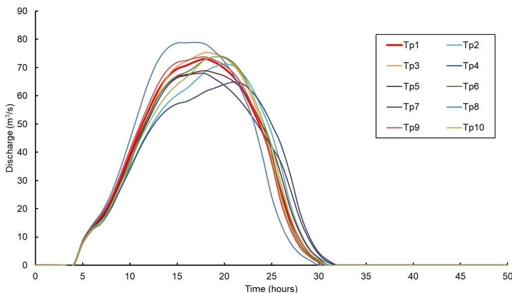
Figure 6-3 Sampled discharge at Duck Pond from the Birrega Main Drain under different rainfall temporal patterns, Tp1 to Tp10, for the 1% AEP 18-hour event
