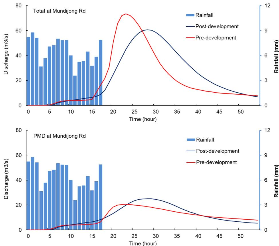
Figure 7-14 The impact of Option B to flow at Mundijong Road and Peel Main Drain
