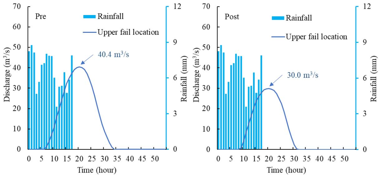
Figure 8-8 Comparison between discharges from the Pre- and Post-development conditions measured at the Upper fail location
