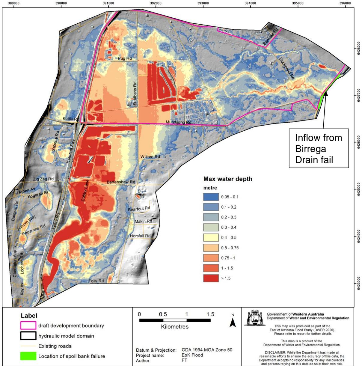
Figure 6-16 Maximum flood water depth from the Local model with spoil bank fail 100%
