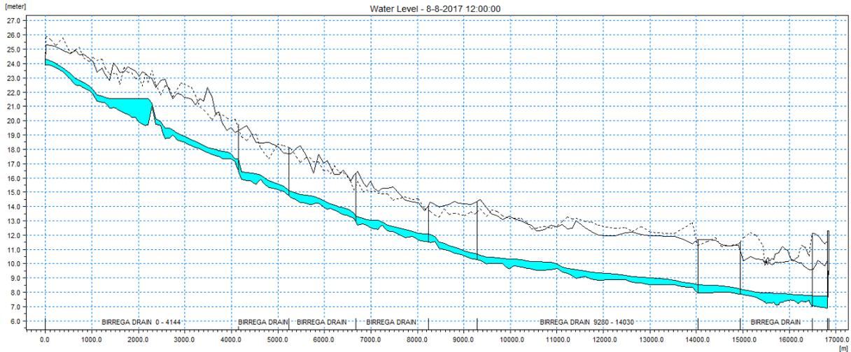
Figure 5-9 Initial water level for the Birrega Main Drain before its confluence with the Oaklands Main Drain
