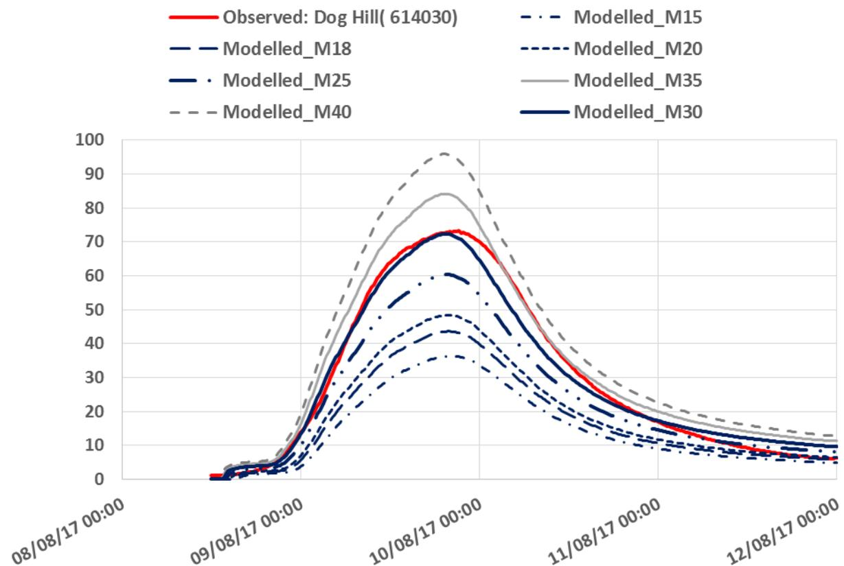
Figure 5-14 Calibration of channel roughness at Dog Hill site using Manning's M for the 2017 event (Source: MSA 2020)
