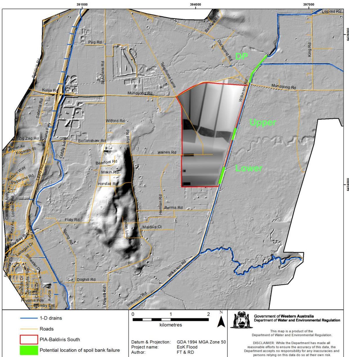
Figure 8-1 Hypothetical bathymetry of the options for the development scenario on North East Baldvis south of Mundijong Road precinct along with susceptible locations of spoil bank failure
