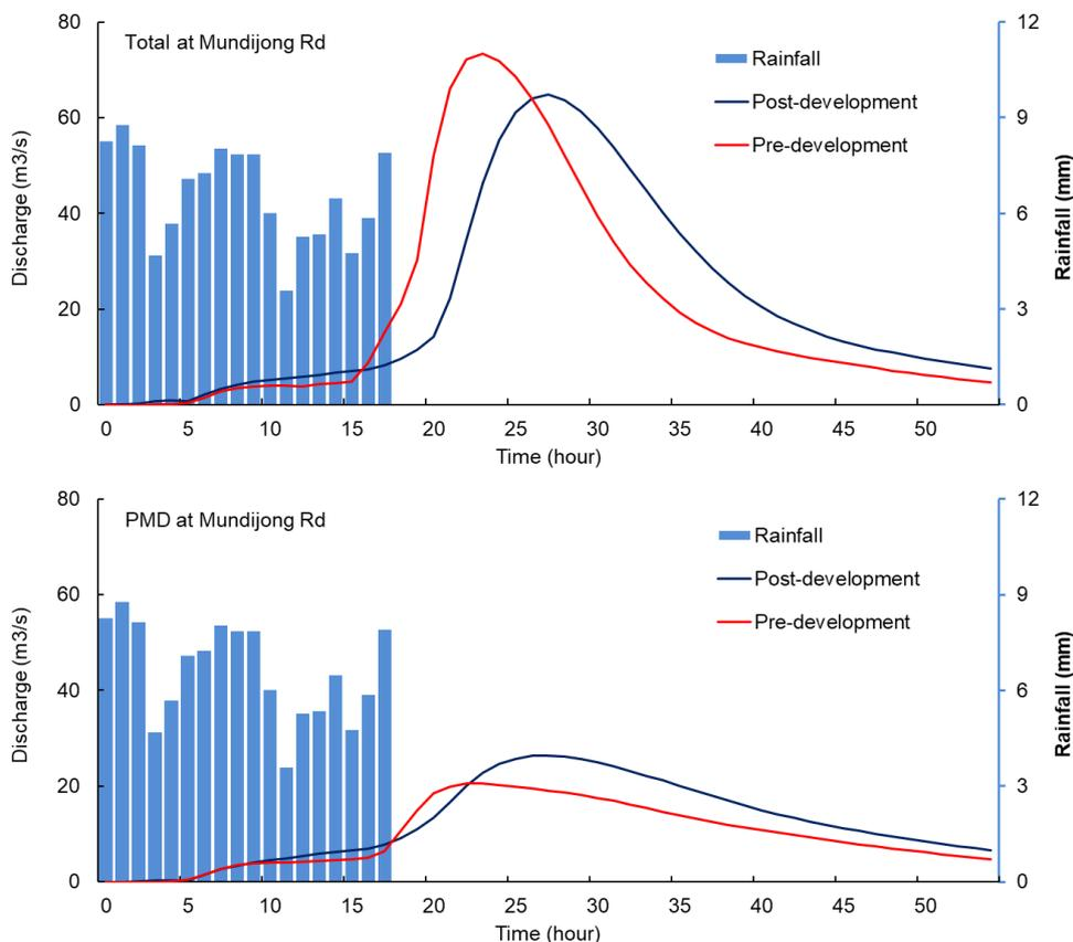
Figure 7-19 The impact of Option B+ to flow at Mundijong Road and Peel Main drain
