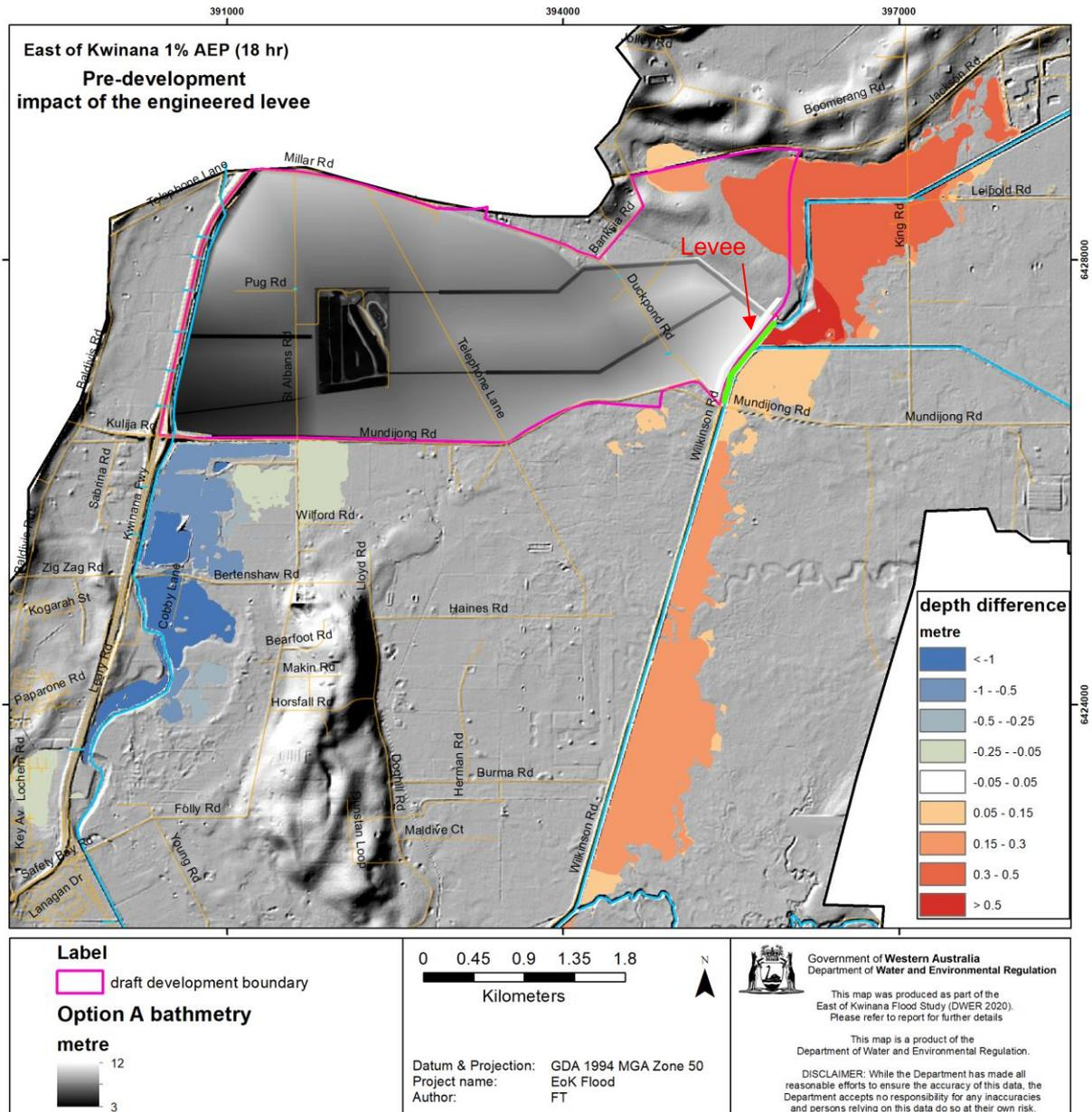
Figure 7-4 The engineered levee's impact at the Birrega Main Drain in Option A to the outsides (the upstream and downstream areas)
