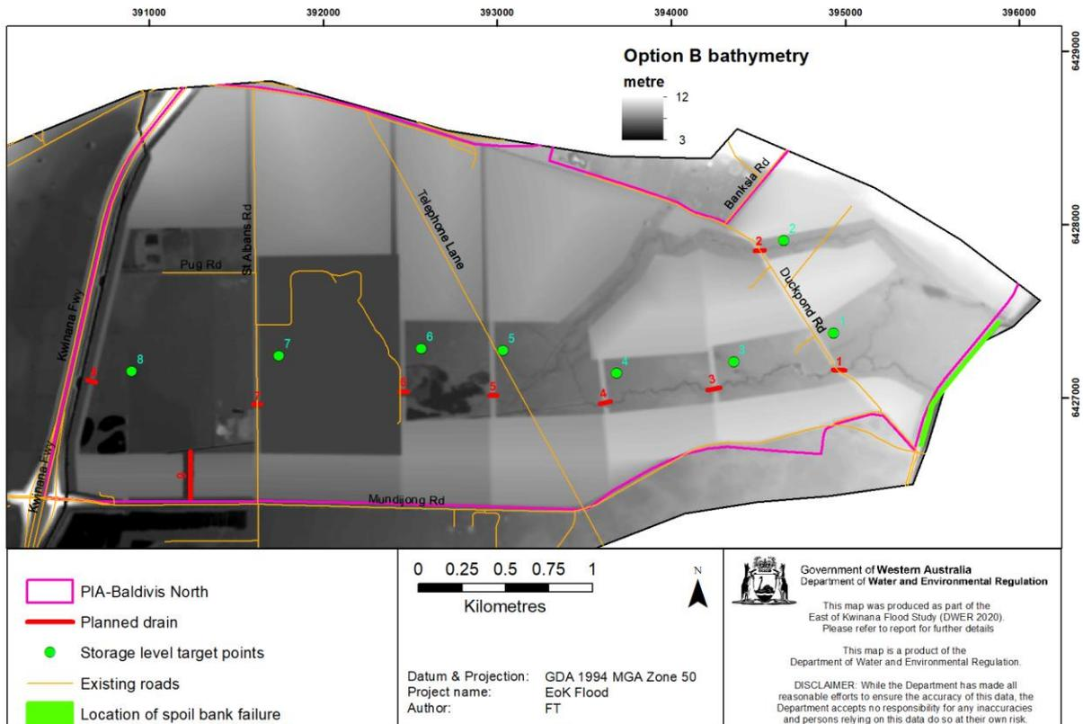
Figure 7-9 Hydraulics control channels (red) to divert floodwaters and flood level gauging points (green) to control storage levels
