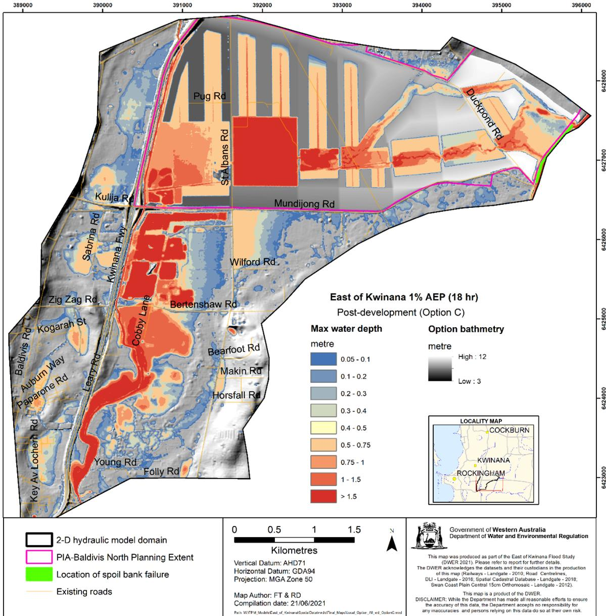
Figure 7-22 Maximum flooding water depth in Option C under 1% AEP 18-hour rainfall. Existing roads are also shown inside the North East Baldvis north of Mundijong Road precinct.
