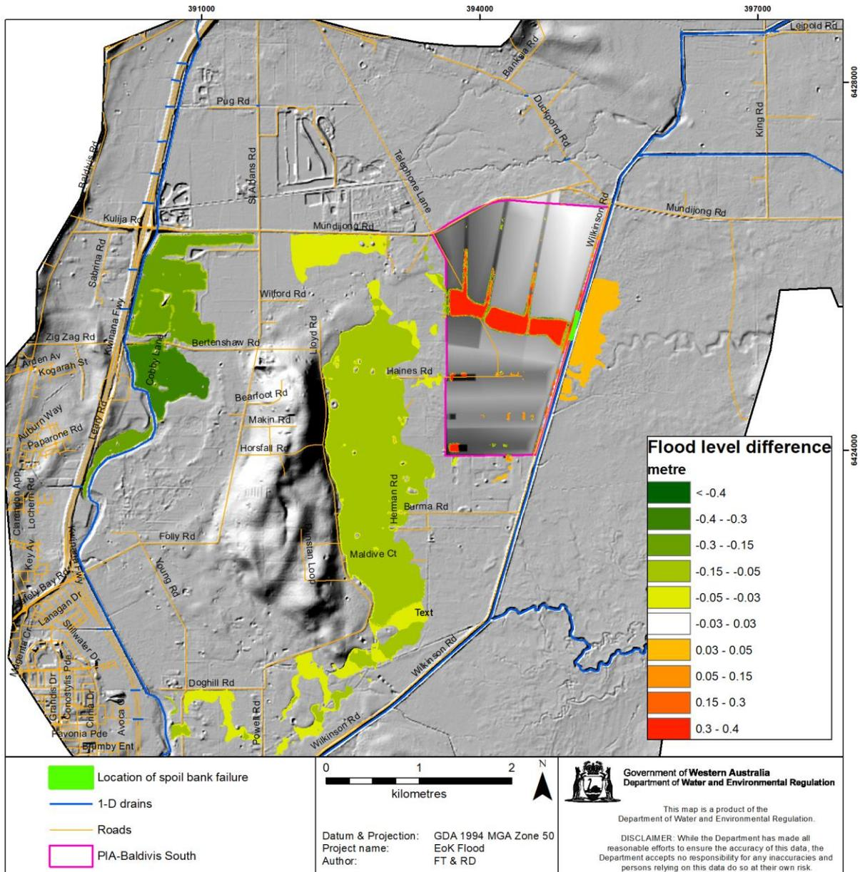
Figure 8-7 Flood level difference between the post- and pre-development conditions as given in Figure 8-6 and Figure 8-5
