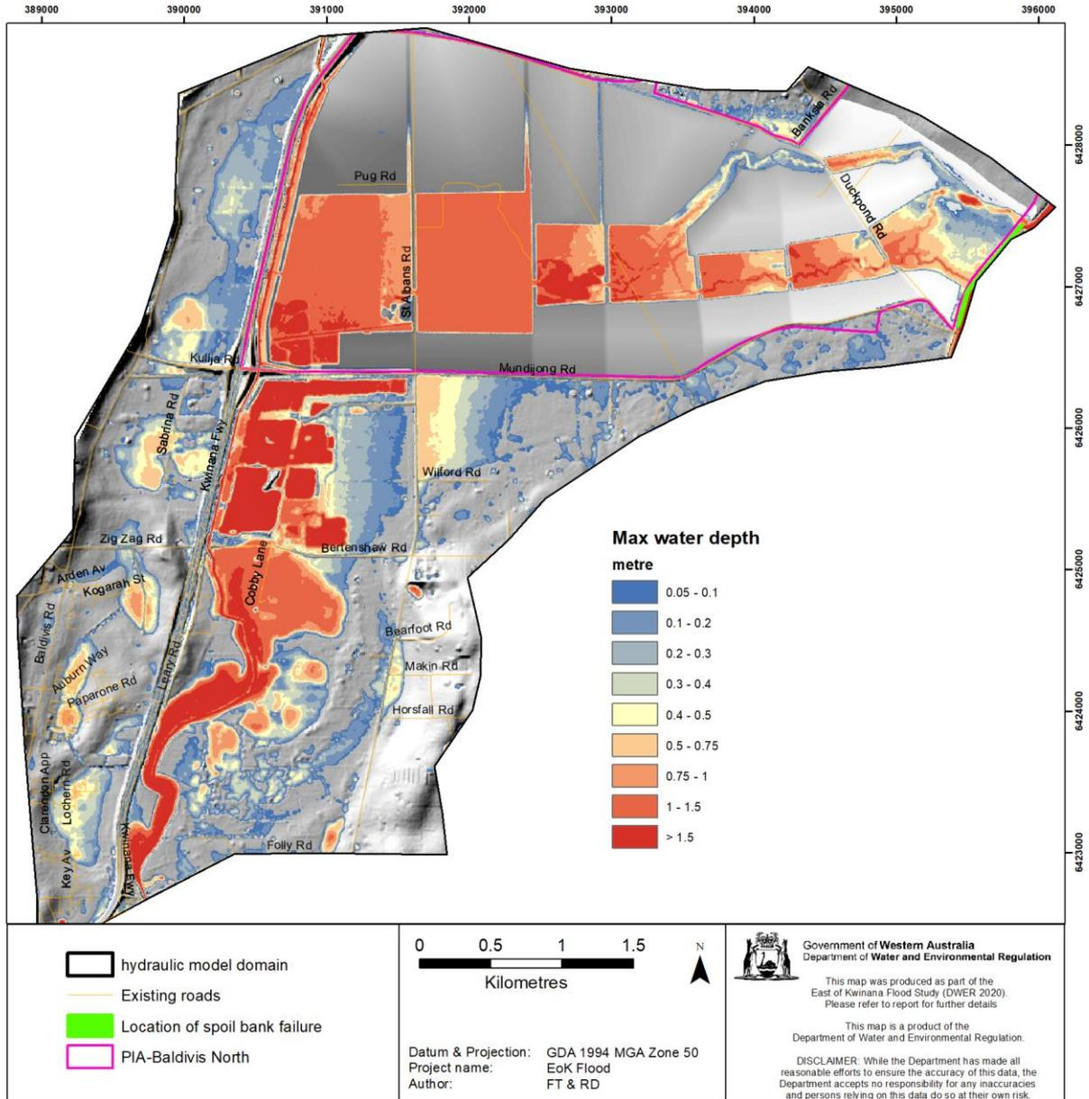
Figure 7-16 Maximum flooding water depth in Option B+ under 1% AEP 18-hour rainfall
