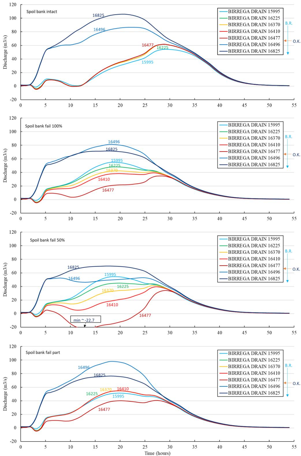
Figure 6-8 Comparison of hydrographs at eight cross-sections of Birrega Main Drain (B.R.) around its confluence with Oaklands Main Drain. Birrega chainage numbers are shown. Oaklands intersects with Birrega between chainages 16477 and 16496.
