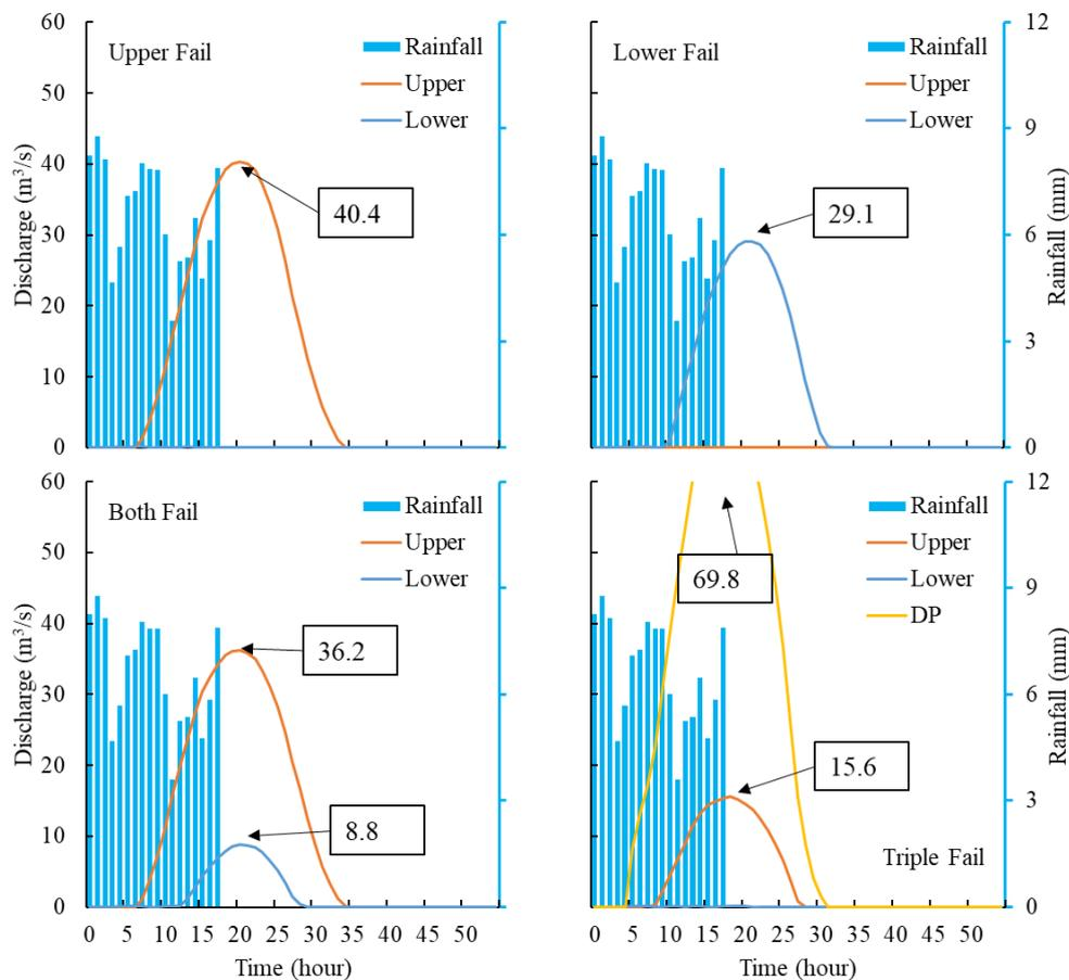
Figure 8-4 Discharges from the Birrega Main Drain measured immediately downstream the respective potential spoil bank failure locations (refer to Table 8-1 for all cases)
