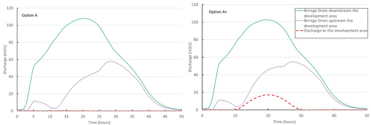
**Figure 7-8** The engineered levee's impact on Birrega Main Drain by allowing a maximum of 17 m<sup>3</sup>/s discharge into Option A terrain
