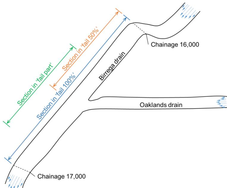
Figure 6-5 A schematic diagram on the Birrega Main Drain spoil bank failure scenarios
