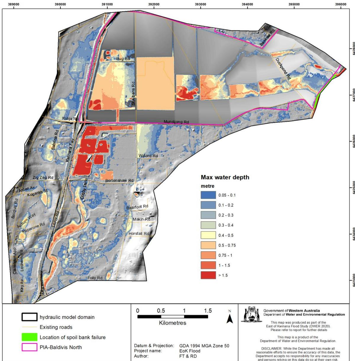
Figure 7-11 Maximum flooding water depth in Option B under 5% AEP 18-hour rainfall
