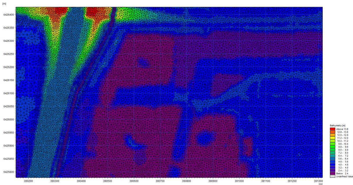
Figure 5-16 Example of mesh showing fine resolution at the corner of Mundijong Road and Kwinana Freeway in the local model
