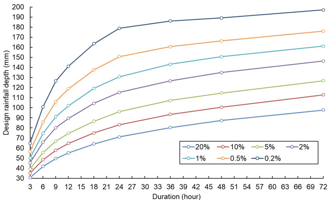
Figure 4-2 Design rainfall depths (mm) for the regional model at different AEP events.
