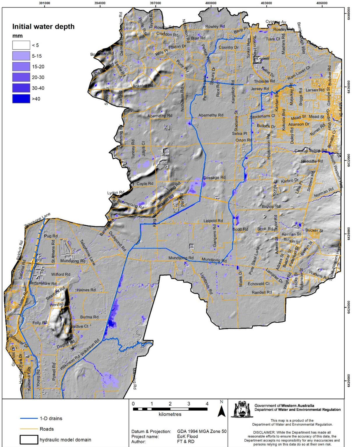
Figure 5-6 Overland water depth for all design and validation runs
