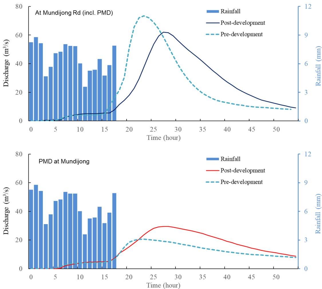
Figure 7-24 The impact of Option C to flow at Mundijong Road and Peel Main drain under 1% AEP 18-hour rainfall
