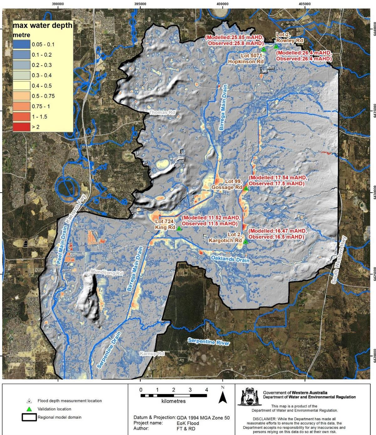
Figure 5-15 Observed versus modelled water levels for the 1987 flood event, along with the flood mapping from the simulation
