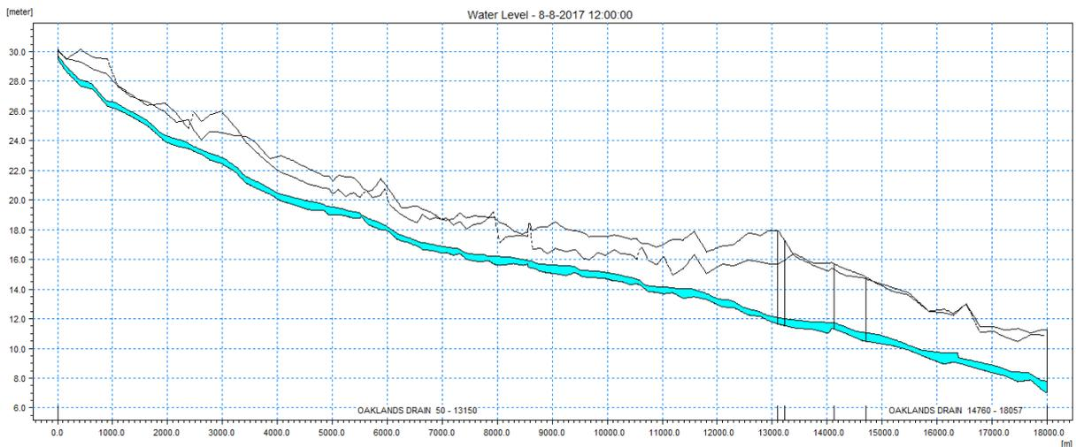
Figure 5-10 Initial water level for the Oaklands Main Drain before its confluence with the Birrega Main Drain
