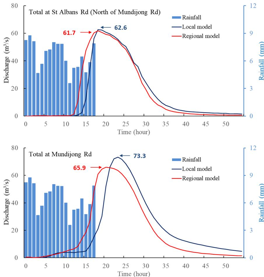
Figure 6-18 Comparison of the total discharges over St Albans Road (top) and Mundijong Road (bottom)
