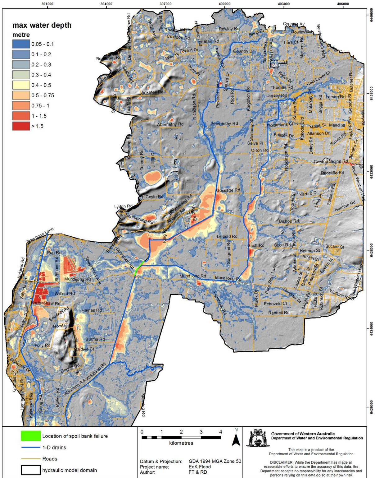
Figure F-13 Maximum flooding water depth with the build levee to 10.5 m AHD scenario (at 1% AEP 18-hour Tp1 rainfall)
