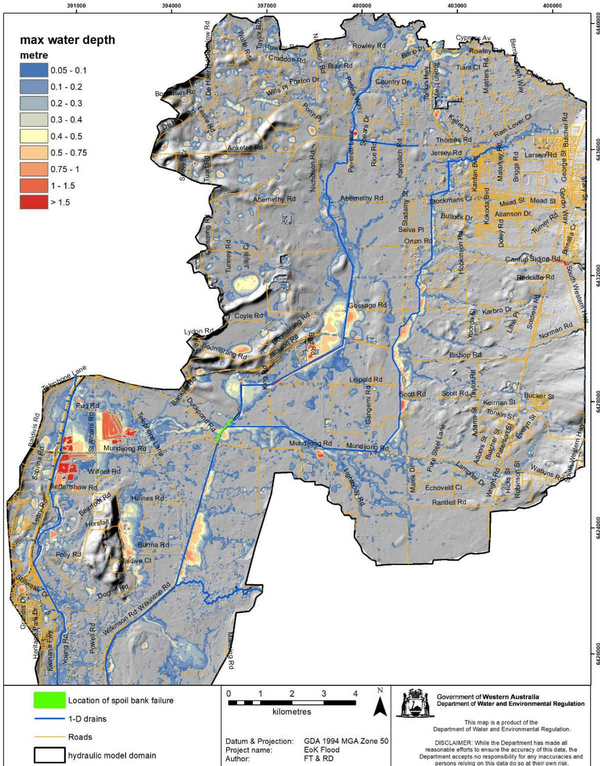
Figure D-10 Max. water depth at 5% AEP from 12-, 18-, 24- and 36-hour rainfalls with evenly distributed temporal patterns
