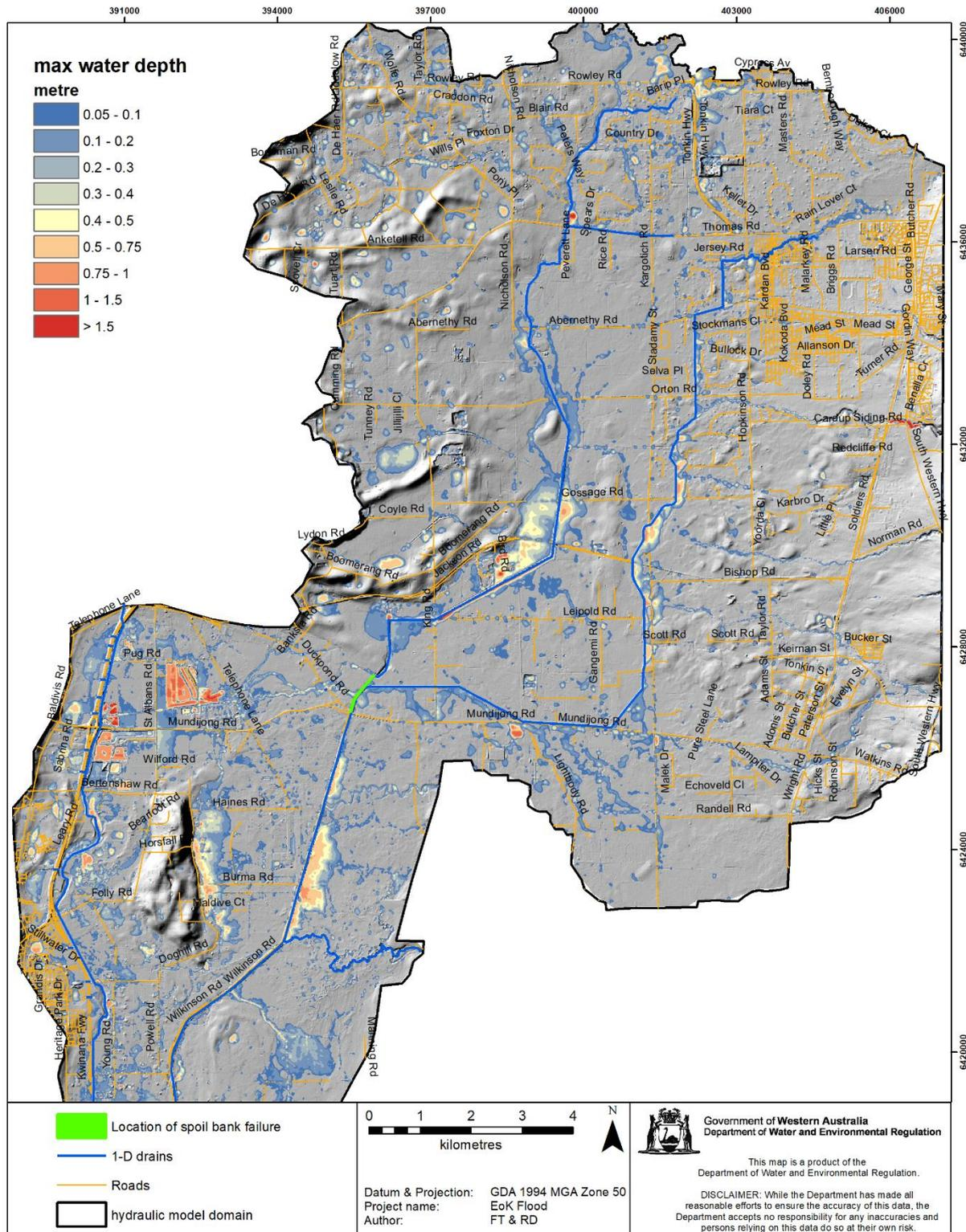
Figure E-11 Max. water depth at 10% AEP from 12-, 18-, 24- and 36-hour rainfalls with evenly distributed temporal patterns
