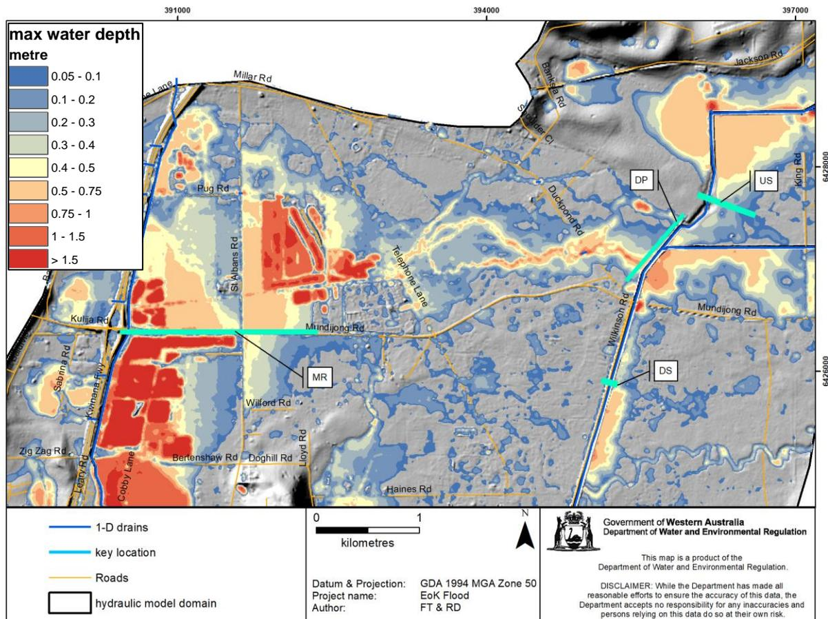
Figure 6-11 Location of the cross-sections for flow statistics (max water depth is from Figure 6-9)
