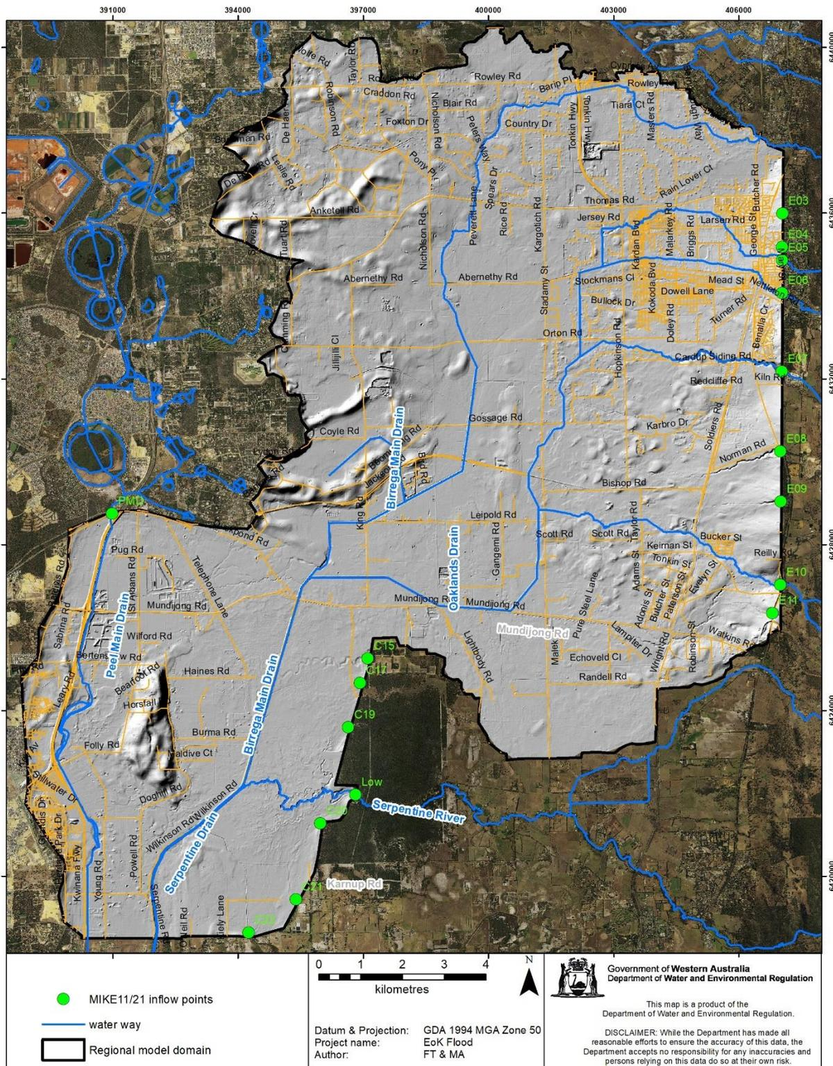
Figure 4-4 Position of design inflows in the regional model (PMD – Peel Main Drain and low-lowlands are MIKE11 inflows, while the rest are MIKE21)
