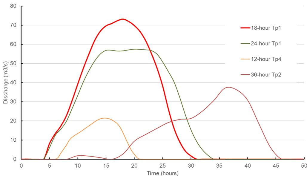
Figure 6-2 Sampled discharges from Birrega Main Drain into North East Baldivis north of Mundijong Road precinct under different rainfall temporal patterns, Tp1 to Tp10, for the 1% AEP 18-hour event
