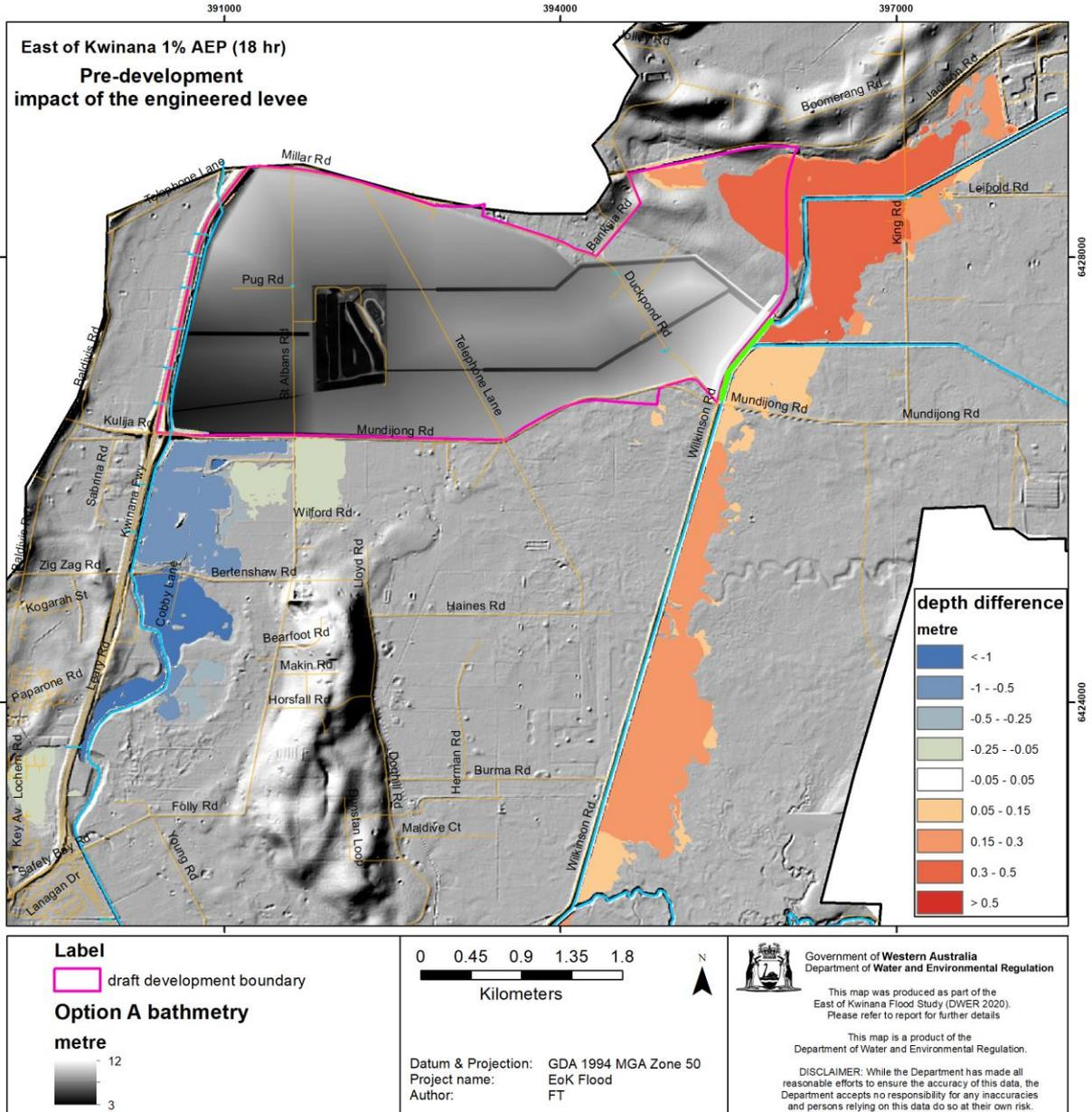
Figure 7-7 The engineered levee's impact on the floodplain by allowing a maximum of 17 m<sup>3</sup>/s discharge into Option A terrain
