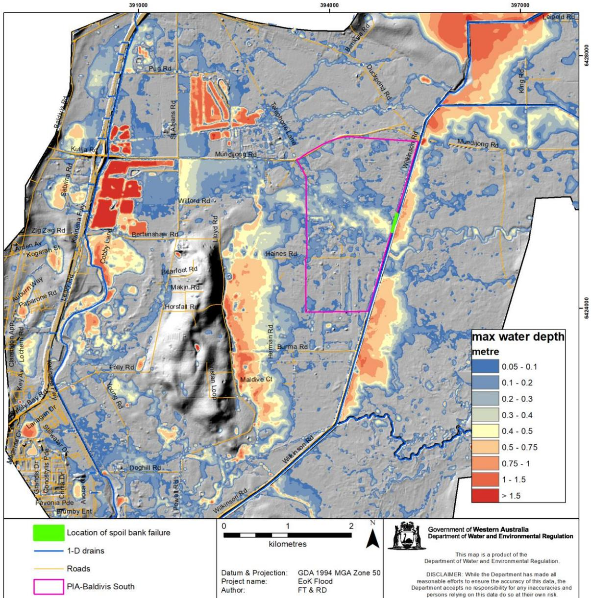
Figure 8-5 Maximum pre-development flooding water depth focusing on North East Baldvis south of Mundijong Road precinct under 1% AEP 18-hour Tp1 rainfall
