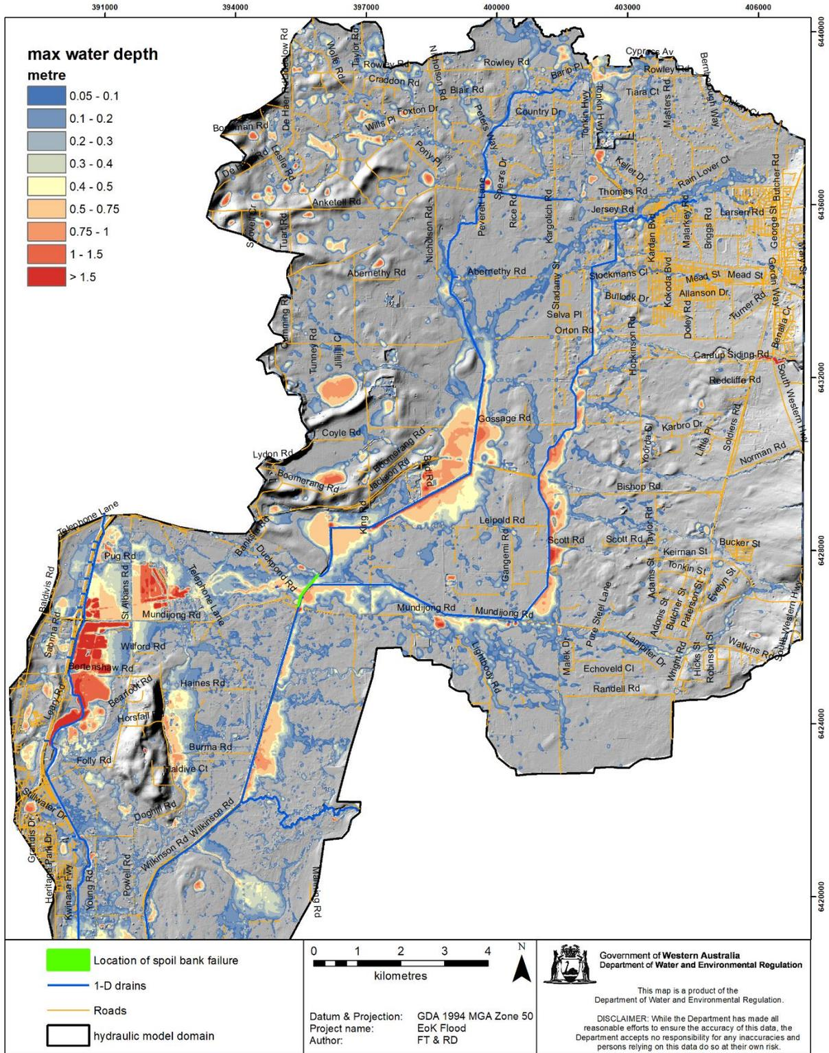
Figure 6-9 Max water depth at the 1% AEP 18-hour Tp1 inputs for the pre-development case (spoil bank fail 100%)
