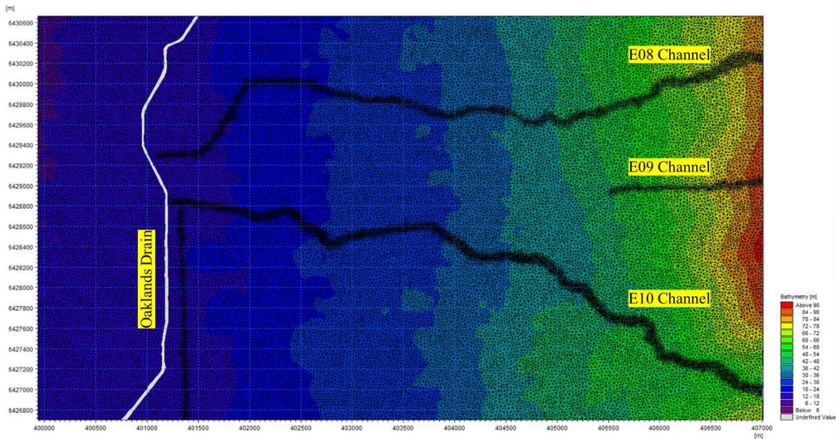
Figure 5-2 Example of mesh showing different mesh resolution/geometry. Here, the pre-development mesh is overlaid on pre-development DEM levels.
