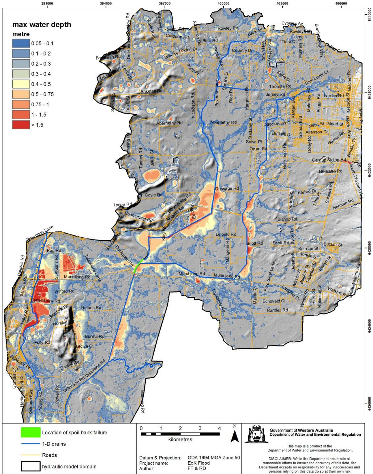
Figure F-12 Maximum flooding water depth with spoil bank fail part scenario (at 1% AEP 18-hour  $Tp1$  rainfall)
