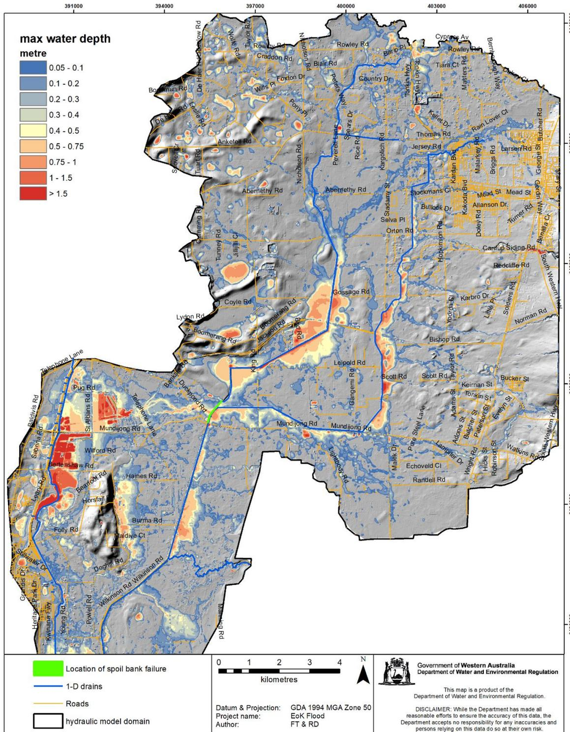
Figure 6-1 Flood mapping from 1% AEP runs (12, 18, 24 and 36-hour durations) at the spoil bank fail 100% scenario, as discussed in section 6.2.3. Each of the rainfalls was deemed to be evenly distributed.
