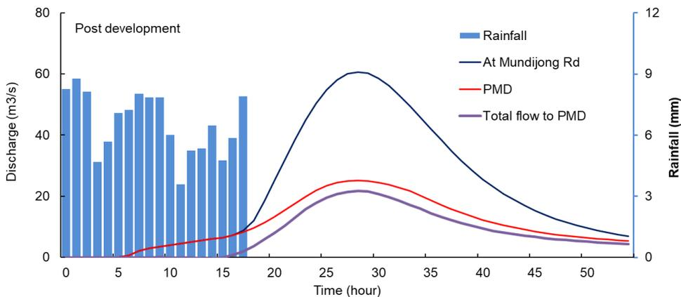
Figure 7-13 Selected discharge hydrographs in Option B under 1% AEP 18-hour duration rainfall
