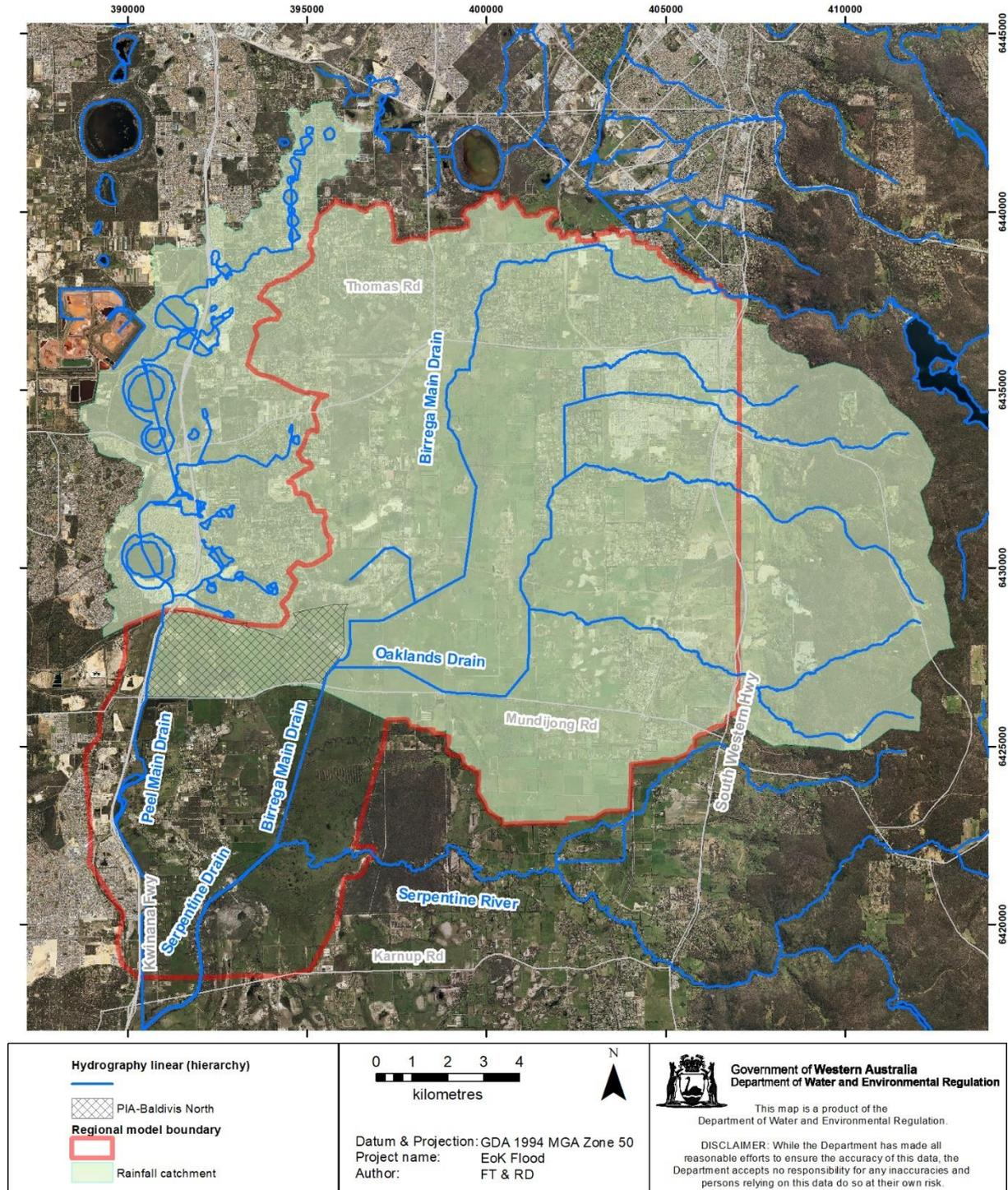
Figure 4-1 The catchment used to generate the design rainfalls North East Baldivis north of Mundijong Road (grid), the hydraulic model and the key linear hydrography linear
