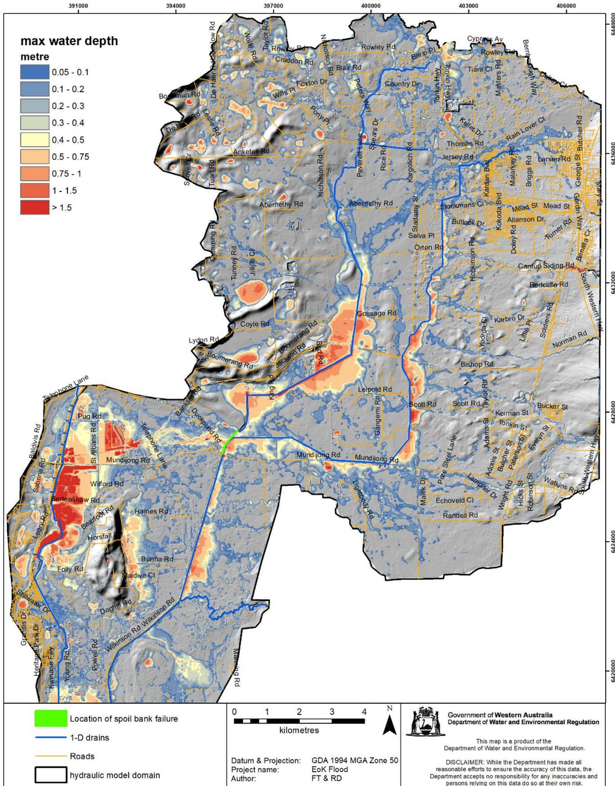
Figure B-6 Max. water depth at 0.5% AEP from 12-, 18-, 24- and 36-hr rainfalls with evenly distributed temporal patterns, which was generated by calculating the maximum floodwater depth at each grid
