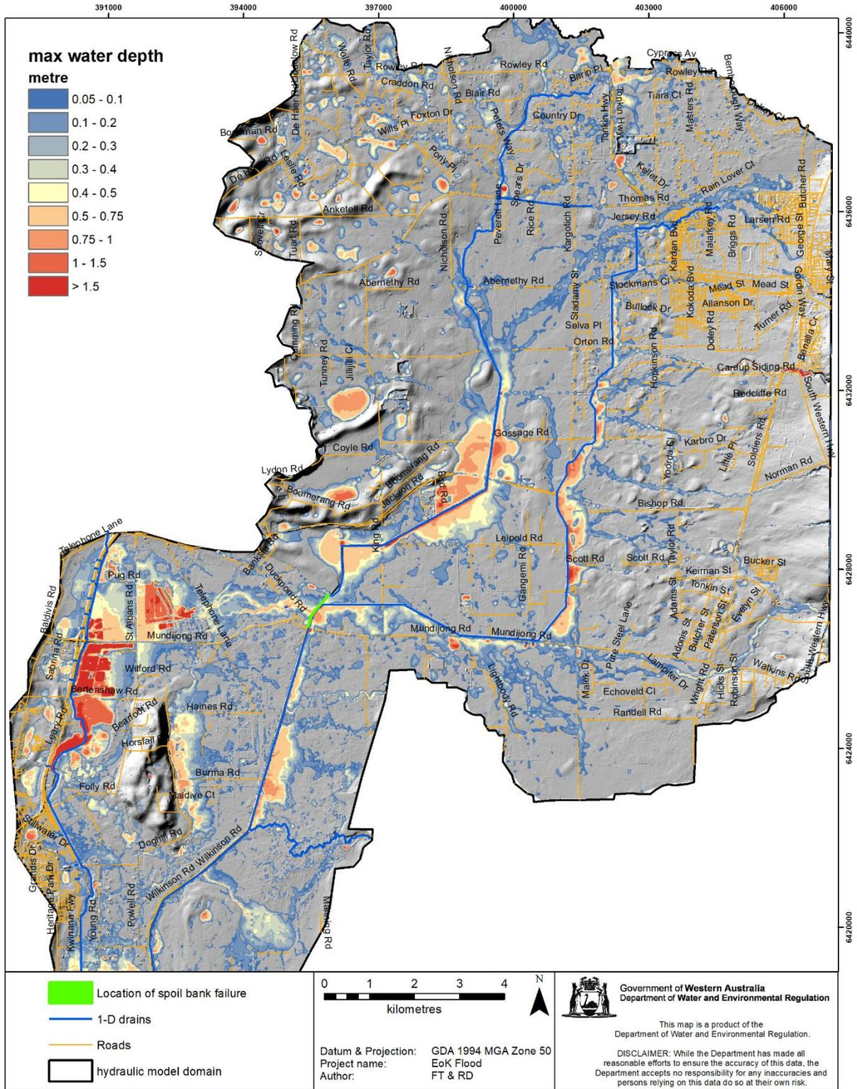
Figure C-8 Maximum flooding water depth at 1% AEP 18-hour  $Tp4$  back-loaded rainfall (with spoil bank fail 100%)
