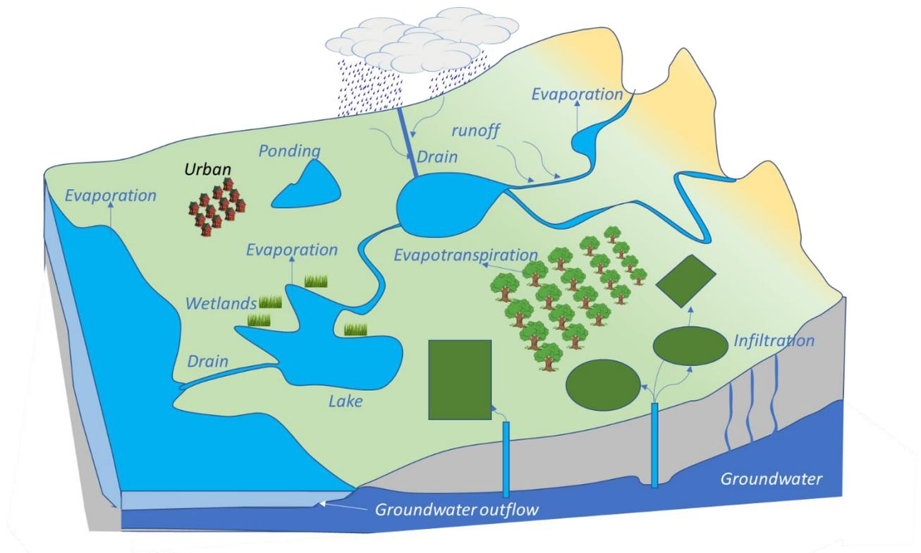
Figure 2-1 The East of Kwinana flood model conceptualisation (Cloud, Town, Forest, Grass based on various sources)
