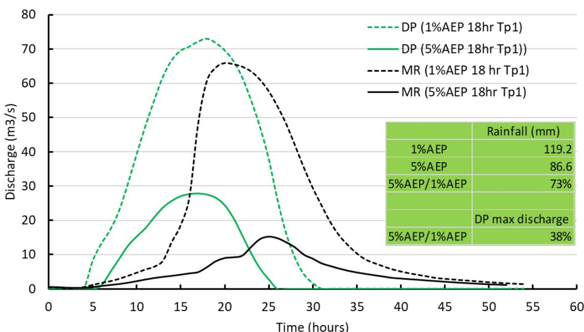
Figure 6-12 Comparison between the discharges from 1% AEP and 5% AEP rainfalls at two locations
