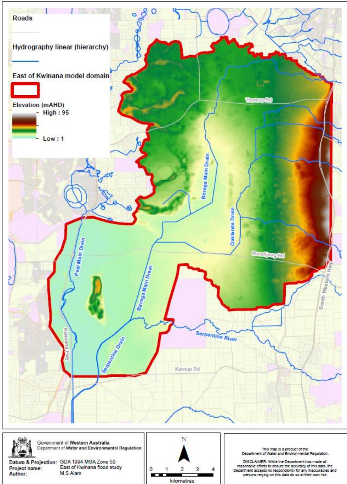
Figure 3-4 Model topography map developed from the department's 1 m LiDAR dataset
