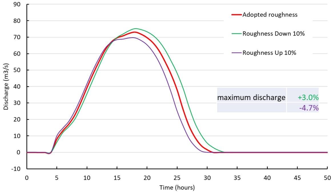
Figure 6-14 Sensitivity check on hydraulic roughness at 1% AEP 18-hour Tp1 by comparing the discharge at DP (refer to Figure 6-11 for the location)
