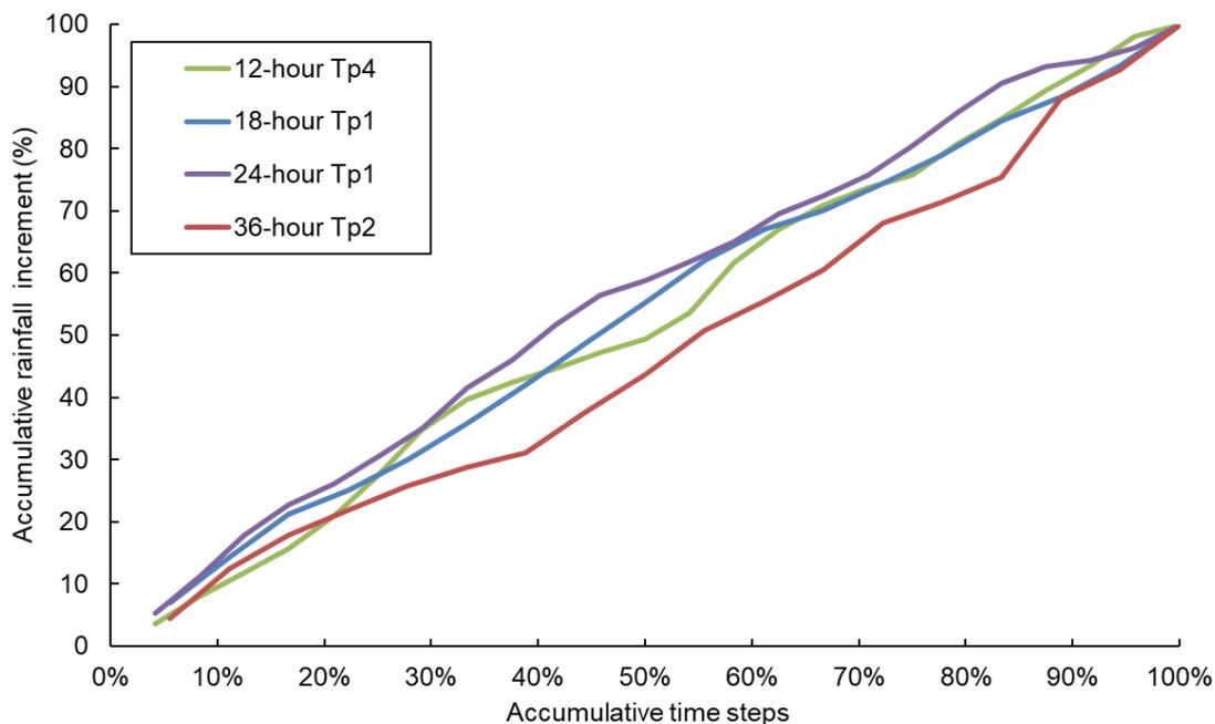
Figure 6-4 Temporal patterns deemed to be the median ones at 12-, 18-, 24- and 36-hour rainfall durations
