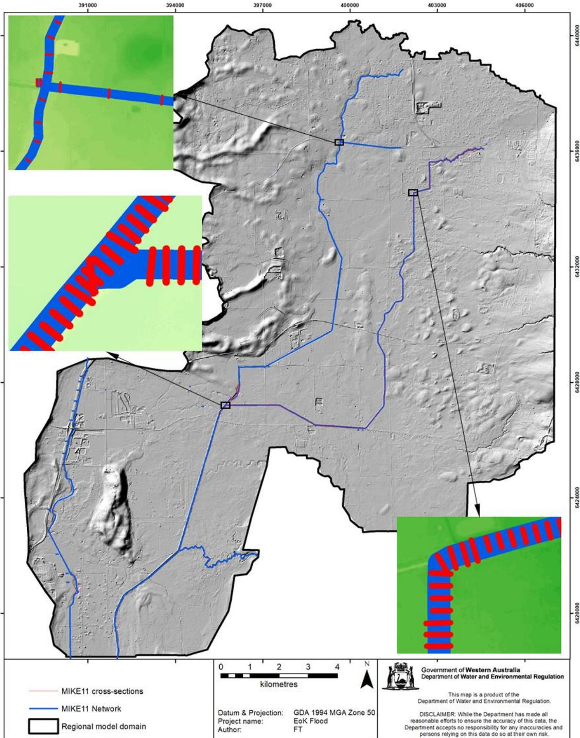
Figure 5-8 MIKE 11 Network and Cross-sections– insets show the cross-sections at three locations
