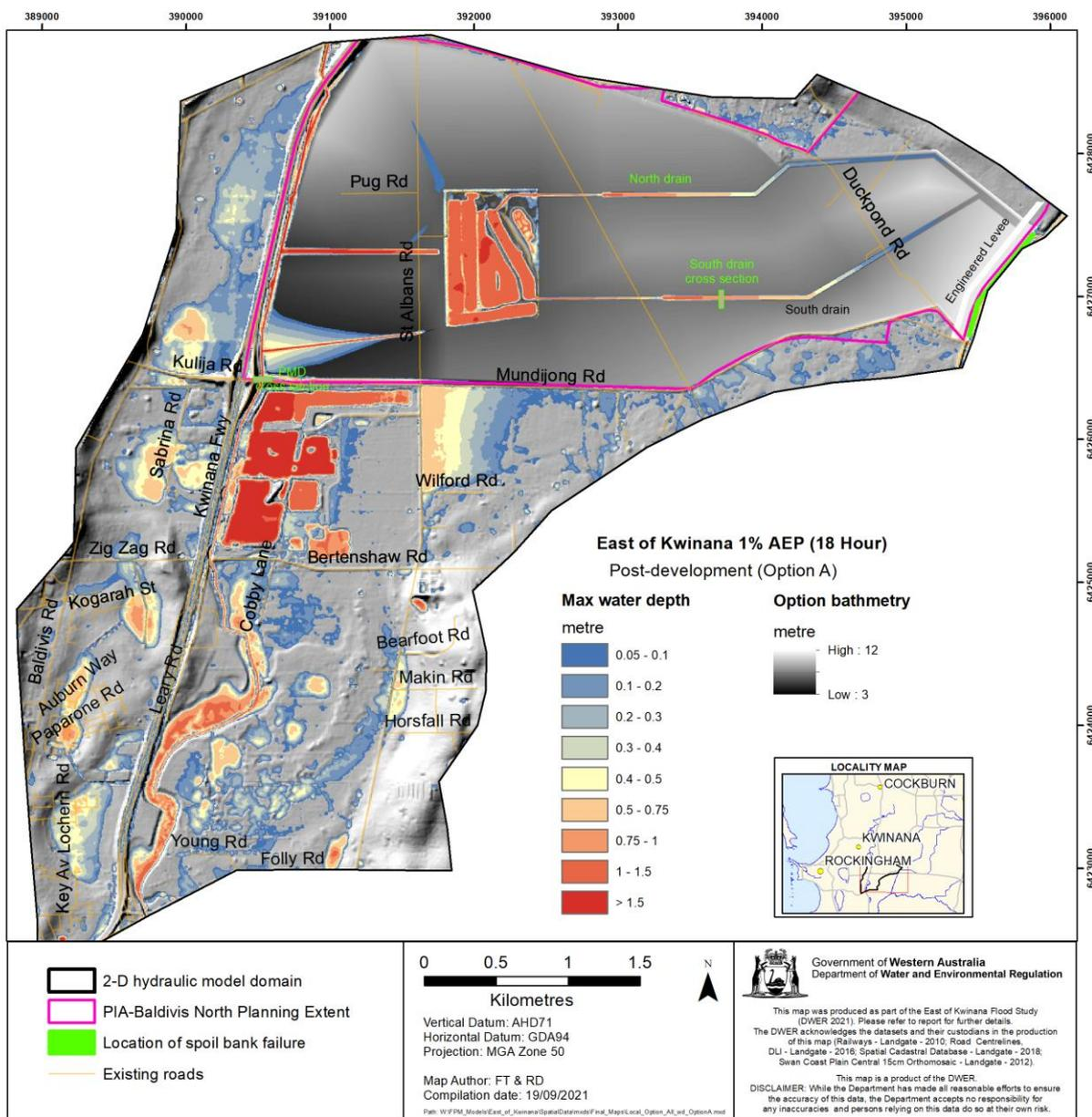
Figure 7-2 Flood mapping for Option A from the 1% AEP 18-hour Tp1 design rainfall
