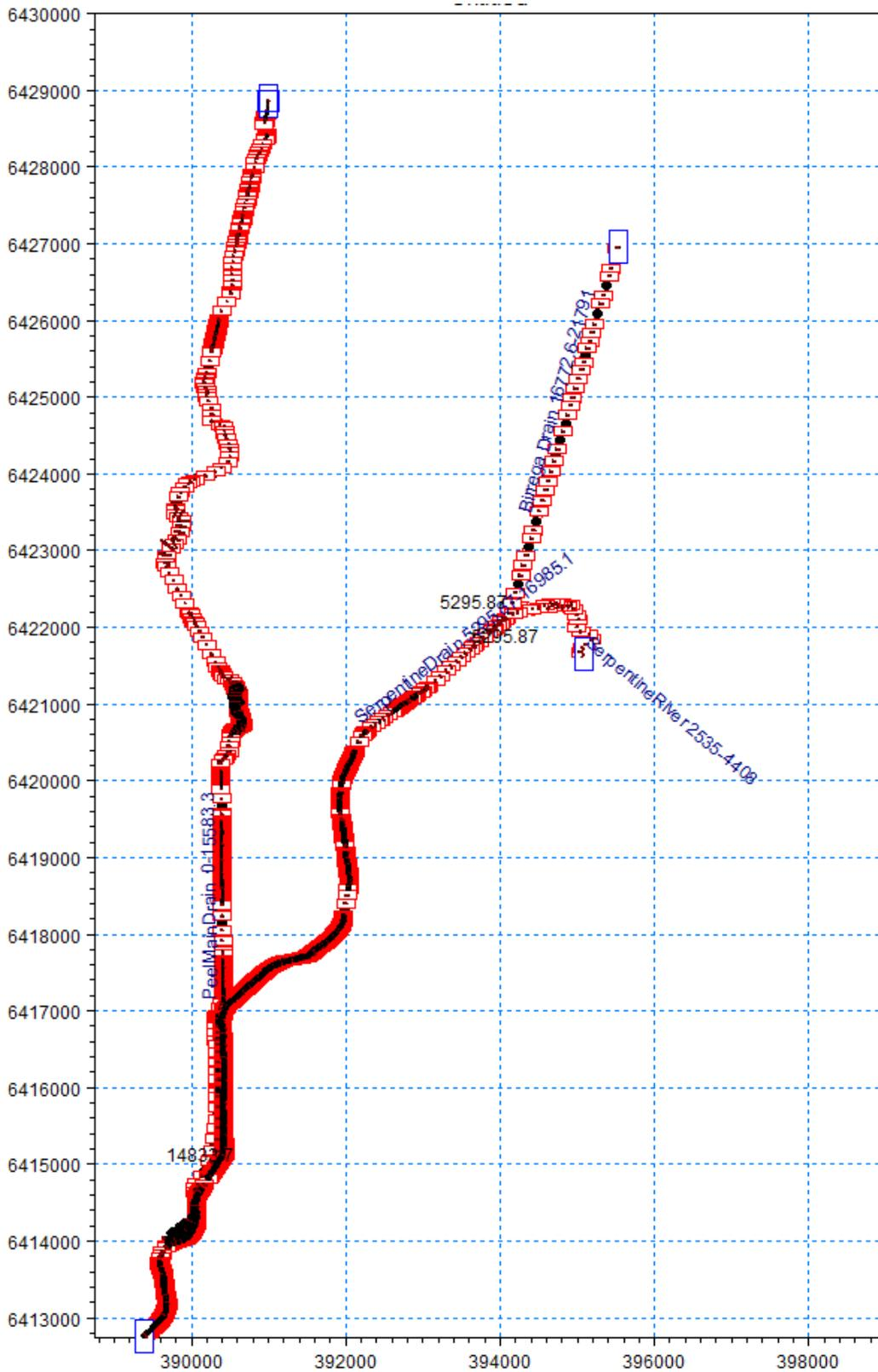
Figure 5-13 Flow network as seen from MIKE11 considered for the channel roughness coefficient's calibration (Source: MSA 2020)
