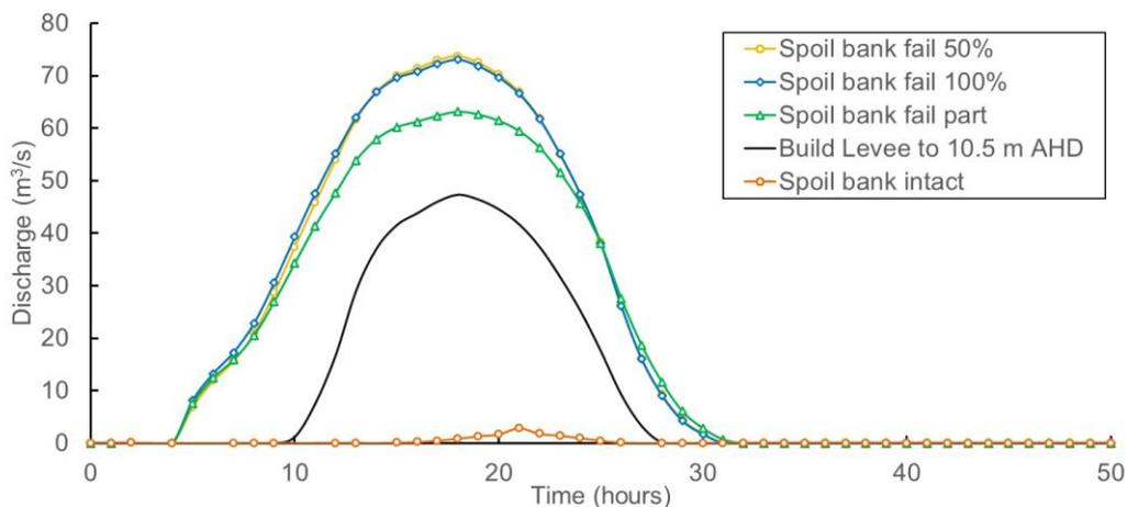
Figure 6-7 Sampled discharges from Birrega Main Drain to the North East Baldivis north of Mundijong Road precinct from five spoil bank failure scenarios (1% AEP 18-hour Tp1)
