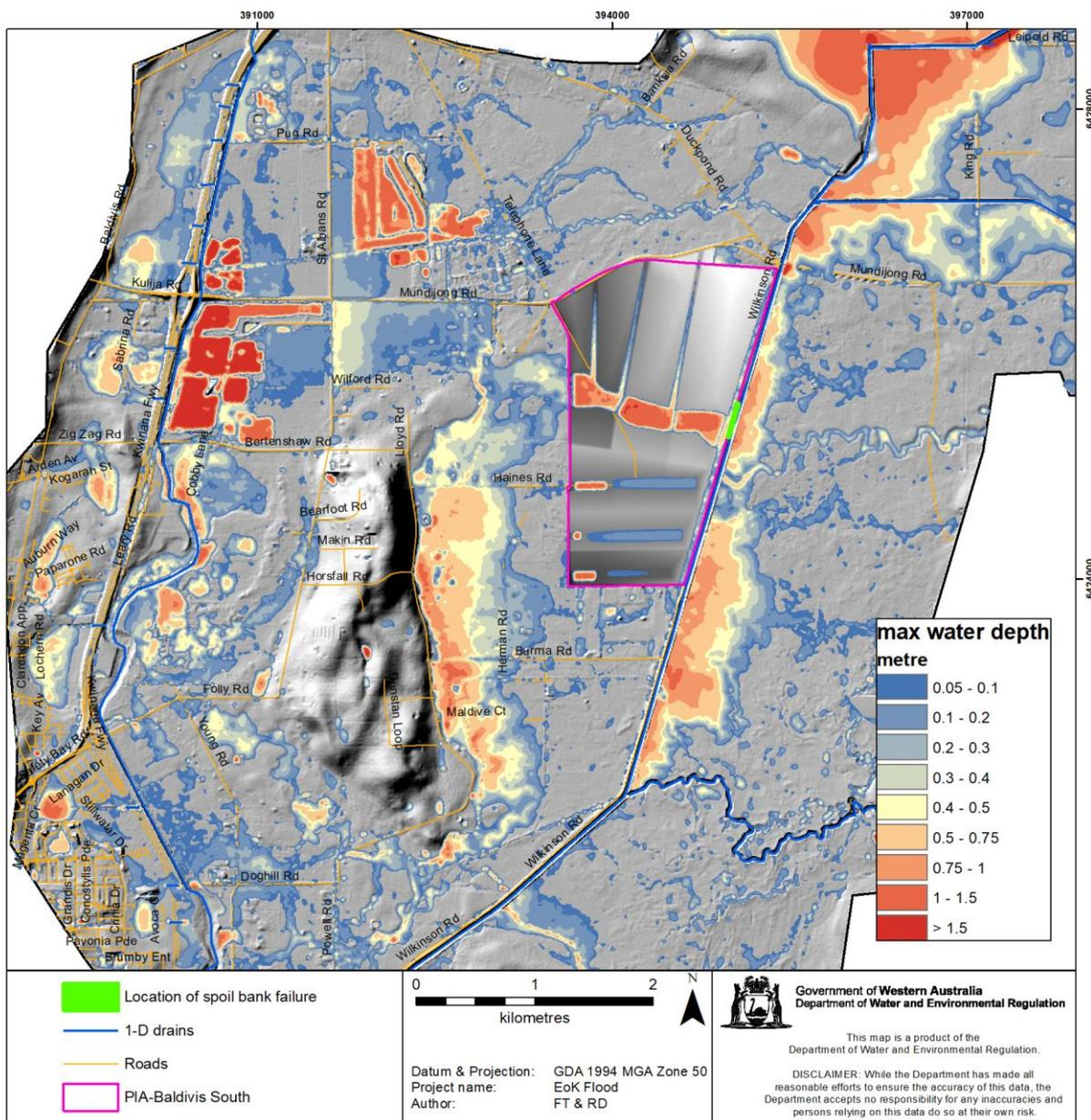
Figure 8-6 Maximum post-development flooding water depth focusing on North East Baldvis south of Mundijong Road precinct under 1% AEP 18-hour Tp1 rainfall
