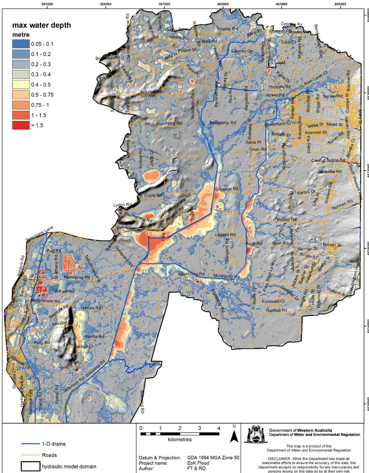
Figure C-7 Maximum flooding water depth with spoil bank intact (at 1% AEP 18-hour Tp1 rainfall)
