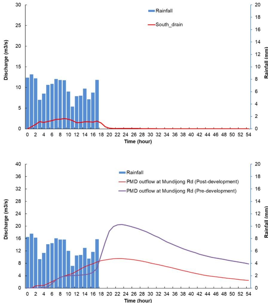
Figure 7-3 Hydrographs measured at the South Drain and the Peel Main Drain at Mundijong Road (see the locations in Figure 7-2)
