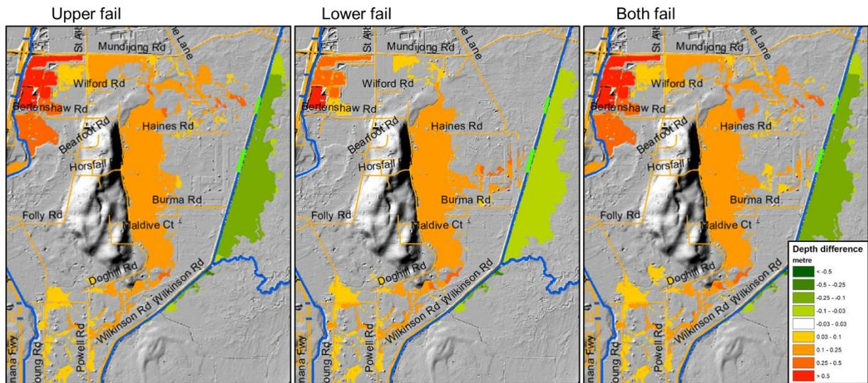
Figure 8-3 The flood difference maps between the failure scenarios and the Intact case (refer to Table 8-1 for all cases)
