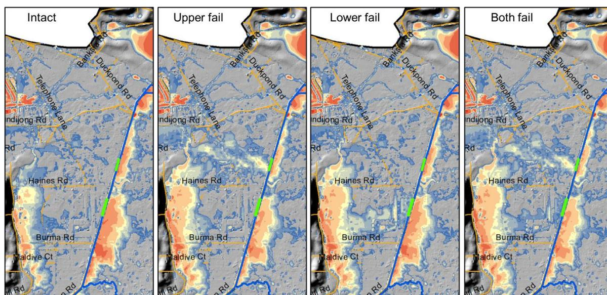
**Figure 8-2** The 1% AEP flood levels around the North East Baldvis south of Mundijong Road precinct from different spoil bank failure scenarios
