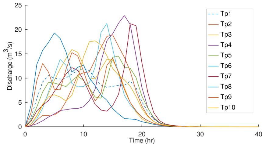
Figure 4-5 RORB Hydrographs at E07 for 1% AEP 18-hour duration rainfall at different temporal patterns
