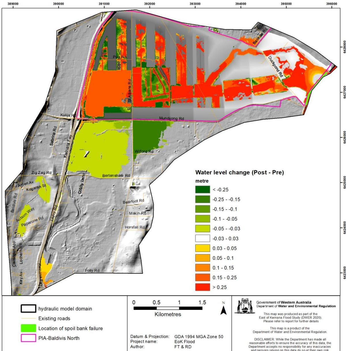
Figure 7-25 The impact of Option C on flooding outside the North East Baldvis north of Mundijong Road precinct
