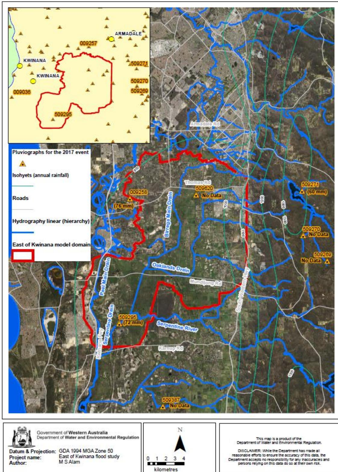
Figure 3-1 Pluviographs used in the hydrology and hydraulic models for the 2017 calibration event
