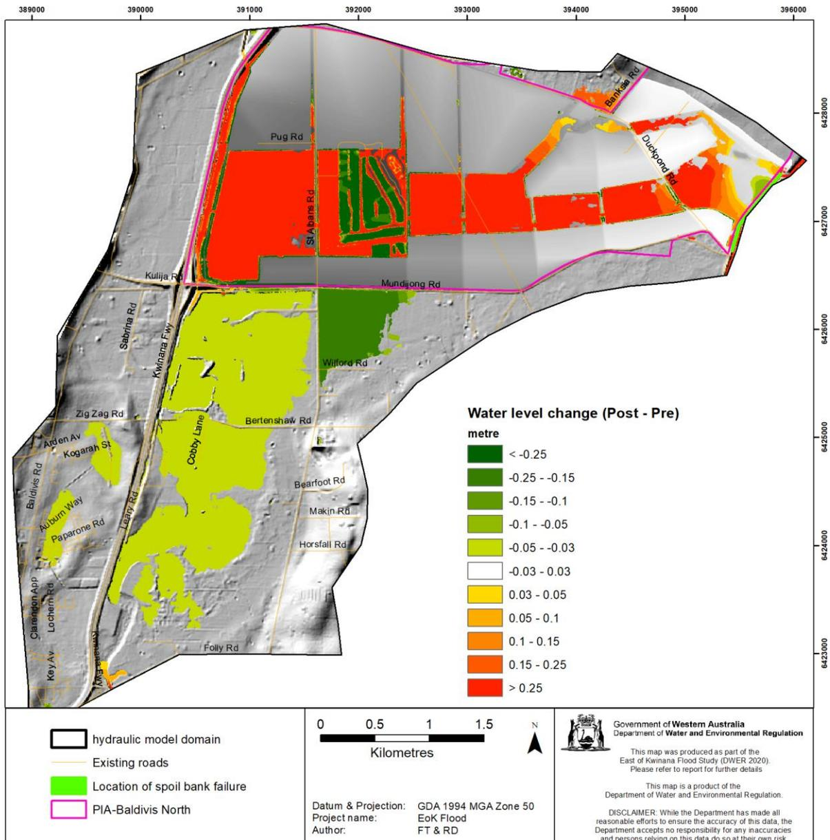
Figure 7-20 The impact of Option B+ to flooding outside the North East Baldvis north of Mundijong Road precinct
