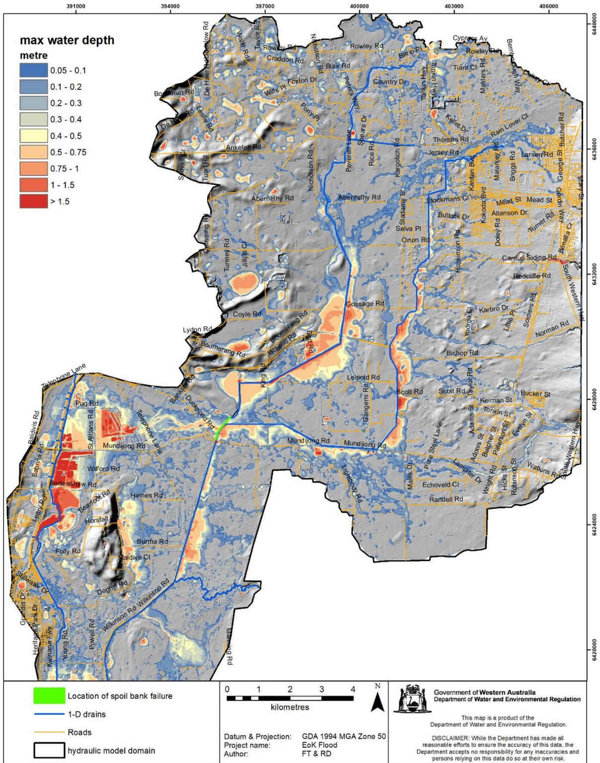
Figure C-9 Maximum flooding water depth at 1% AEP 18-hour  $Tp8$  front-loaded rainfall (with spoil bank fail 100%)
