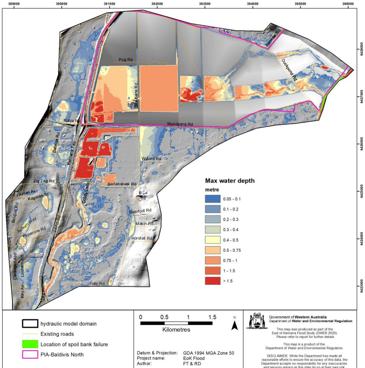
Figure 7-17 Maximum flooding water depth in Option B+ under 5% AEP 18-hour rainfall
