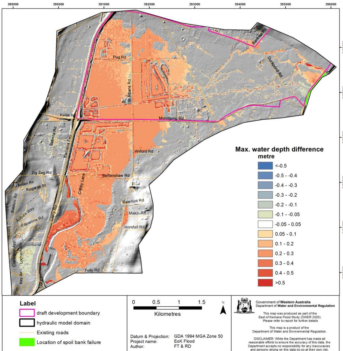
Figure 6-17 The difference in floodwater depth between the local (Figure 6-16) and the regional models (Figure 6-9). The depth between ±0.05 m was not shown.
