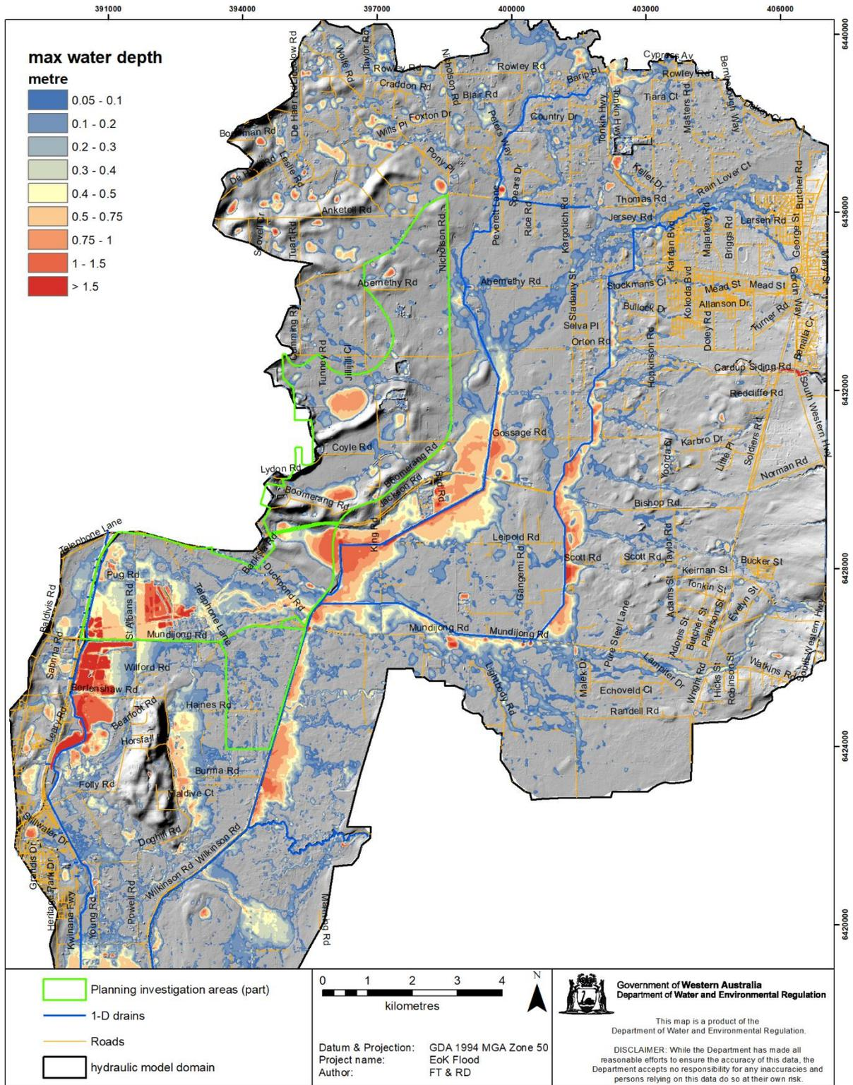
Figure 6-10 Floodplain extent mapping from 1% AEP design runs. This map was produced by a total of eight simulated water levels, as detailed in the text. Part of the PIAs covered by the present study is shown.
