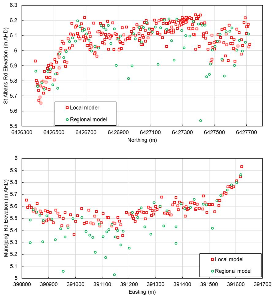
Figure 6-19 Comparison of node bathymetry sampled along the St Albans Road (top) and Mundijong Road (bottom) between the local and the regional model
