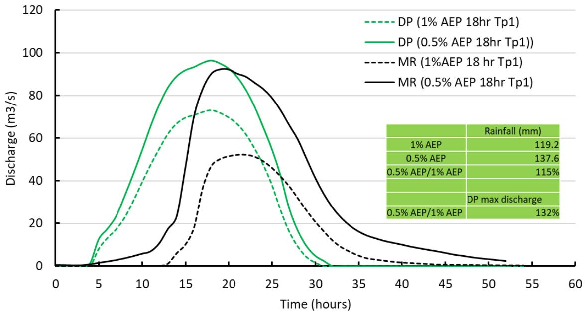
Figure 6-13 Comparison between the discharges from 1% AEP and 0.5% AEP rainfalls at two locations
