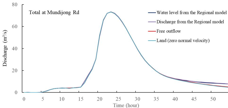
Figure 6-20 Comparison of the total discharges over the Mundijong Road from the local flood model by different boundary conditions
