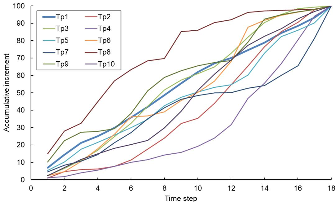
Figure 4-3 Temporal patterns of rainfall for the regional model at 18-hour design events (based on ARR2019, Region: S-SW Flatlands (West) and Area: 200 km<sup>2</sup>)
