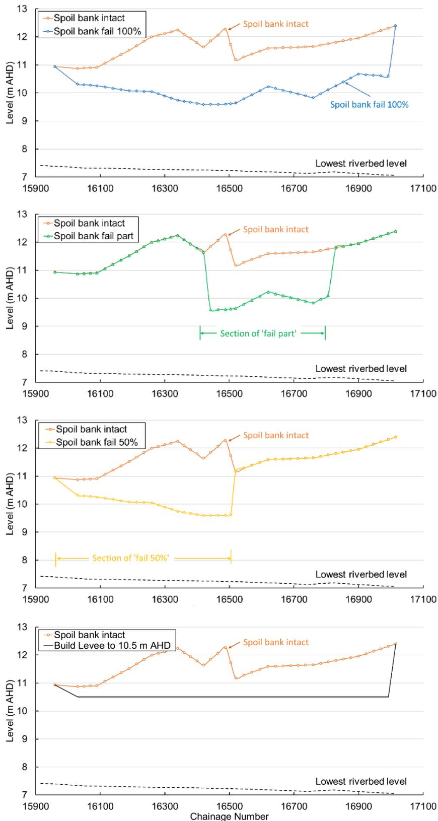
Figure 6-6 Comparison of the heights of the right bank of Birrega Main Drain in different spoil bank scenarios
