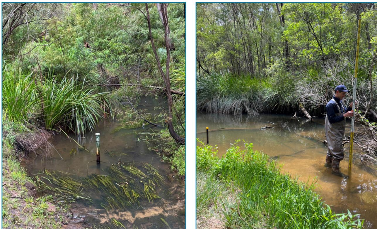
Figure 9 Surveying ecological features and installation of water level loggers at two environmental flow study sites in the Warren River catchment.
