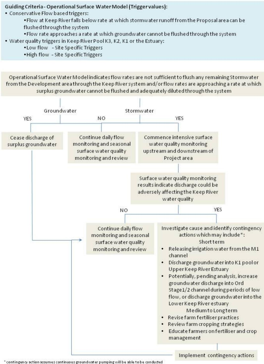
Figure 3 Decision flow chart for the management of stormwater and surplus groundwater discharge
