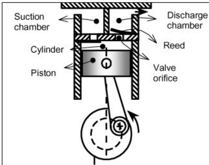
Figure 3.9 Schematic of Reciprocating Compressor
