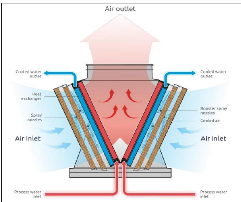
Figure 3.6 Schematic of Adiabatic Cooler
