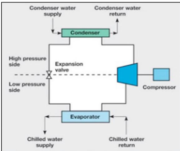
Figure 3.5 Schematic of Chiller System
