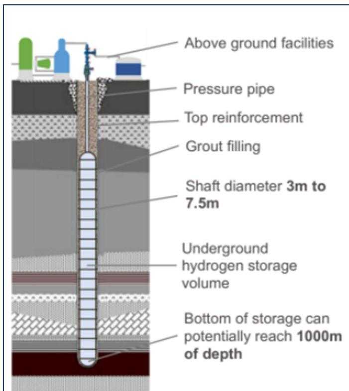
Figure 3.15 Vertical Shaft Hydrogen Storage
