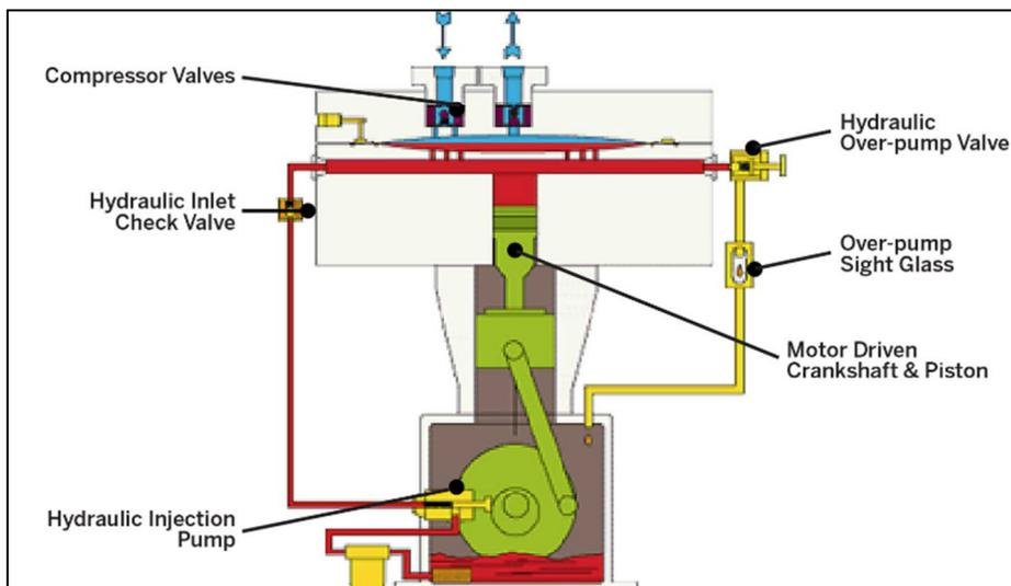
Figure 3.10 Schematic of Diaphragm Compressor
