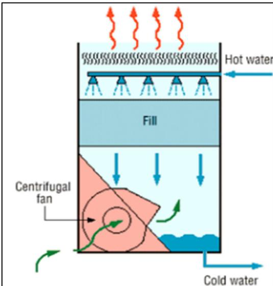
Figure 3.2 Schematic of Evaporative Cooling Tower
