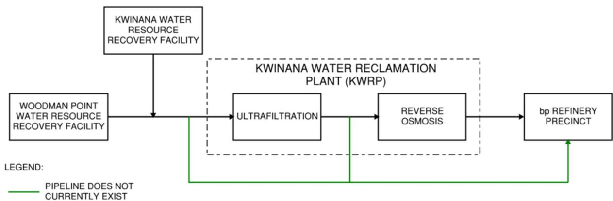
Figure 3.7 Possible Alternative Cooling Water Supply Options
