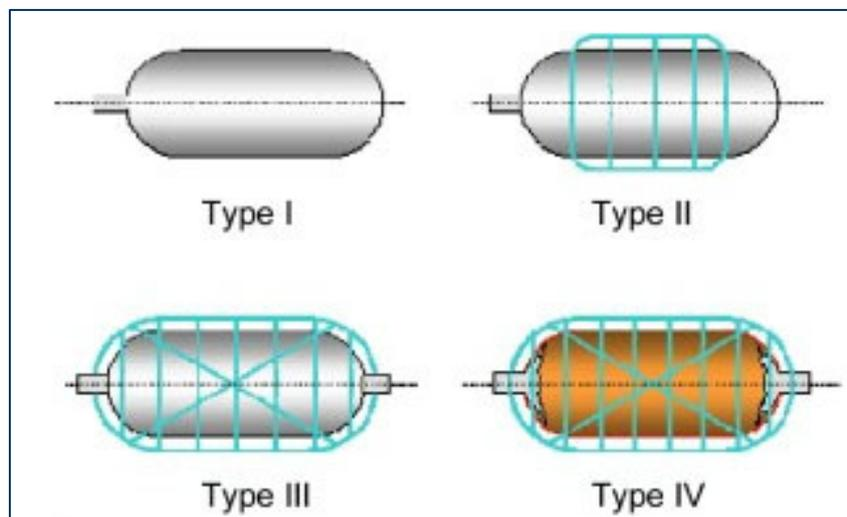
Figure 3.11 Types of Hydrogen Storage Vessels
