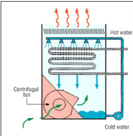
Figure 3.3 Schematic of Closed-Loop Evaporative Cooling Tower
