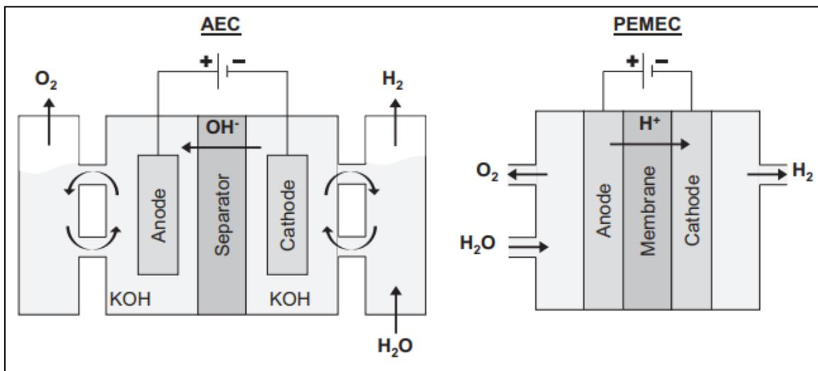
**Figure 3.1 Alkaline Electrolysis Cell (AEC) and Polymer Electrolyte Membrane Electrolysis Cell (PEMEC)**
