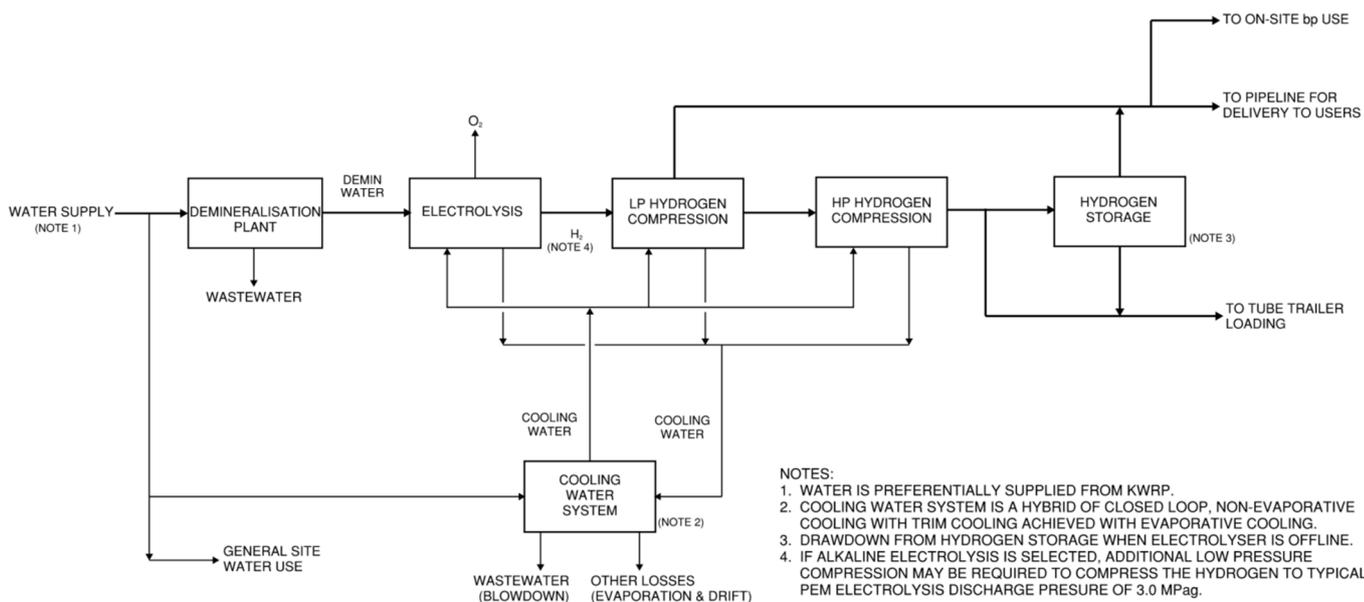
Figure 2.2 Block Flow Diagram of the Hydrogen Production Facility
