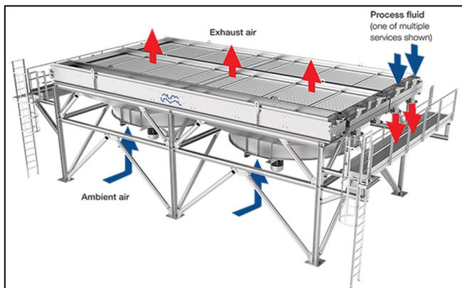
Figure 3.4 Schematic of Fin Fan Cooling
