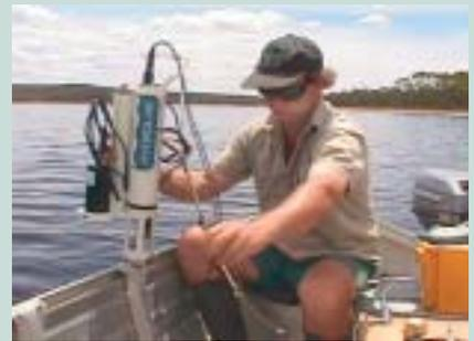
Figures 4, 5 and 6 (top to bottom): Analysing nutrient samples in a laboratory and sampling from the boat in Wilson Inlet with a Hydrolab instrument.
