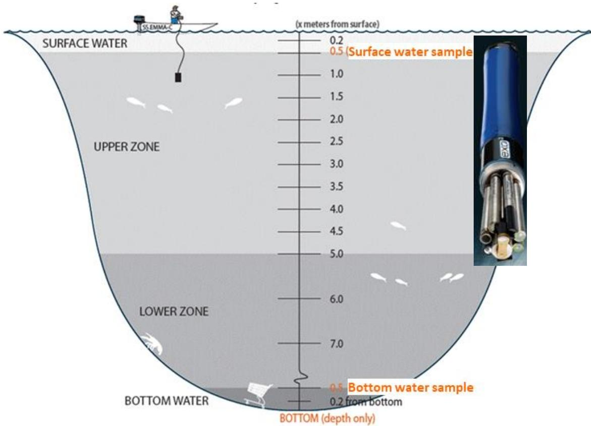
Figure 4 Profiling and water sampling in Wilson Inlet. The insert shows the EXO2 used for physical-chemical profiles.
