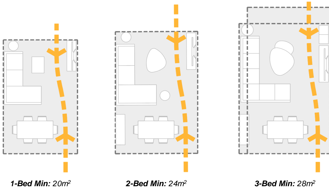
Figure 10: Optimum living space proportions showing furniture layouts and circulation route. The dimensions can be scaled up relative to number of dwelling bedrooms.
