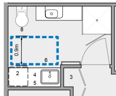
Figure 20: Laundry integrated within bathroom – Open joinery
