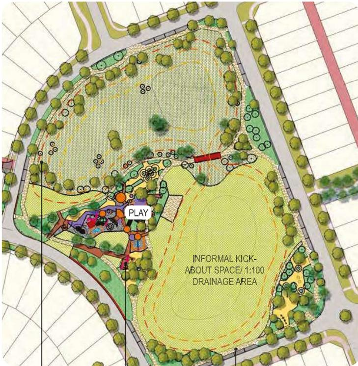
VEGETATED DRAINAGE BASINS WITH SUB-SOIL DRAINAGE
