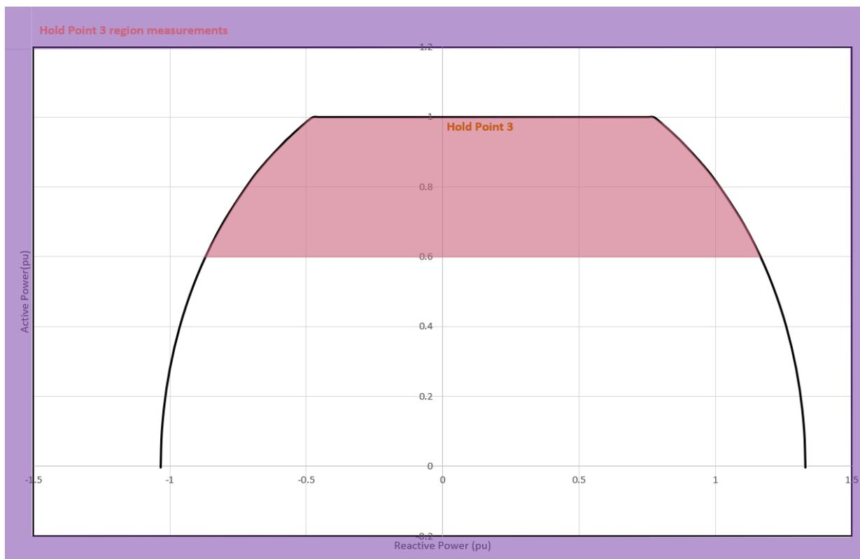
5.4.4. Generating System Reactive Power reference test (HP3\_RPT)
