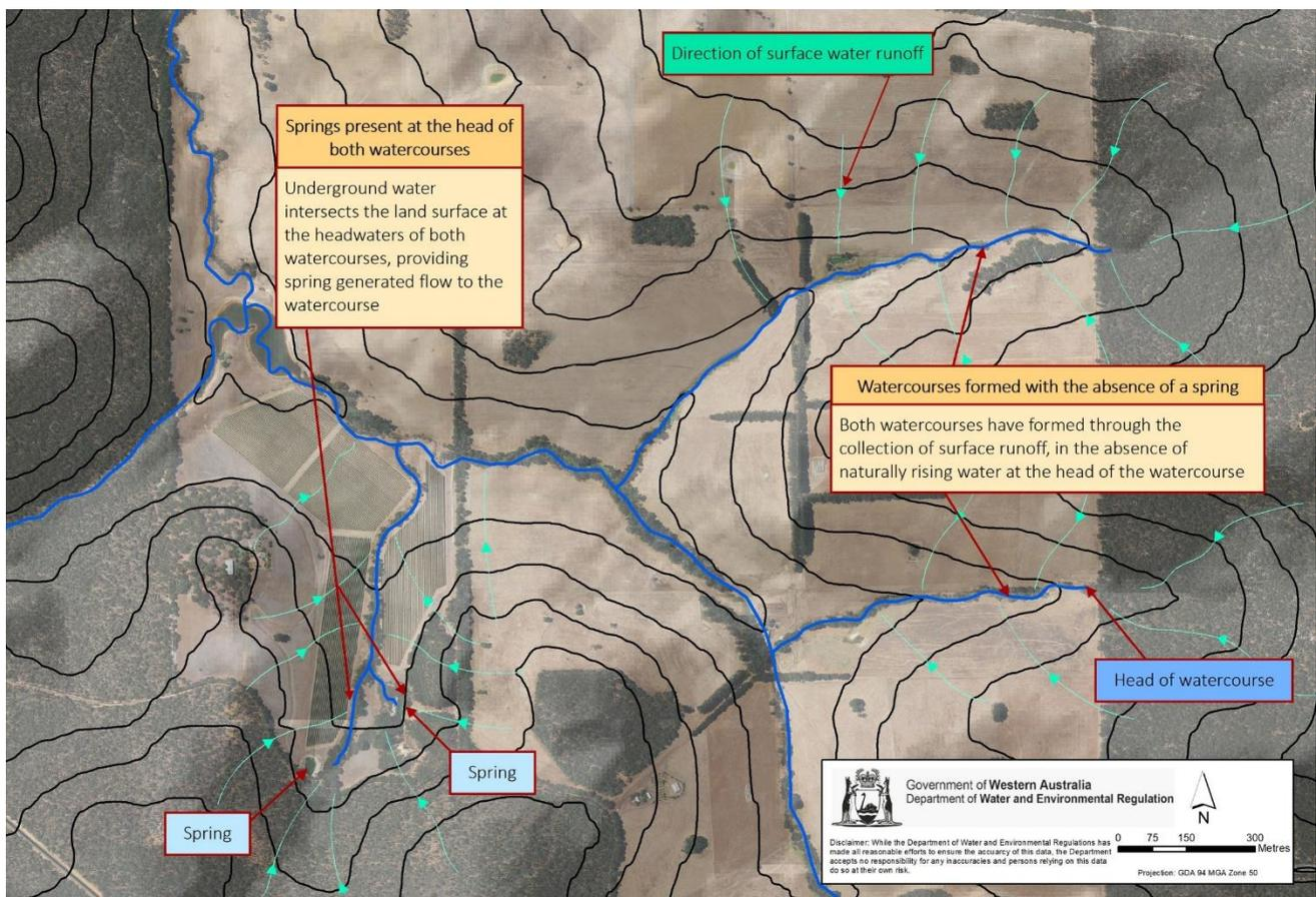
**Figure 1** Watercourses are present in the landscape where surface runoff and/or subsurface flow collect to flow in a single direction across the land surface, and may or may not have a spring at the head.
