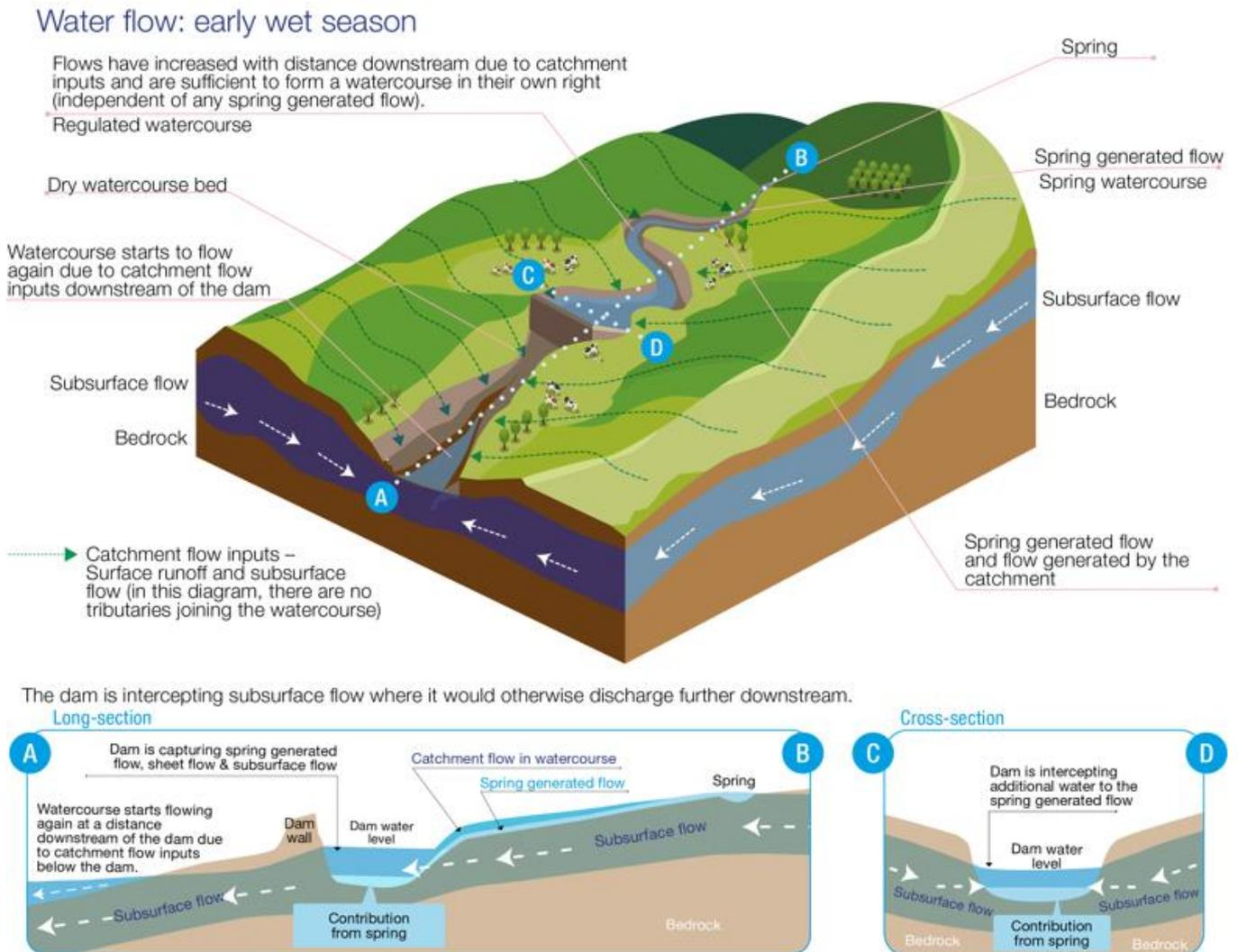
**Figure 2** Diagram showing the catchment hydrology and flow dynamics that may occur on a property following the commencement of the wet season. The diagram shows how flow in a watercourse may change from the head of a watercourse to the downstream property boundary. In this scenario, underground water levels have risen in response to rainfall and the spring is discharging water. The flow volume from the spring does
