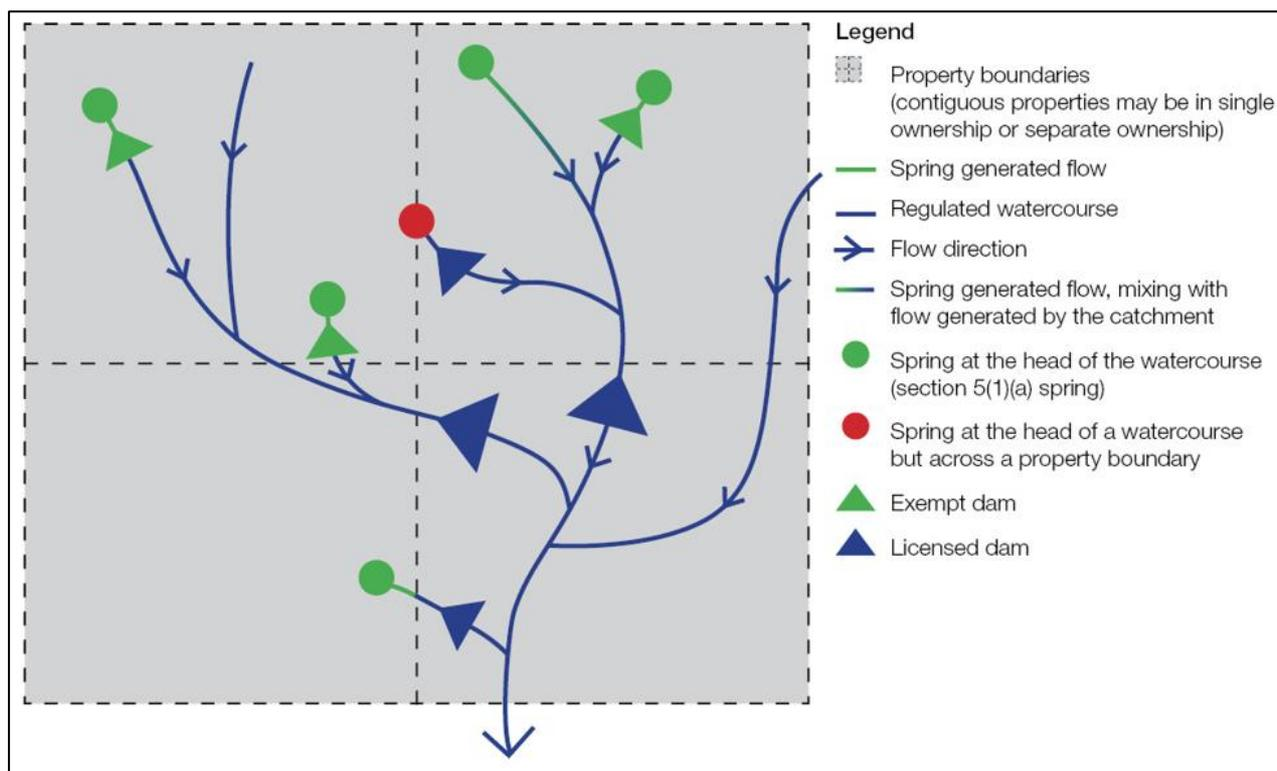
**Figure 6** A spring that exists over a property boundary is not a section 5(1)(a) spring. The spring must be wholly within a property boundary and the water flow generated by that spring must be taken within that property boundary to be exempt from regulation.
