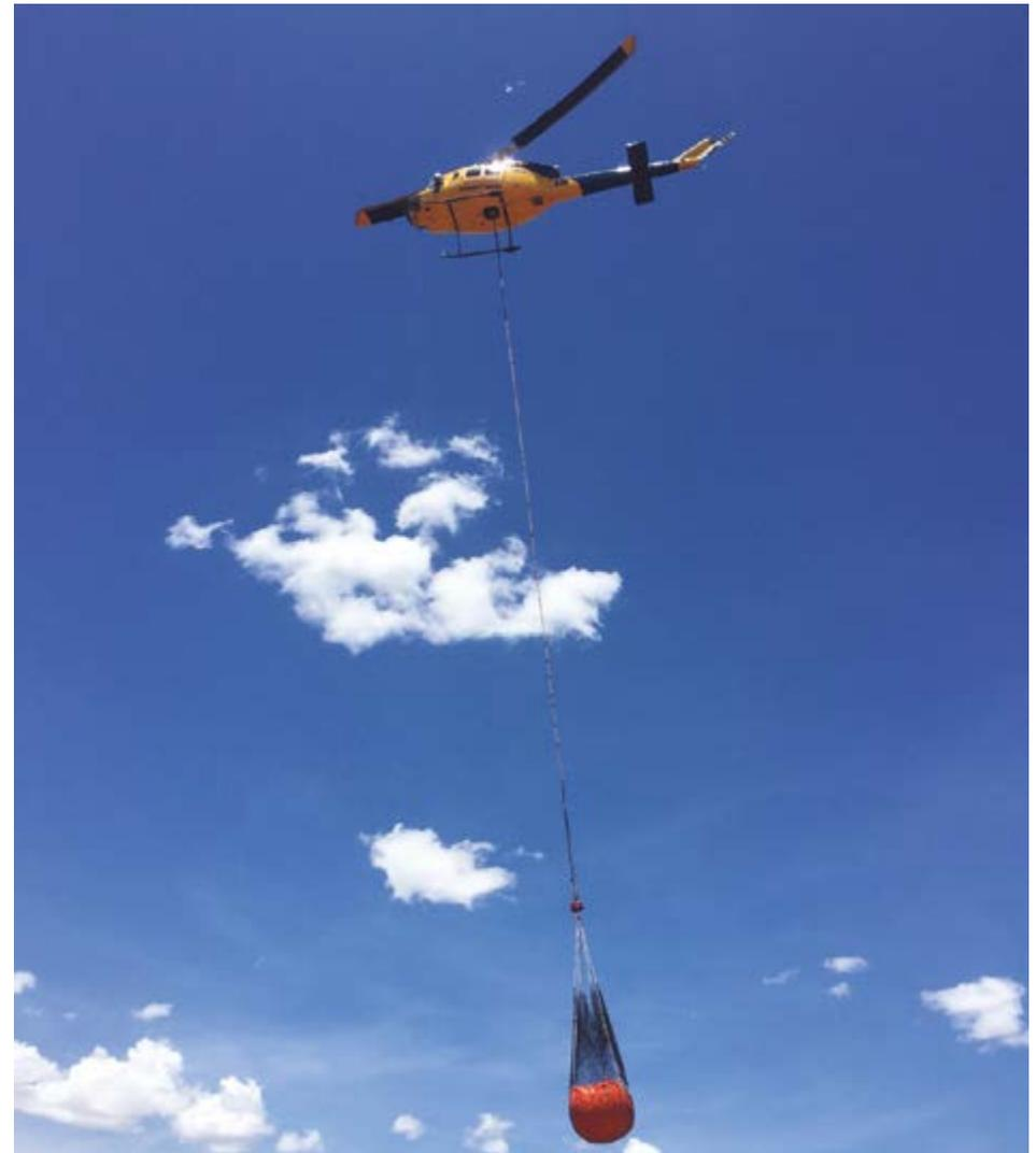
Figure 18. Bell 412 helicopter delivering fuel
