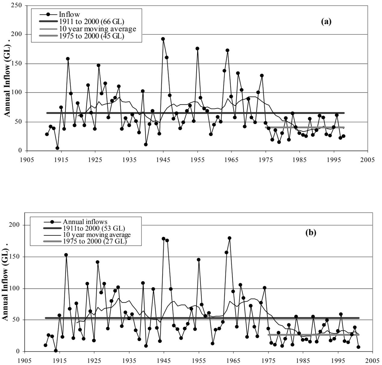
Figure 6. Modelled and observed data for inflows into the (a) Serpentine and (b) Canning reservoirs
