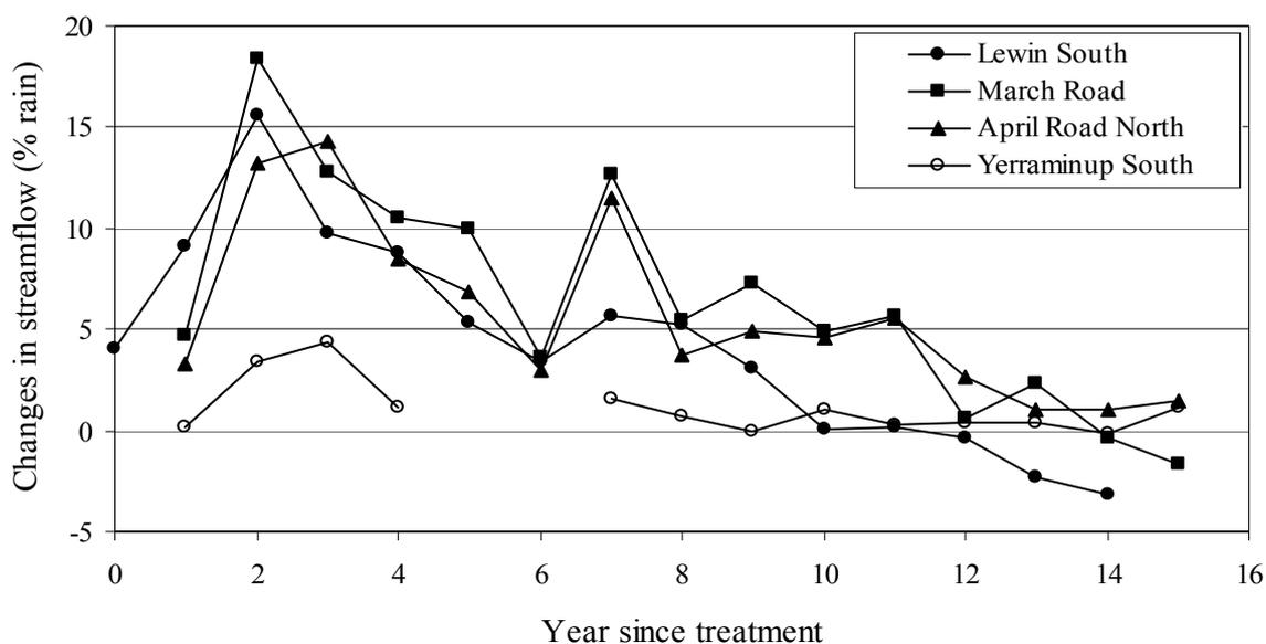
Figure 10. Streamflow response to logging experimental catchments in the Southern Forest
