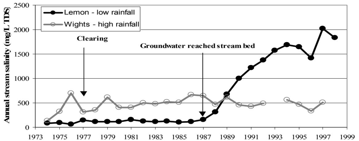
Figure 9. Increase in stream salinity due to clearing for agriculture
