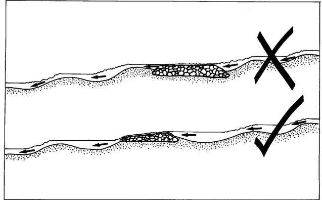
Figure 5: Take advantage of natural high points along the profile when siting a crossing.
