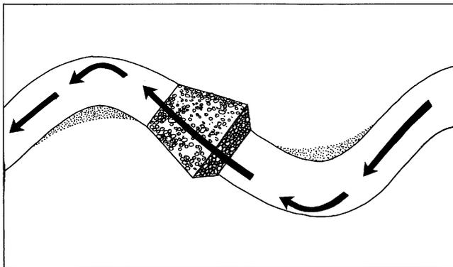
Figure 4: Crossings should be built on a straight stretch of river or at a crossover point in the middle of a meander.
