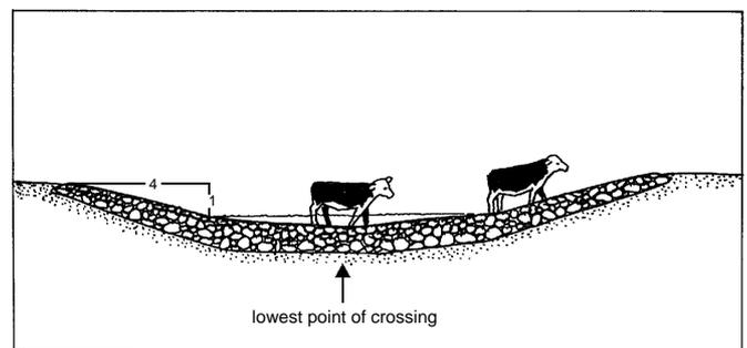
*Figure 2: The basic geometry of a livestock crossing.*
