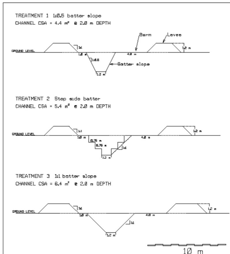
**Figure 19 Wubin batter trials – cross sections**
