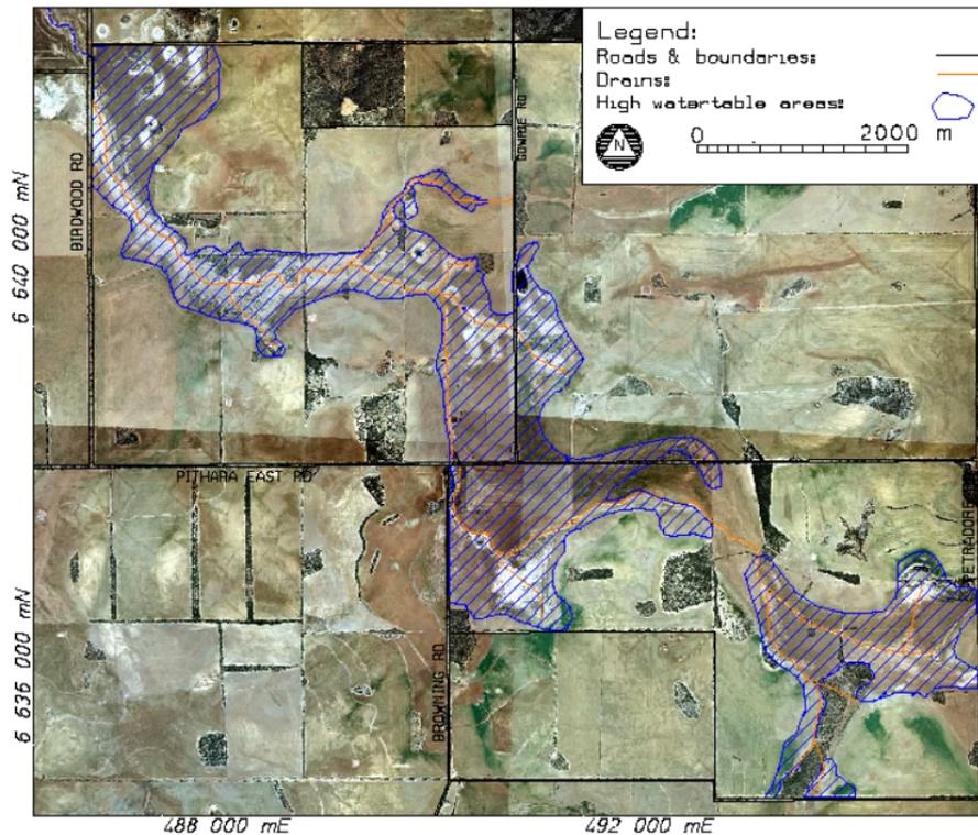
**Figure 4 Pithara drainage project – site layout**
