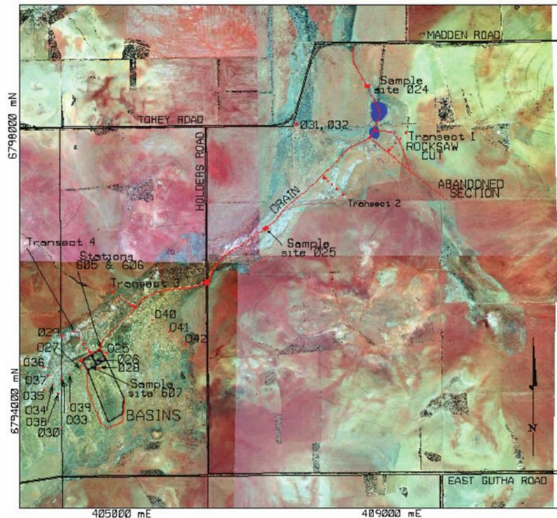
**Figure 6 Morawa drainage project – site layout**
