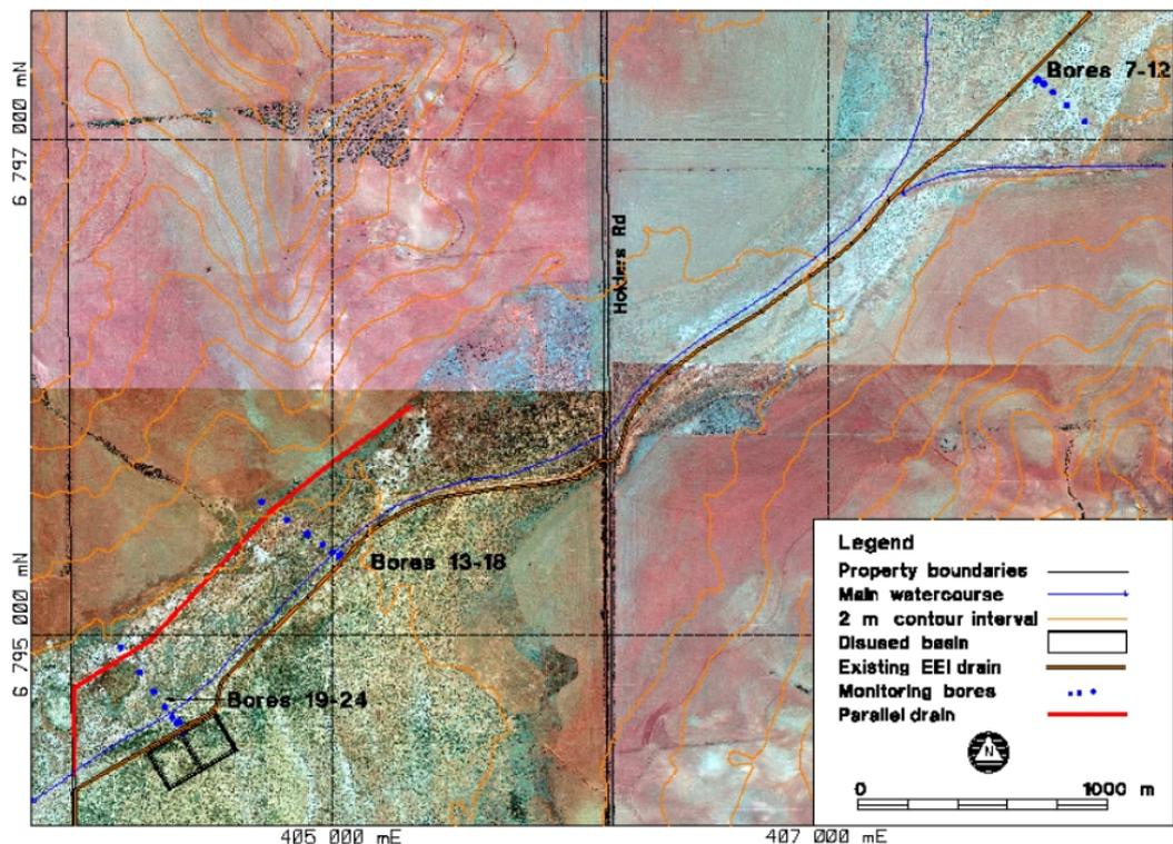
**Figure 12 Morawa parallel drains – site layout**
