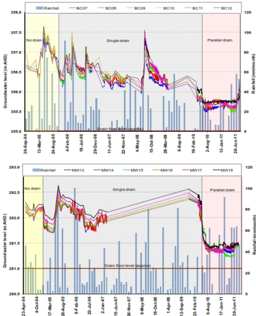
**Figure 26 Watertable response to parallel drains: hydrographs from monitoring transect bores at Beacon (top) and Morawa (bottom) show very different watertable response at the same site following the construction initially of single drains (2004-2005) and later a parallel drain (2010) (from Cox and Tetlow, 2015)**
