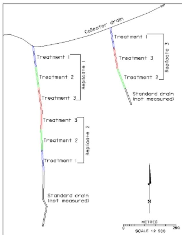
**Figure 18 Wubin batter trials – site layout**
