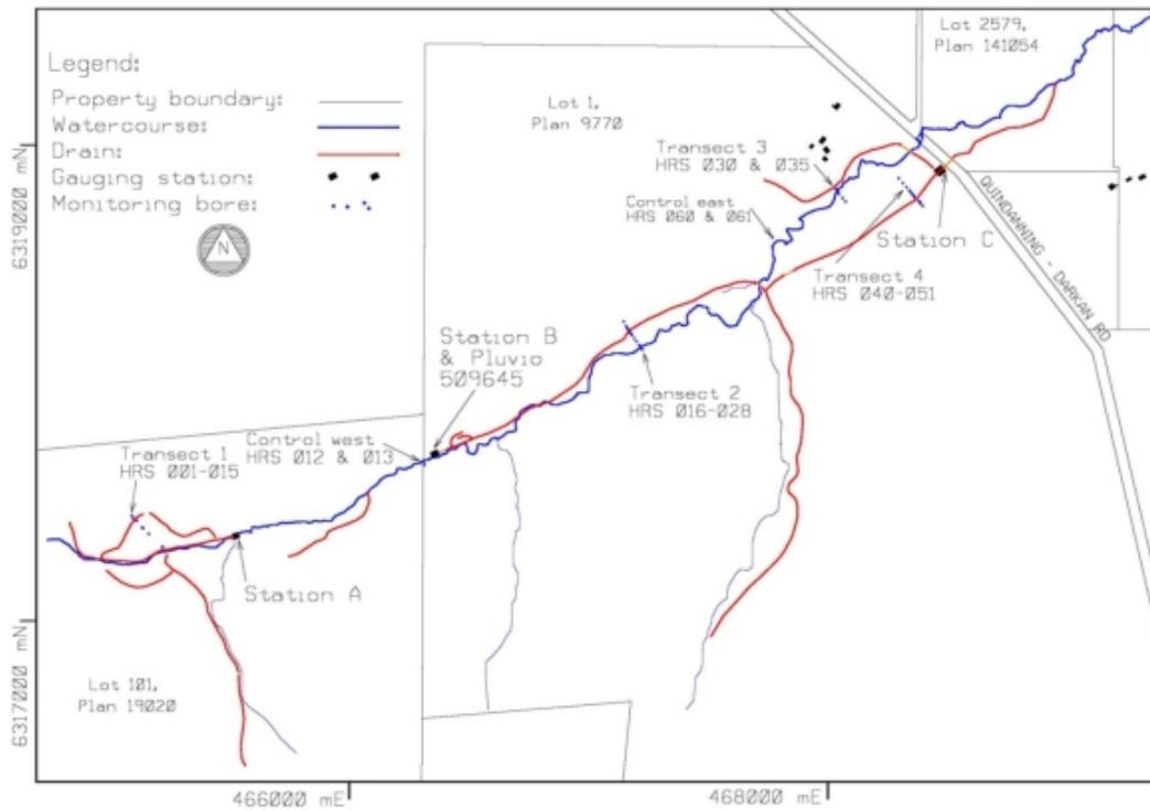
**Figure 8 Hillman River South drainage project – site layout**
