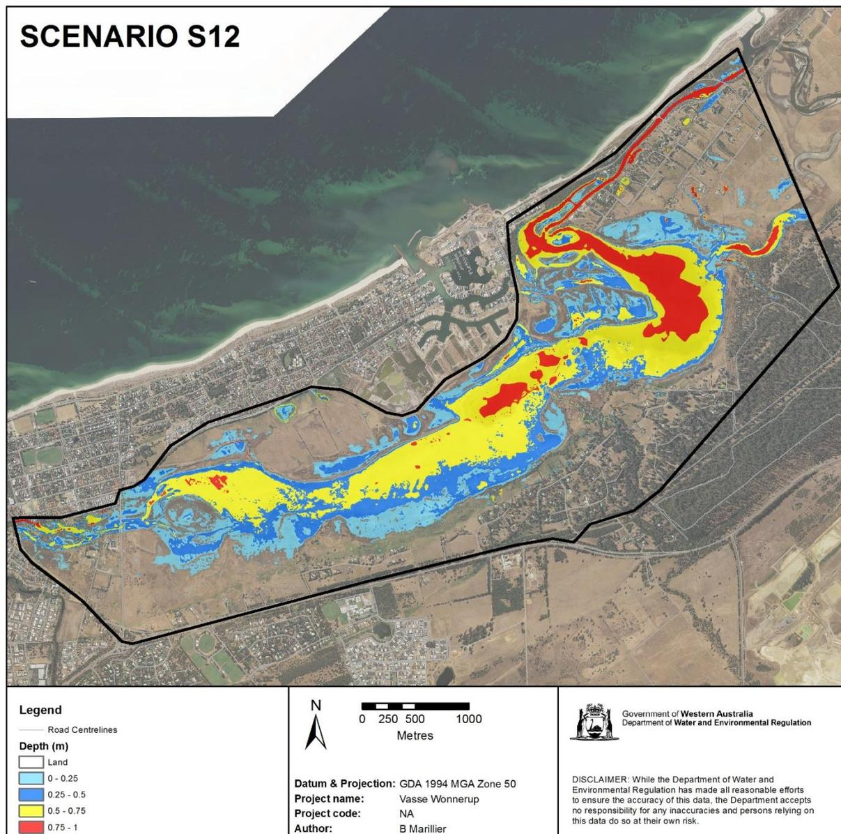
Figure 5-36: Estimated average maximum extent of seawater inundation in April with water level at 0.42 mAHD, surge barriers removed (S12)
