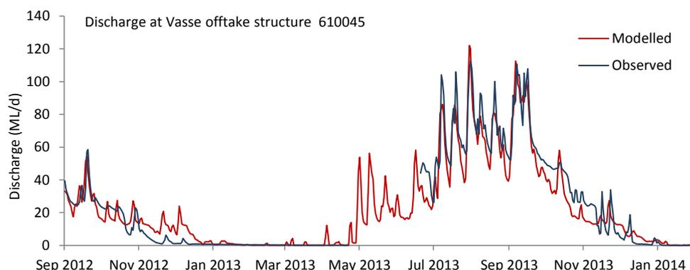
Figure 4-8: Modelled and observed discharge at the Vasse offtake for 2012 and 2013
