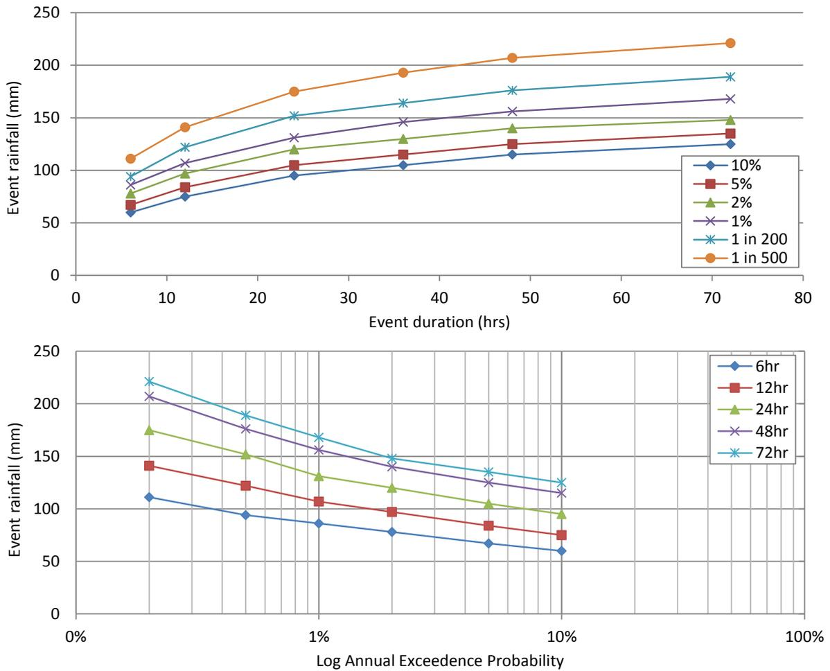
Figure 3-1: Rainfall intensity frequency duration (IFD) data plotted with event duration versus event rainfall for different AEPs (top); and rainfall IFD probabilistic plot for log AEP versus event rainfall for different event durations (bottom)
