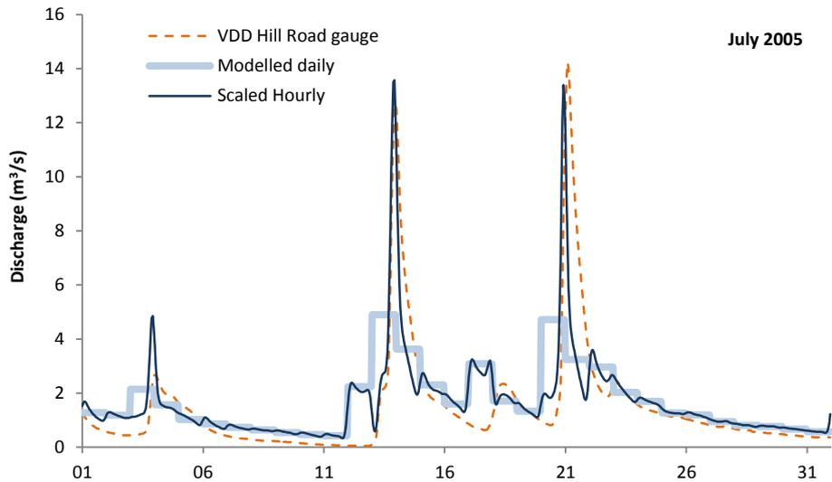
*Example of daily to hourly scaling of flows based on gauged hourly flow and modelled daily flow*
