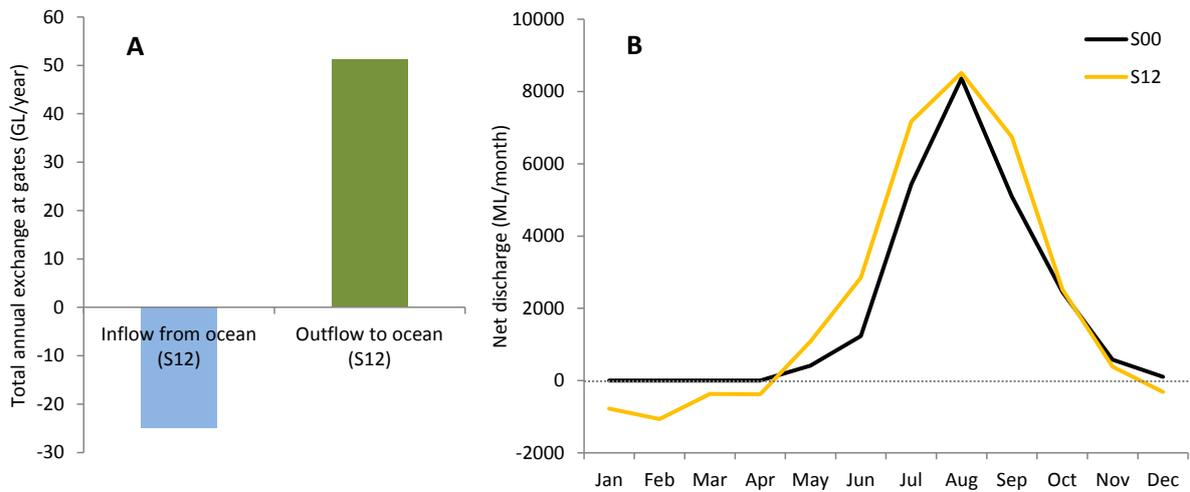
Figure 5-35: Total average volume of water exchanged between the ocean and Vasse Estuary in the absence of surge barriers (A) and average monthly net discharge (B). Negative discharge indicates inflow from the ocean
