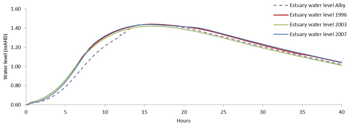
Figure 4-3: Simulated Vasse Estuary water levels for ocean boundary conditions from Figure 4-2 for the 1% AEP flow event
