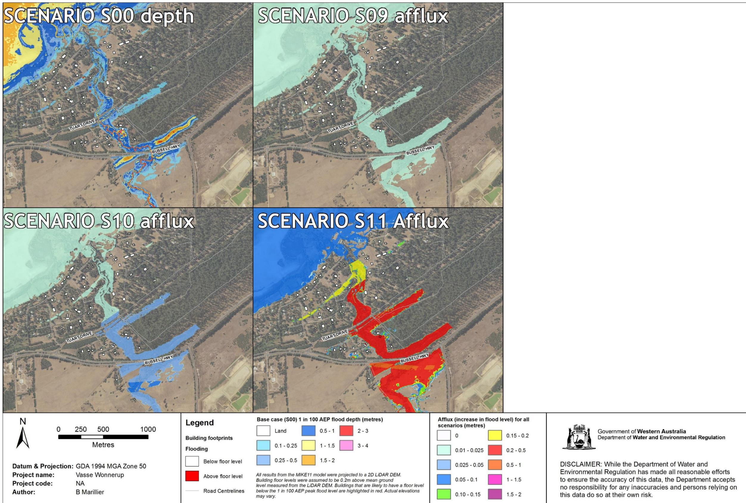
Figure 5-16: Extent of 1% AEP flooding on the Lower Sabina River for S00, S09, S10 and S11
