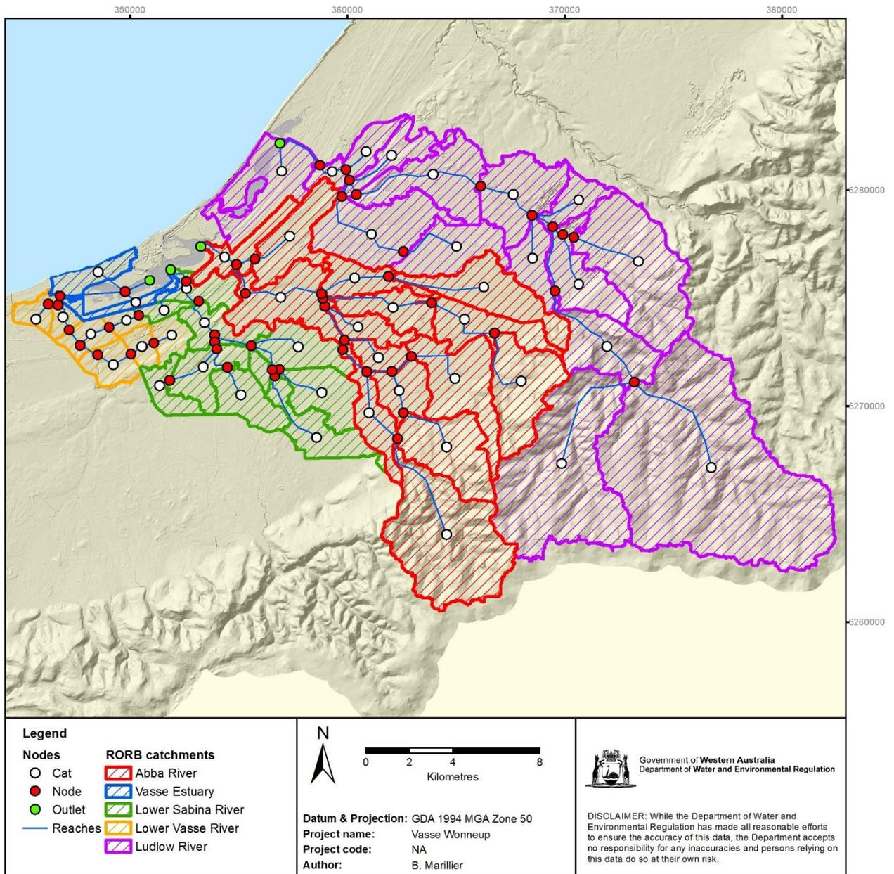
Figure 3-2: Runoff Routing B models in the Vasse-Wonnerup estuary catchment
