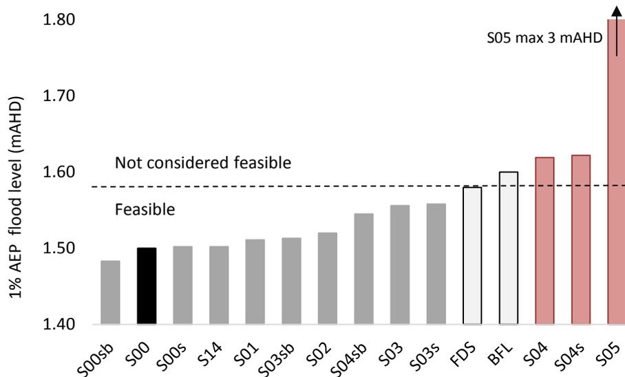
Figure 5-17: Feasibility of Lower Vasse River reconnection options relative to floodplain development strategy (FDS) and building floor level (BFL) upstream of Causeway Road bridge
