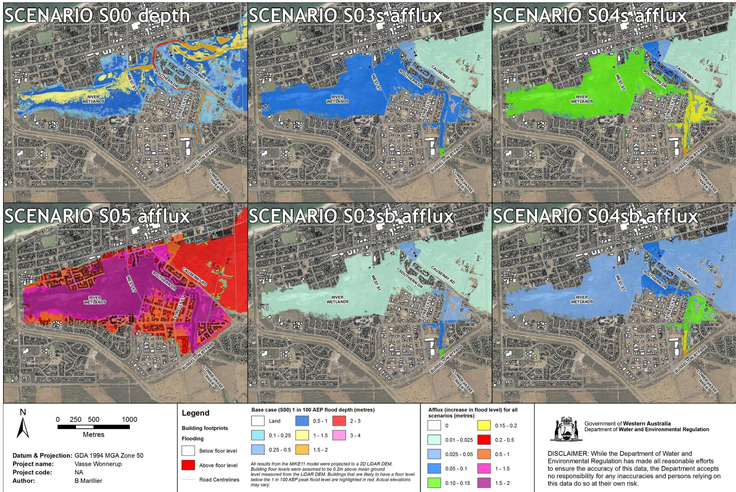
Figure 5-13: Extent of 1% AEP flooding on the Lower Vasse River between Busselton Bypass and the Butter Factory weir. Base case and reconnection scenarios
