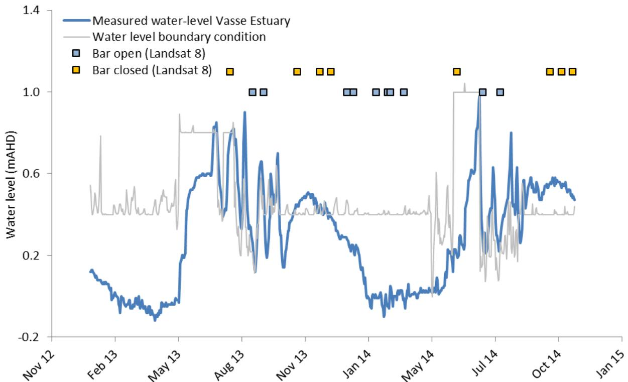
Figure 4-4: Artificial water-level boundary condition including the effects of check boards and sand bar closure
