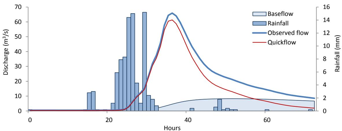
Figure 3-3: Example of baseflow separation for the 1997 event on the Ludlow River
