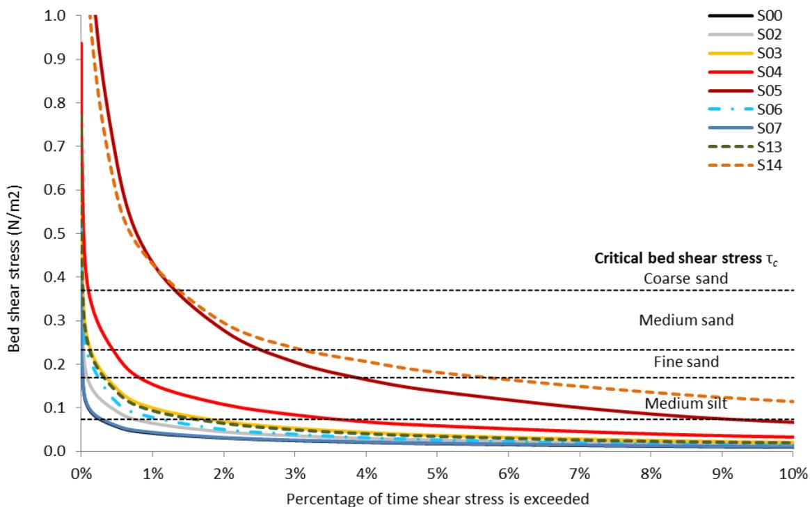
Figure 5-25: Bed shear stress exceedence in the Lower Vasse River (Lower Vasse River 7)
