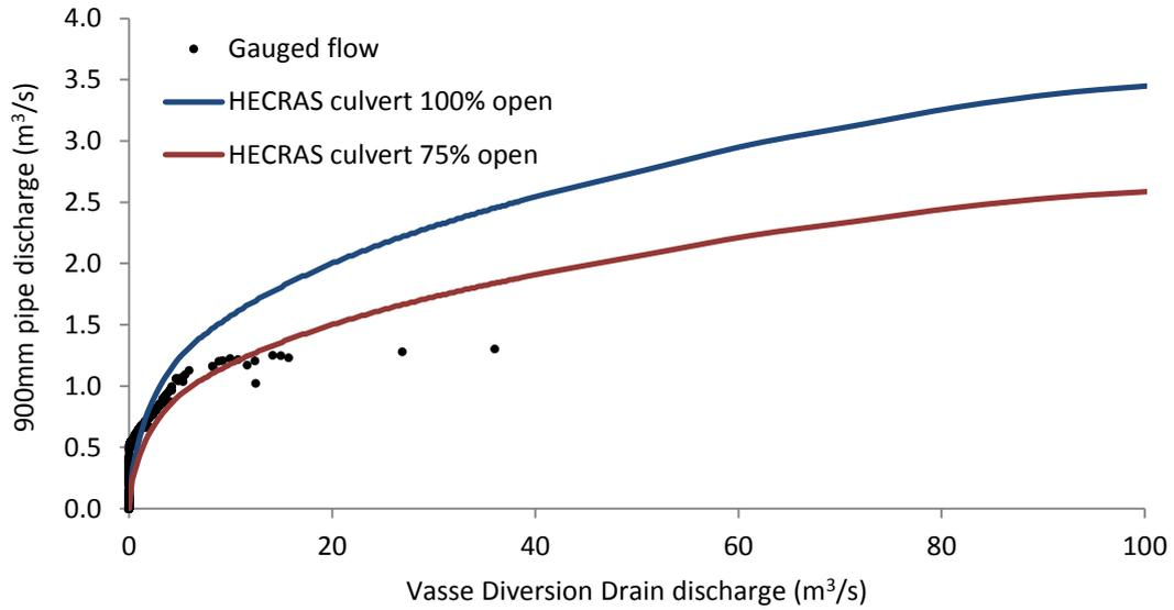
Rating curve generated using a HEC RAS model of a section of the Vasse Diversion Drain with a lateral outflow culvert 900 mm in diameter. Black data points indicate gauged flow on the Vasse Diversion Drain (610014) and on the offtake structure (610045) for data collected between 2012 and 2014.
