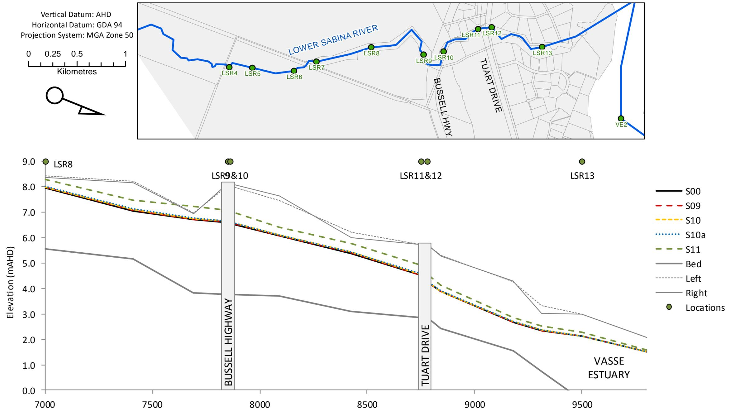
Figure 5-15: Long-section of peak flood levels for the 1% AEP event on the Lower Sabina River at Bussell Highway and Tuart Drive
