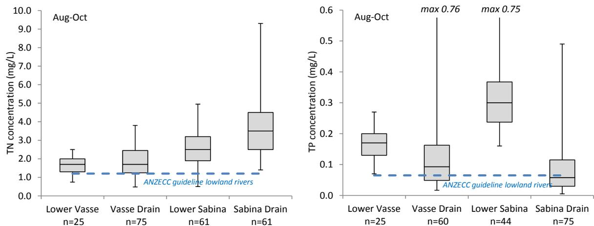
Figure 2-11: Total nitrogen and total phosphorus concentrations August to October
