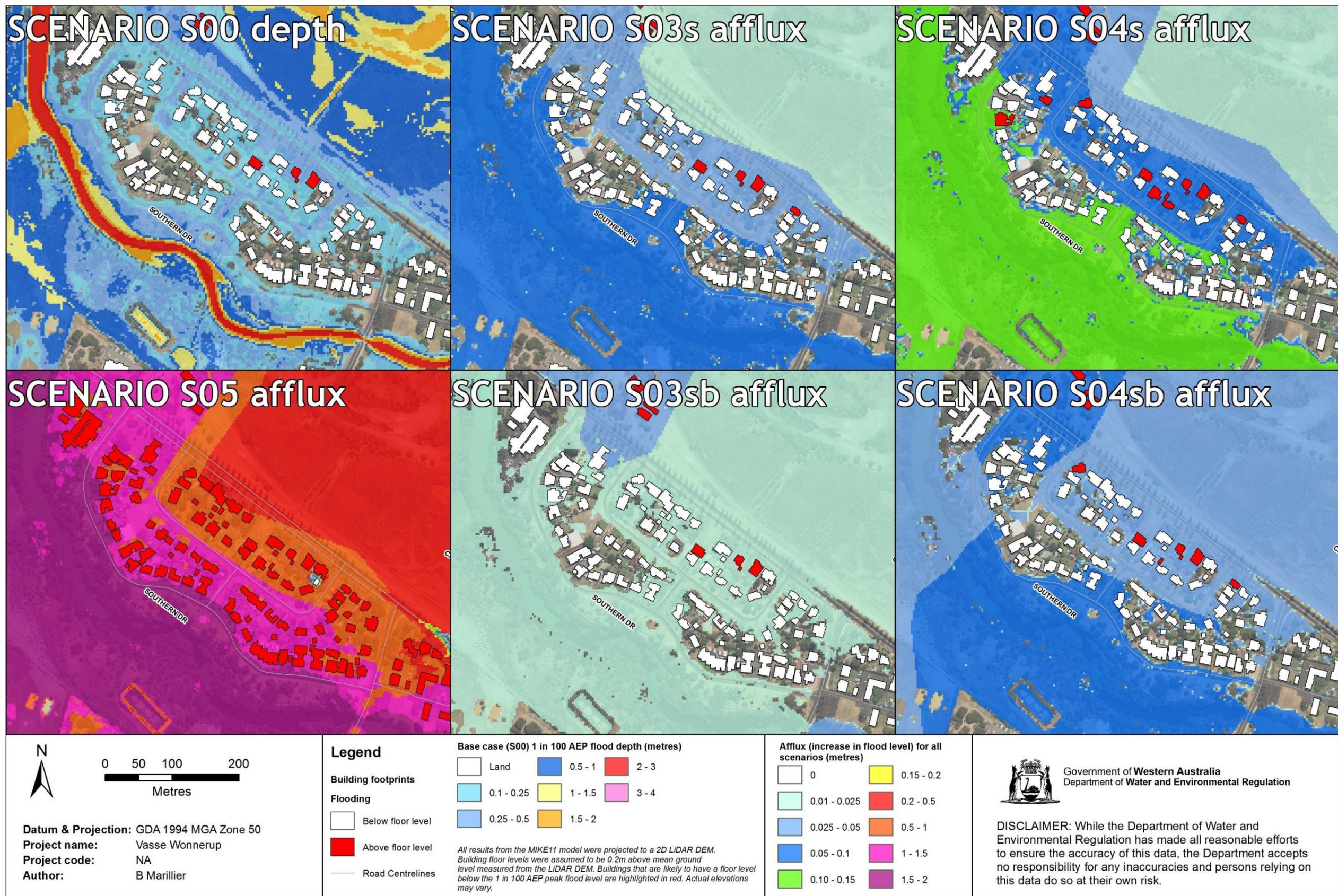
Figure 5-14: Extent of 1% AEP flooding on the Lower Vasse River between Southern Drive and Causeway Road. Base case and reconnection scenarios
