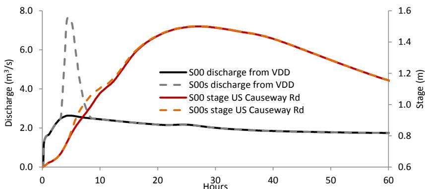
*Figure 5-9: Comparison of base case and spillway scenario flows for the 1% AEP event. Increased discharge from the spillway does not increase peak flood level on the Lower Vasse River*
