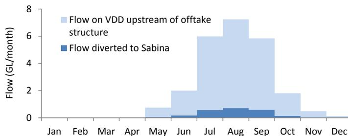
Figure 5-7: Average monthly reduction of flow at the Vasse Diversion Drain offtake structure with flow diversion upstream at Sabina Diversion weir
