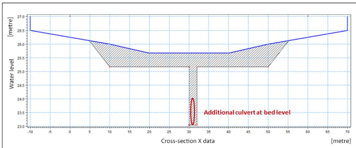
Figure 5-5: Addition of culverts at Sabina Diversion weir
