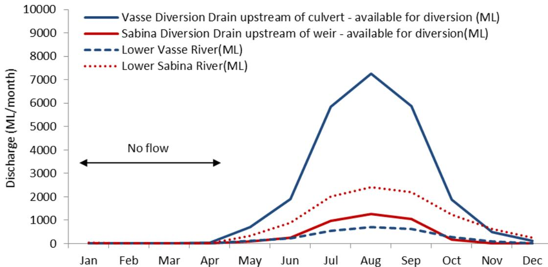
Figure 2-7: Modelled average monthly flows on the Vasse and Sabina diversion drains upstream of diversion structures and downstream Lower Vasse and Lower Sabina river flows (2001–14)
