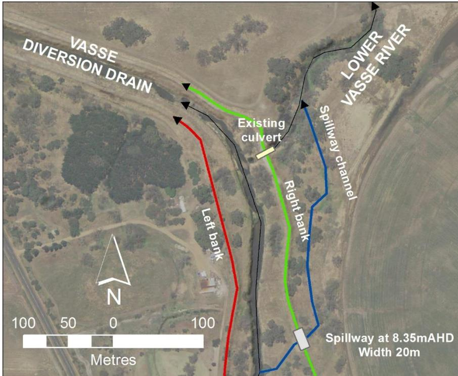
Figure 5-1: Spillway diagram
