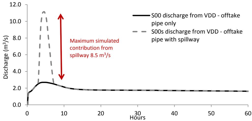
The target spillway peak discharge was 7 m<sup>3</sup>/s but a 20% safety factor was applied, resulting in a conservative spillway contribution of 8.5 m<sup>3</sup>/s, and a total contribution through the offtake structure and spillway of 11.1 m<sup>3</sup>/s.
