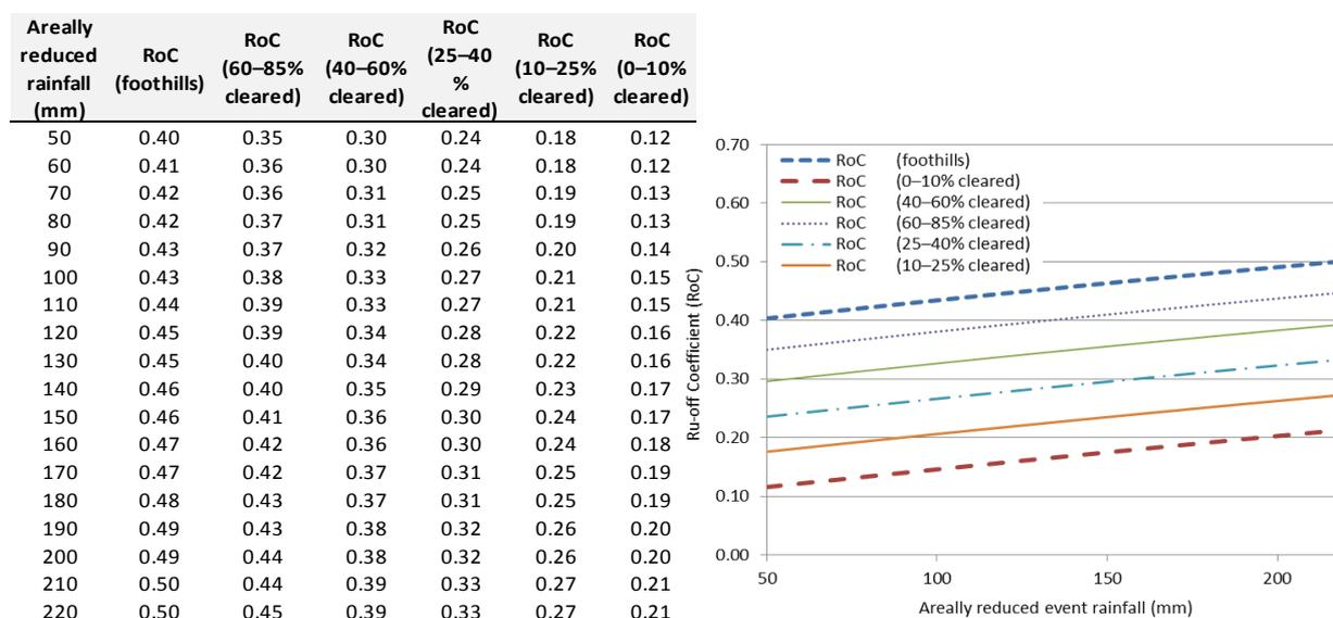
Table 3-6: Regional Runoff Routing B coefficients developed by the Water Corporation and GHD (2013) for different proportions of land clearing. Additional categories of 40–60% cleared and 10–25% cleared were interpolated
