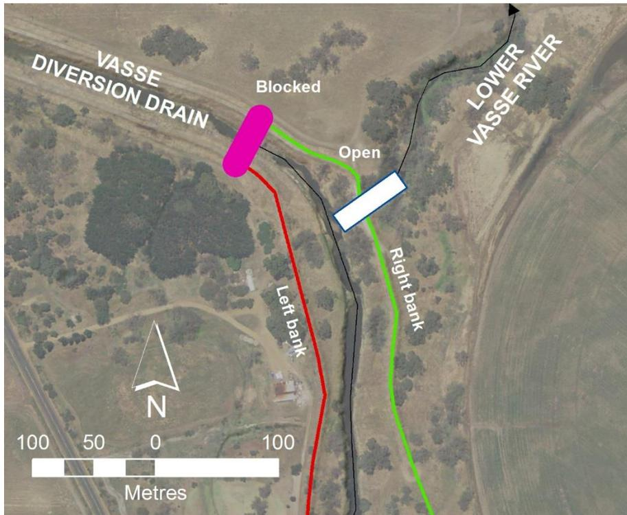
Figure 5-4: Full reconnection of Vasse Diversion Drain
