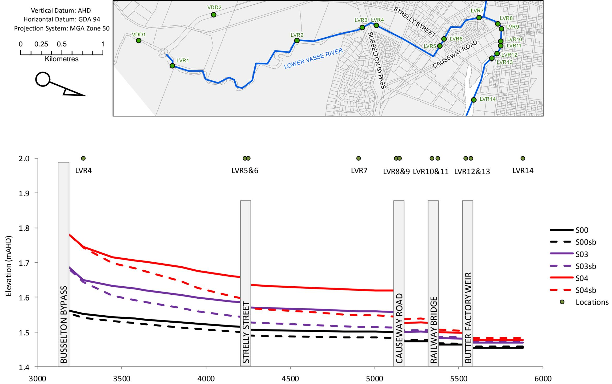
Figure 5-11: Long-section showing impact of Causeway Road bridge upgrade on 1% AEP flood levels for the Lower Vasse River (note vertical axis range 1.4 to 2 mAHD)
