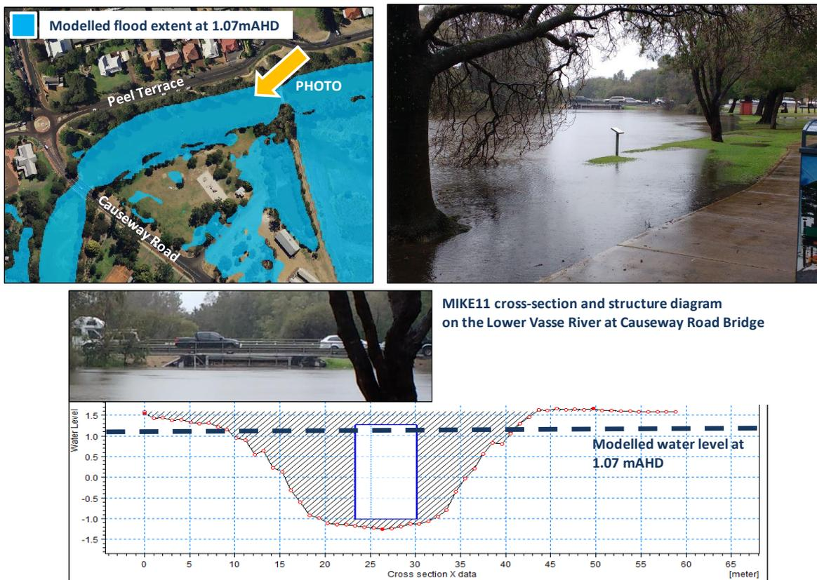
Figure 4-7: Photo showing flooding in the Lower Vasse River and modelled peak water levels July 2016
