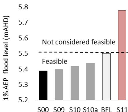
Figure 5-18: Feasibility of Lower Sabina River reconnection options relative to building floor level (BFL) for residential properties upstream of Tuart Drive
