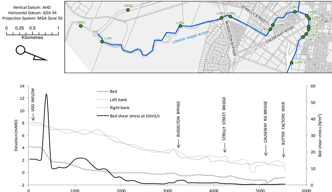
Figure 5-26: Long-section of bed shear stress for steady-state conditions with an inflow of  $10 \text{ m}^3/\text{s}$  for the Lower Vasse River. Where the river is steep and narrow, bed shear stress is highest
