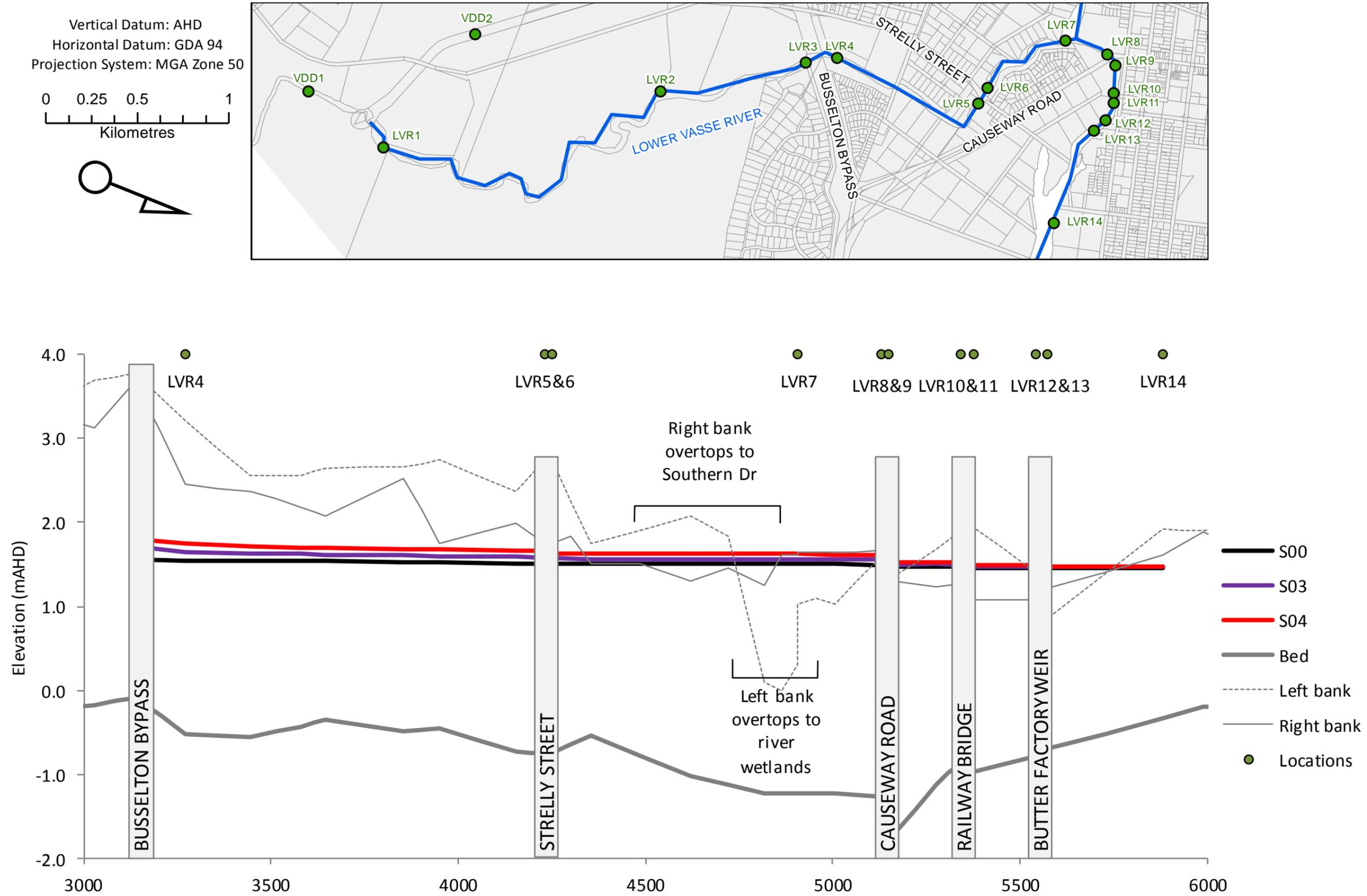
Figure 5-10: Long-section showing 1% AEP peak flood level for S00, S03 and S04 on the Lower Vasse River, Busseton Bypass to Butter Factory weir
