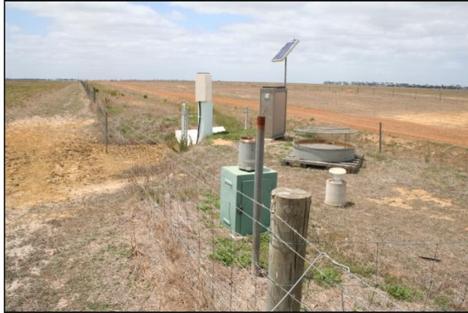
Figure 9 Gauging station equipment at the raised bed station
