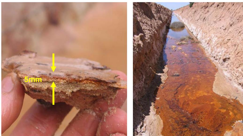
Figure 15 Iron oxide crust formation on lime-sand implicated in slowing neutralisation rates
