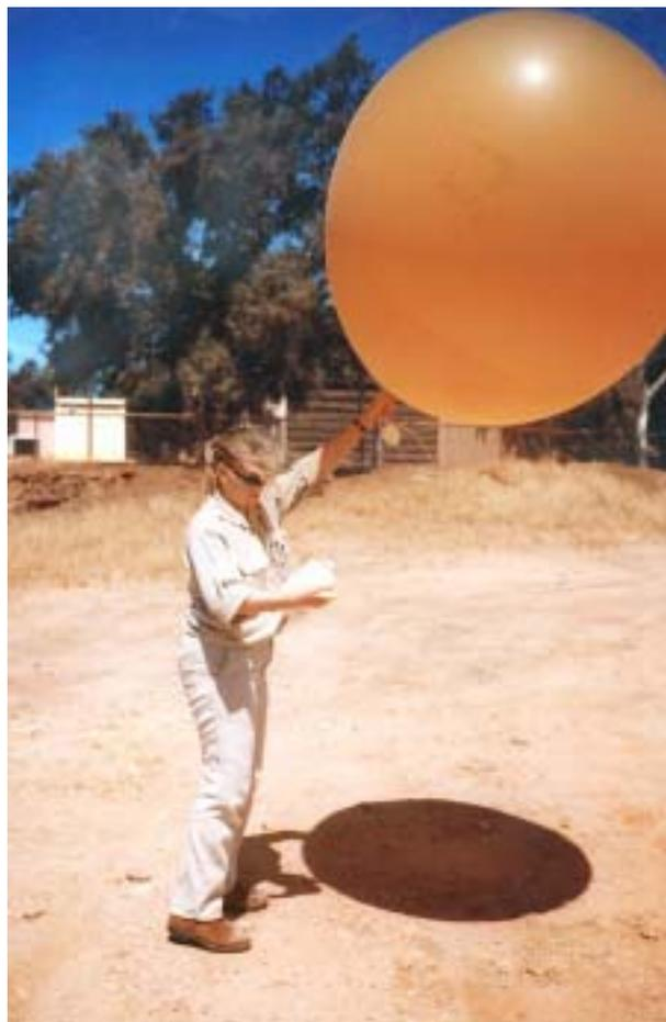
**Figure 5.3** A radiosonde balloon ready to be released at Dampier
