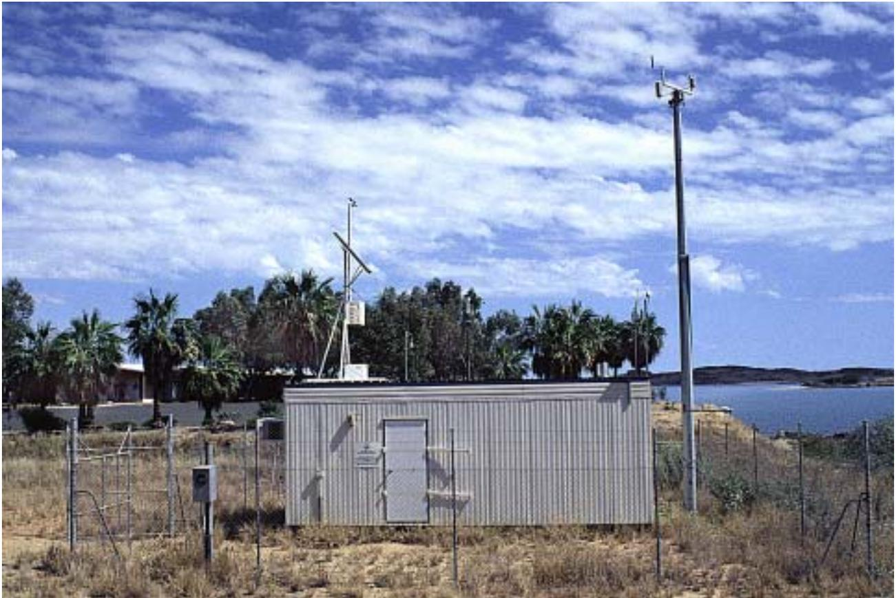
**Figure 2.3 Dampier air quality monitoring station**
