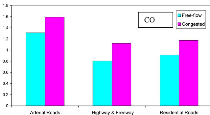
**Figure B3: Driving condition modification factors for diesel buses (PM, NOx, VOCs and CO)**
