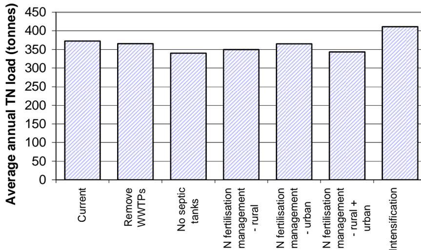
Figure 7.1 Estimated total TN loads from the Leschenault catchment for current land uses and the management scenarios – removal of WWTPs, removal of septic tanks, nitrogen fertilisation management in rural and urban areas, and intensification of dairy farming, horticulture and viticulture
