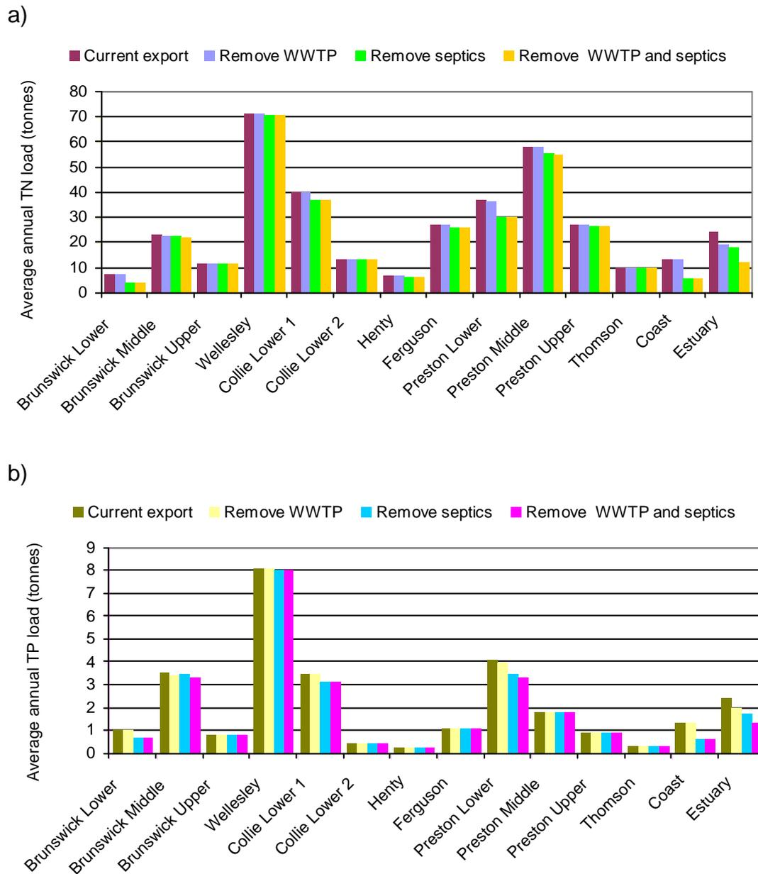
Figure 5.1 The predicted changes in a) average annual TN and b) average annual TP load due to the removal of WWTPs and septic tanks from the Leschenault catchment
