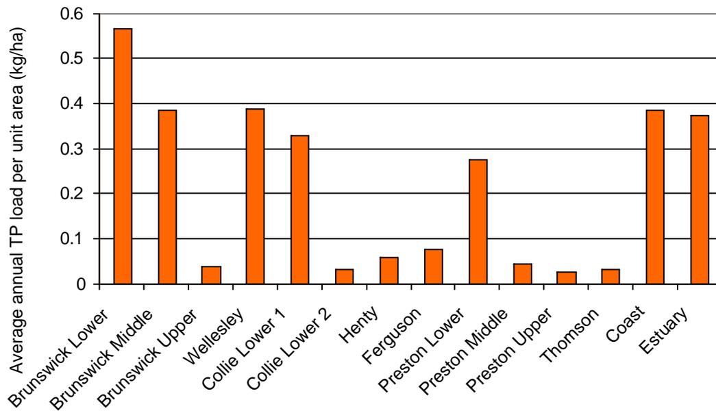
Figure 4.5 Average annual a) TP load (tonnes) and b) TP load per unit area (kg/ha) for the subcatchments of the Leschenault Estuary
