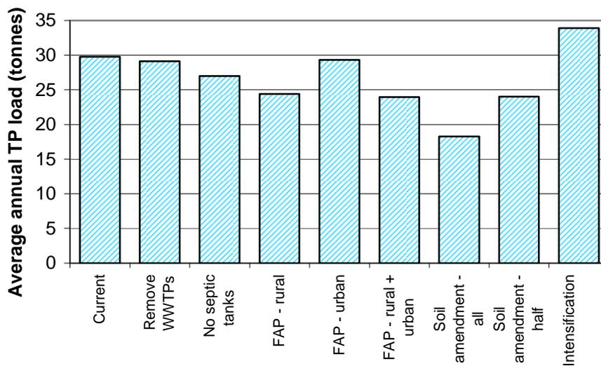
Figure 7.2 Estimated total TP loads from the Leschenault catchment for current land uses and the management scenarios – removal of WWTPs, removal of septic tanks, implementation of the Fertiliser action plan in rural and urban areas, application of soil amendment to low PRI soils, and intensification of dairy farming, horticulture and viticulture
