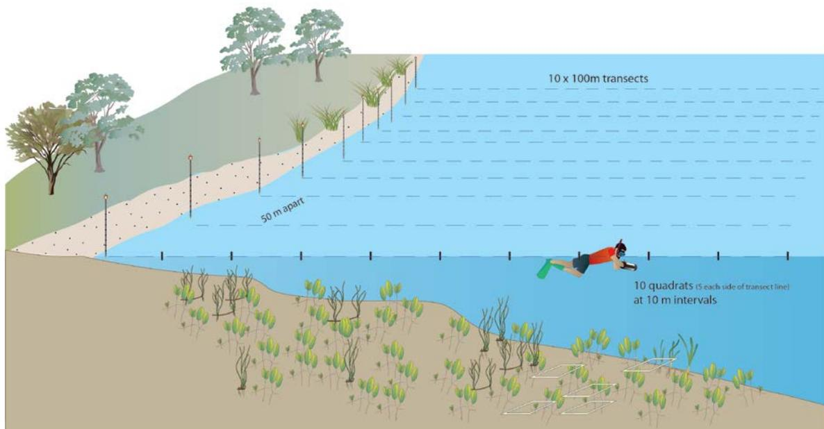
**Figure 12** Diagram of site layout: ten 100 m transects perpendicular to the shoreline are placed 50 m apart. Seagrass species and percentage cover, and water depth are recorded on snorkel from 10 randomly placed quadrats at 10 m intervals.
