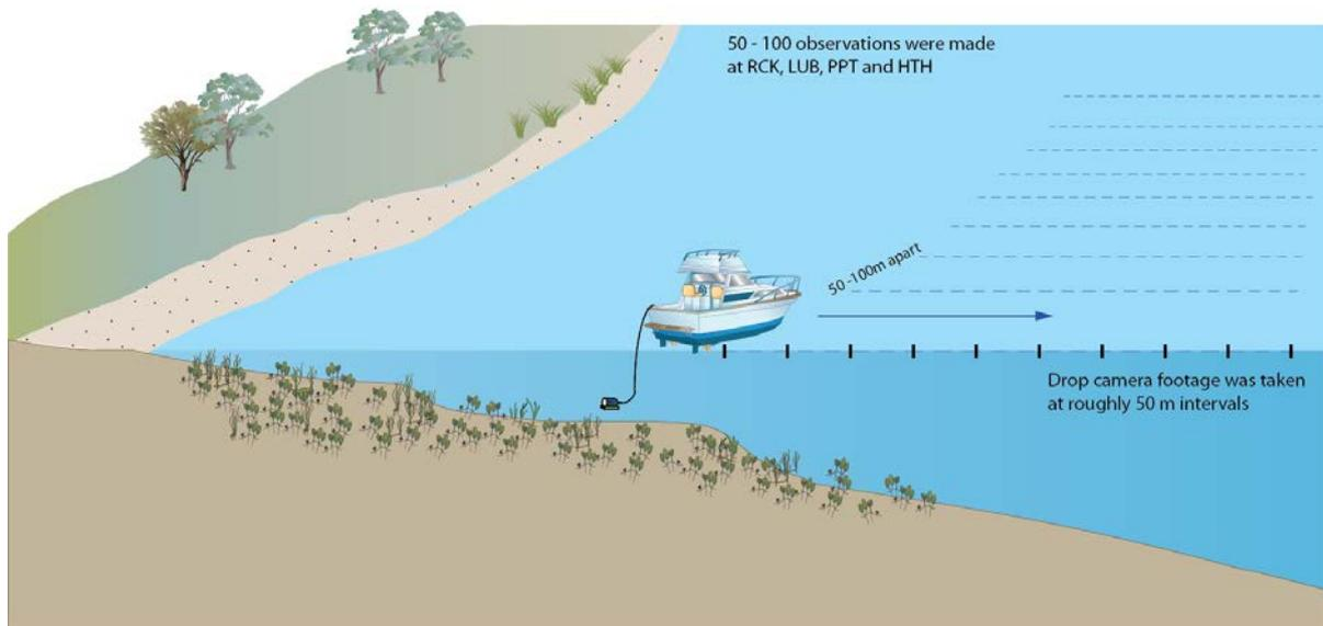
**Figure 13** *Diagram of site layout: seagrass species and percentage cover, and water depth are recorded from underwater video cameras. The camera was dropped approximately every 50 m from navigable point along shore to the depth extent of the seagrass.*
