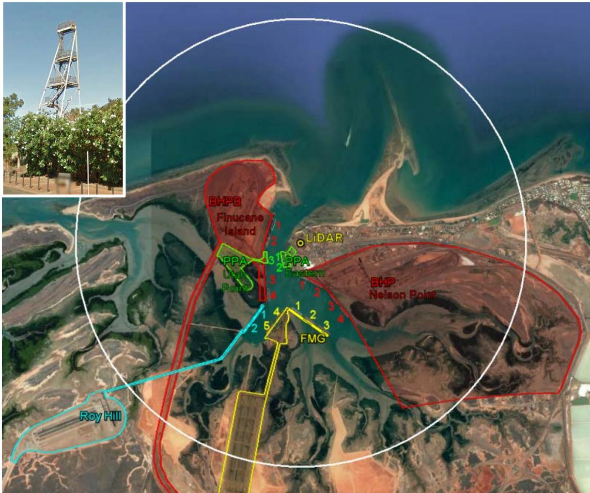
**Figure 1** Port Hedland with major operators BHP, FMG, PPA and Roy Hill outlined. The 5km radius white circle is centred on the LiDAR location atop the Town Centre Viewing tower (inset) and represents the approximate coverage of the LiDAR beam. Allocated loading berths are numbered.
