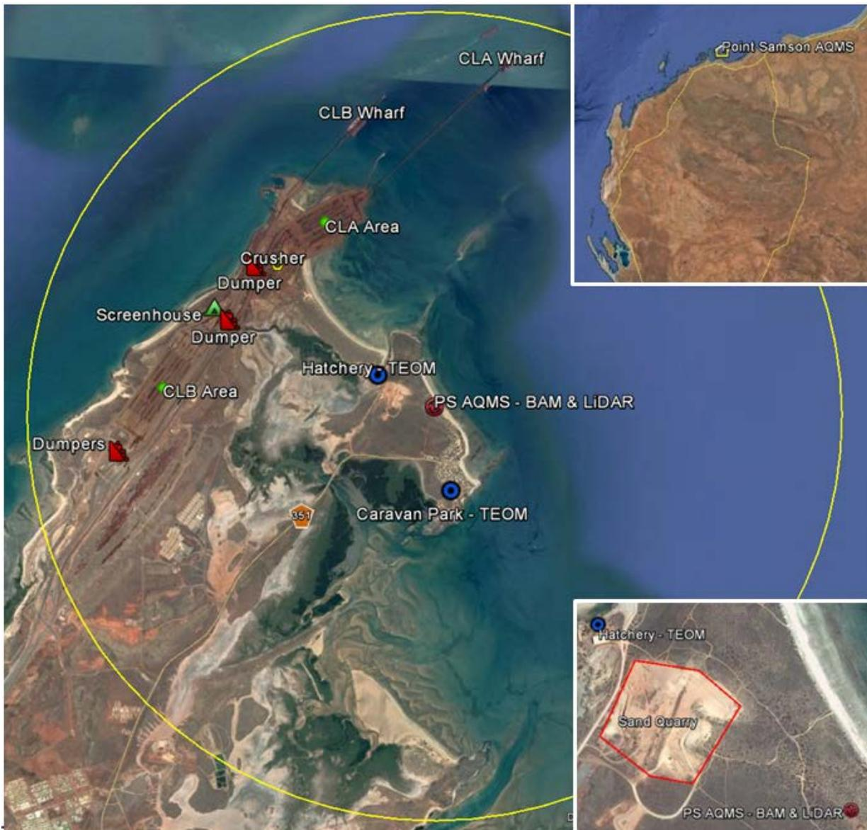
**Figure 1** Point Samson and Rio Tinto Cape Lambert operations with particle monitors marked. The yellow circle represents the approximate extent of the LiDAR beam. Insets show regional location (top right) and a close-up of the sand quarry area (lower right).
