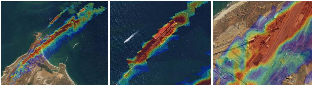
Figure 8 *LiDAR event record on 8 December 2016 at 6:40 am (left) showing ship loading (centre) and screenhouse (right) activities.*
