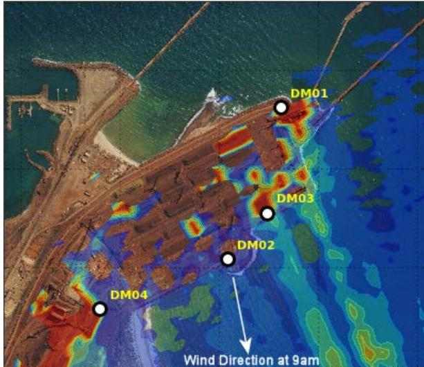
*Figure 10 LiDAR event record on 19 November 2016 at 9 am showing a number of active areas on Cape Lambert and locations of dust monitoring equipment*
