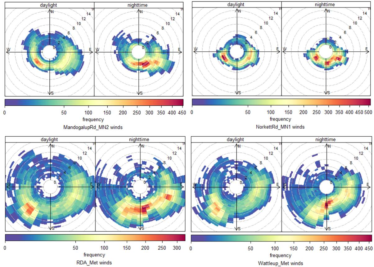
**Figure 8** Polar frequency plots of daylight and nighttime wind speed and direction during the study period for the four meteorological sites within the study area
