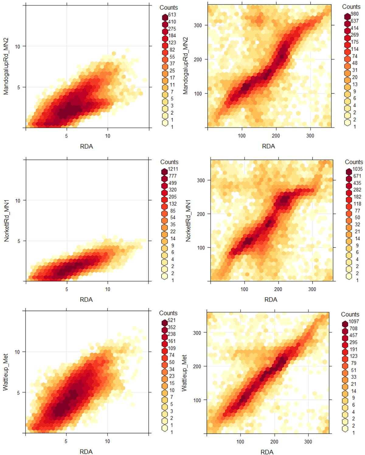
**Figure 9** Scatter plots showing the relationship between corresponding measurements of wind speed (left) and wind direction (right) between the RDA meteorological tower and Mandogalup (top), Norkett (centre) and Wattleup (bottom)
