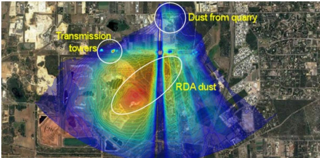
*Figure 14 Summed LiDAR signal with particle sources and hard objects located by LiDAR. The map colours, although representative of relative dust levels, do not represent actual concentrations.*
