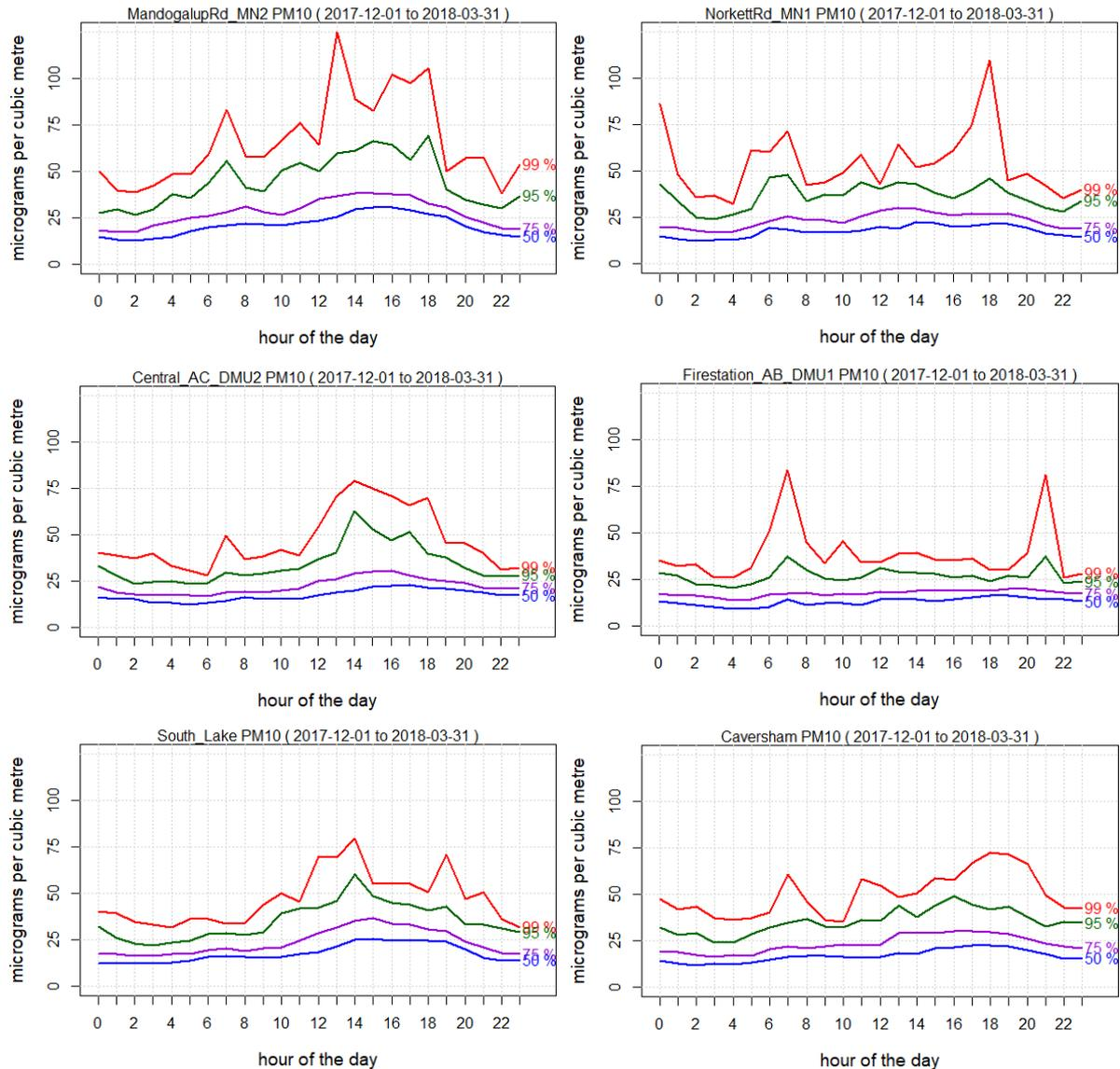
**Figure 6** Profile plot of one-hour averaged PM<sub>10</sub> for Mandogalup (top left), Norkett (top right), Central (mid left) and Firestation (mid right), South Lake (bottom left) and Caversham (bottom right)
