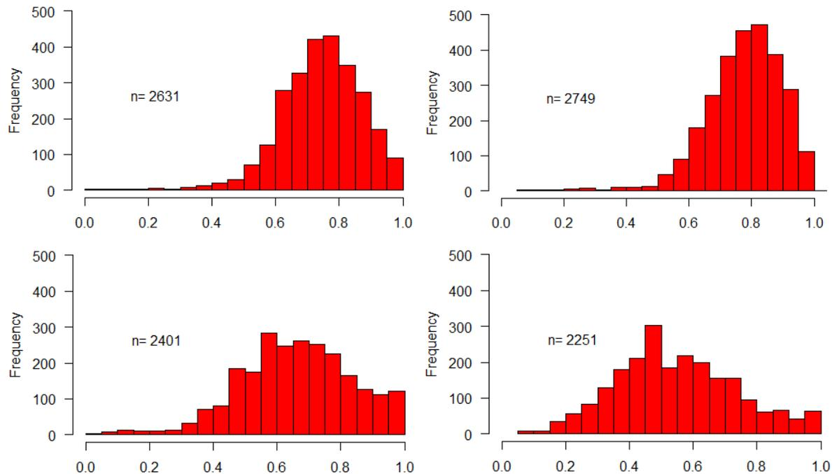
Figure 5 Frequency plot of the ratio of one-hour averaged  $PM_{10}$  to TSP for Mandogalup (top left), Norkett (top right), Central (bottom left) and Firestation (bottom right)
