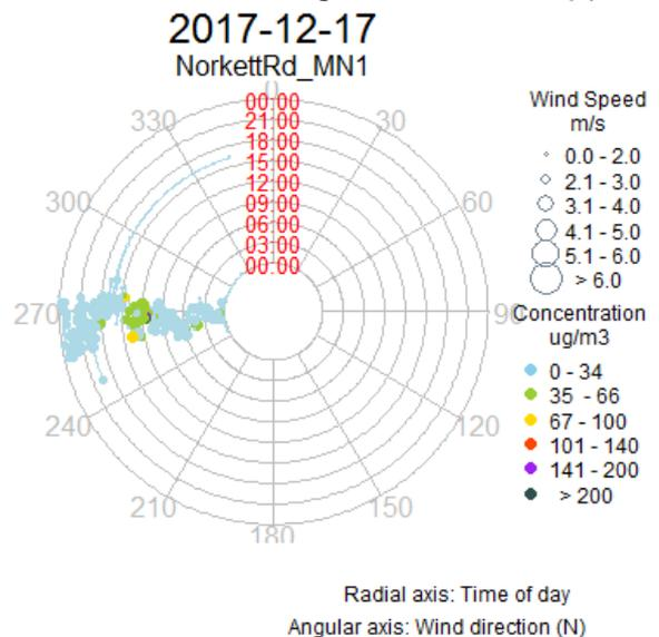
High particle concentrations at the Norkett site were caused by high winds combined with ride-on mower activity near the monitoring station.
