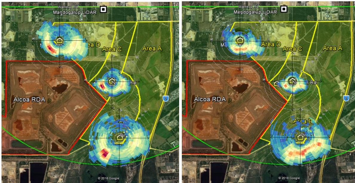
Figure 11 Mandogalup sites overlaid with the daylight (left) and nighttime (right) polar frequency plots for  $PM_{10}$  particles
