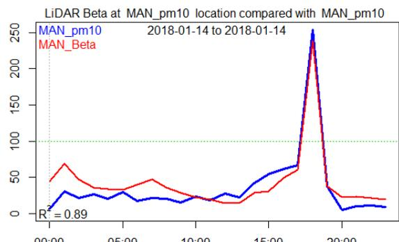
Comparing Beta data recorded by the LiDAR with PM<sub>10</sub> data recorded at Mandogalup (timeoffset=0, mult=2E8).
