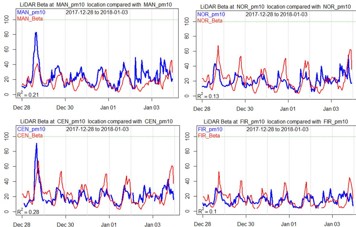
Figure 13 Comparing signals from the LiDAR with particle monitors located at Mandogalup (top left), Norkett (top right), Central (bottom left) and Firestation (bottom right)
