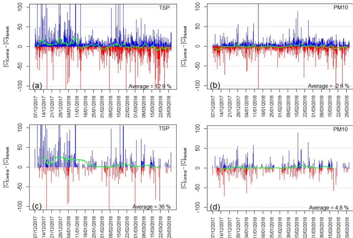
**Figure 3 Comparison of the difference in one-hour averaged particle concentrations between Central and Norkett over the study period (blue represents when  $[C]_{\text{Central}} > [C]_{\text{Norkett}}$  while red represents when  $[C]_{\text{Central}} < [C]_{\text{Norkett}}$ )**
