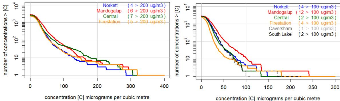
*Figure 2 Cumulative frequency plot for one-hour averaged TSP (left) and PM<sub>10</sub> (right) over the study period*
