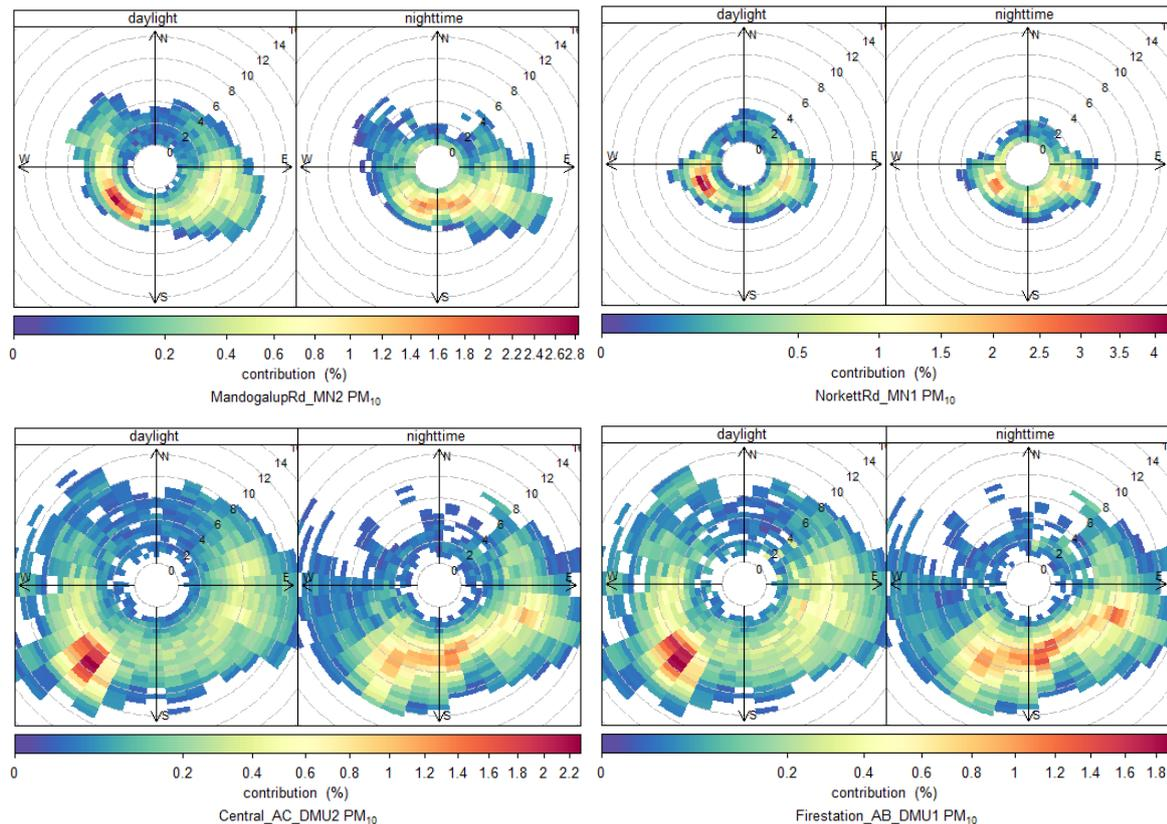
*Figure 10 Weighted mean polar frequency plots of  $PM_{10}$  particles during the study period for Mandogalup (top left), Norkett (top right), Central (bottom left) and Firestation (bottom right)*
