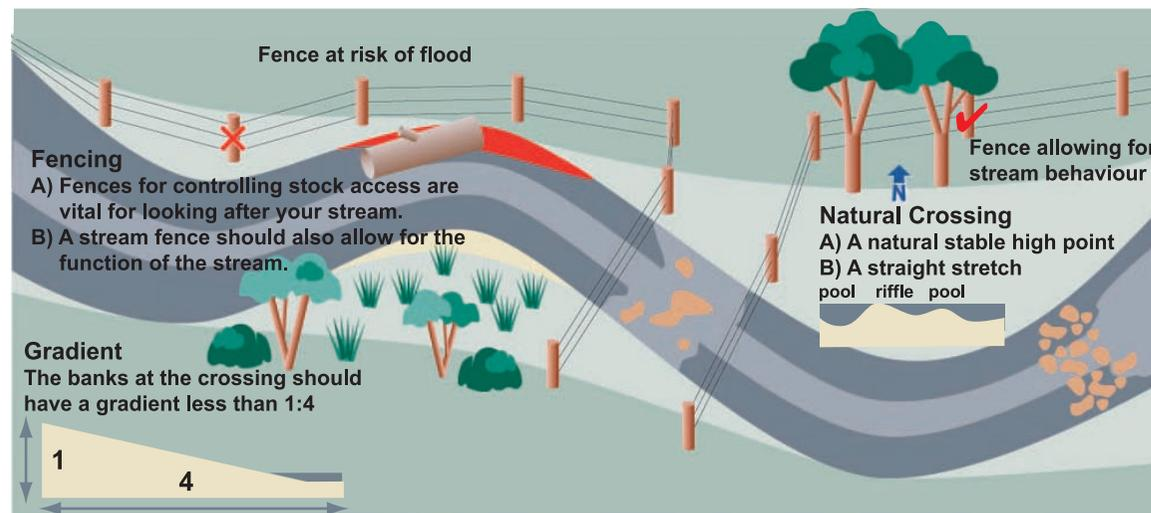
Figure 8 Design criteria for siting farm stream crossings
