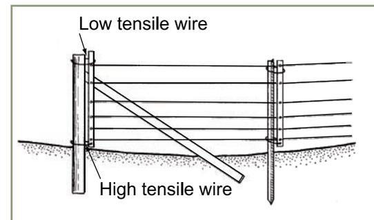
**Figure 4** Options for sacrificial or collapsible fencing suitable for flood conditions
