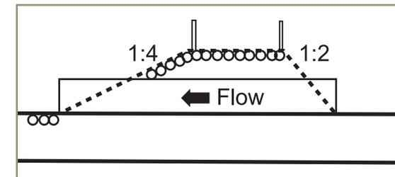
**Figure 9** Batter gradient for culvert crossings
