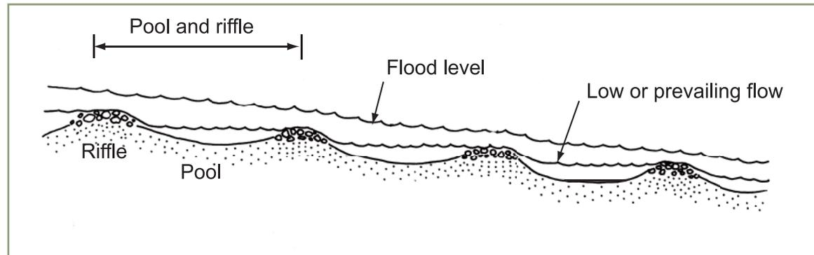
*Figure 7 A series of rock riffles
