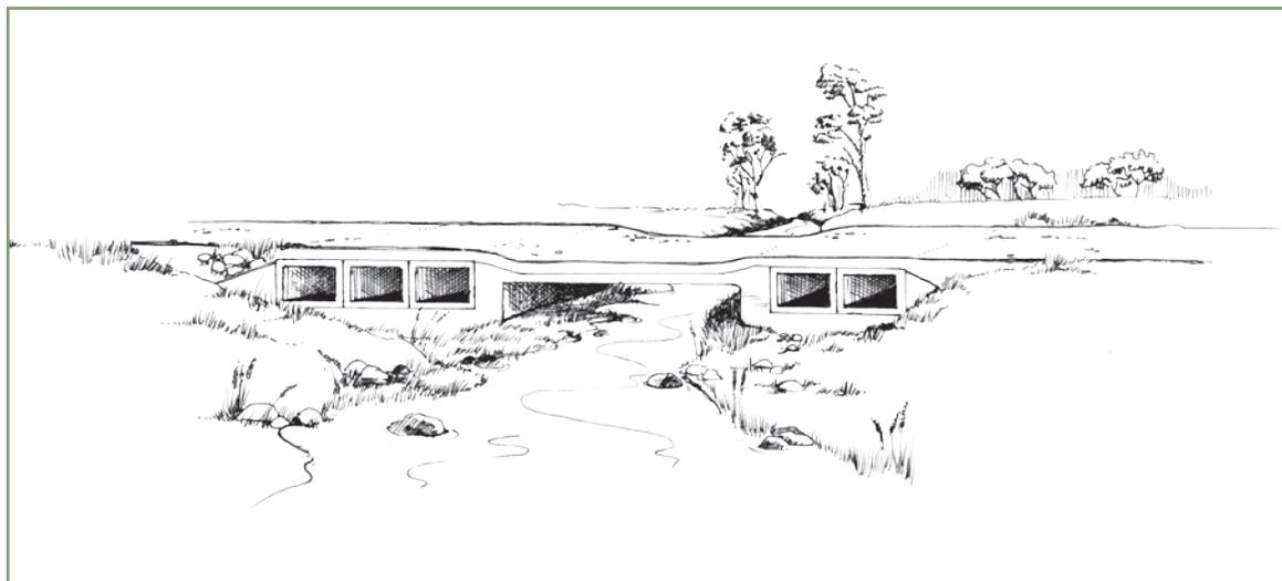
*Figure 10 Box culvert design for braided channel road crossings*
