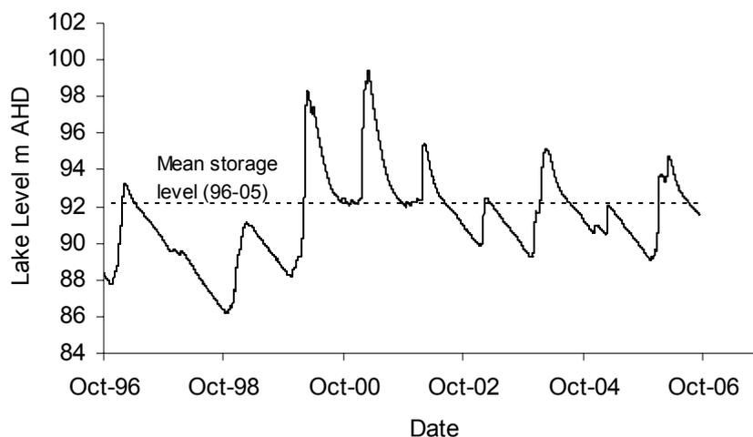
Figure 16 Fluctuations in the Lake Argyle water level
