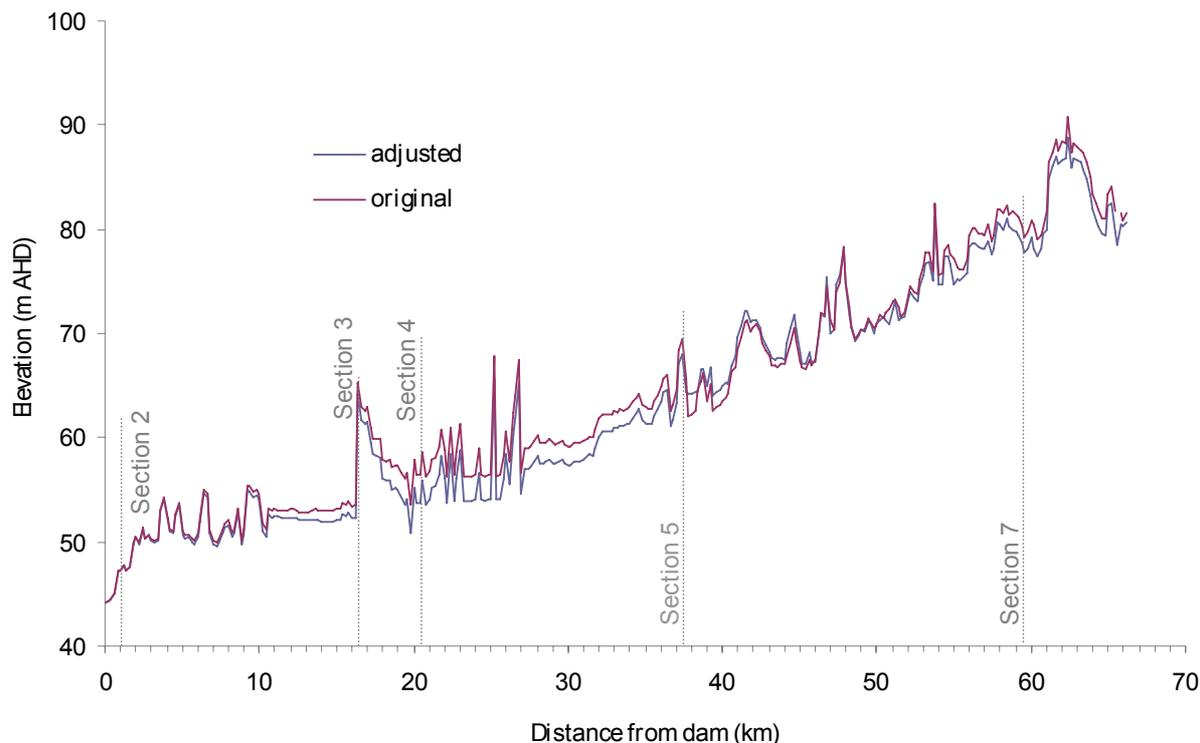
Figure 3 Adjustments made to the 1955/1961 pre-dam surface
