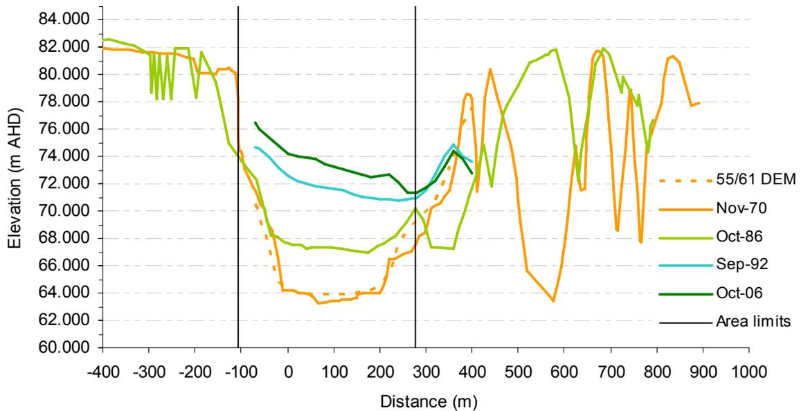
Figure 22 Cross section 5, 37.5 km upstream
