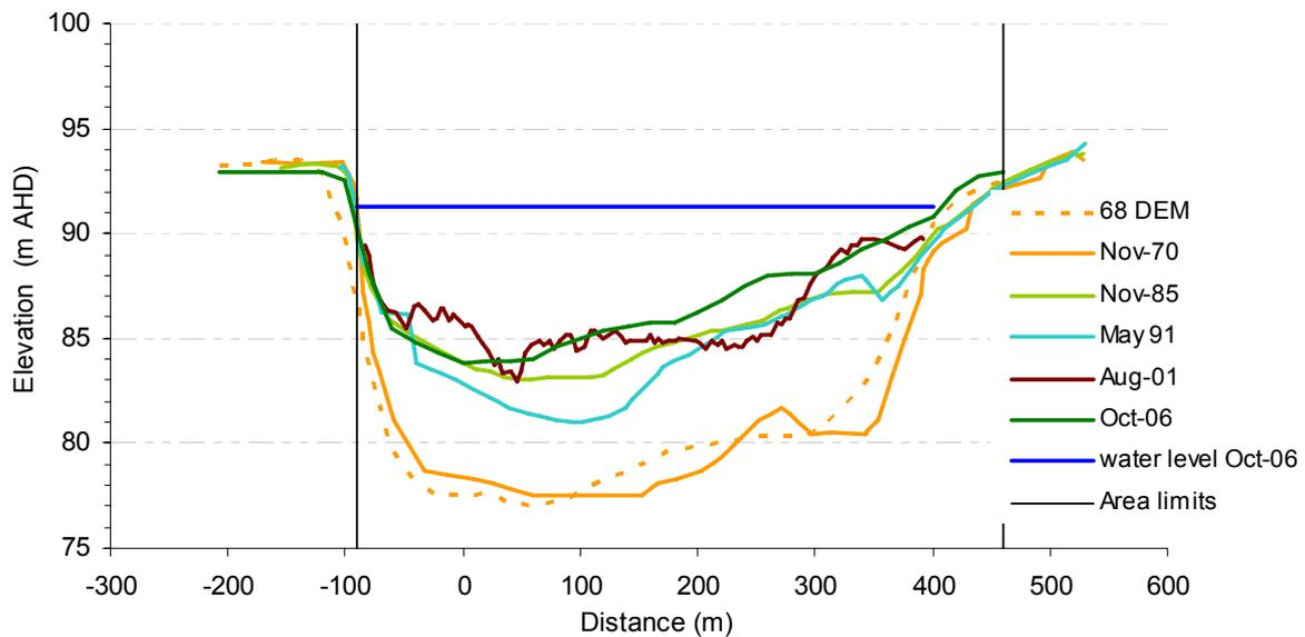
Figure 23 Cross section 7, 59.5 km upstream
