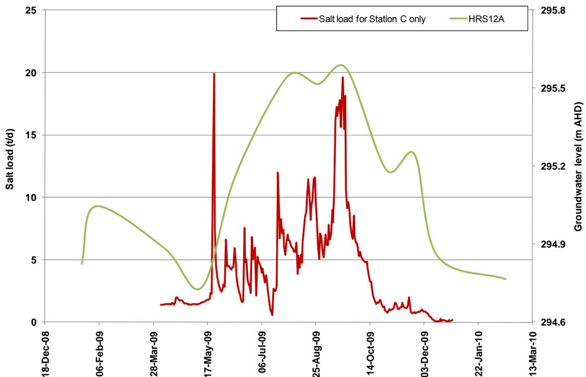
Figure 29 Comparison bore groundwater levels versus salt loads
