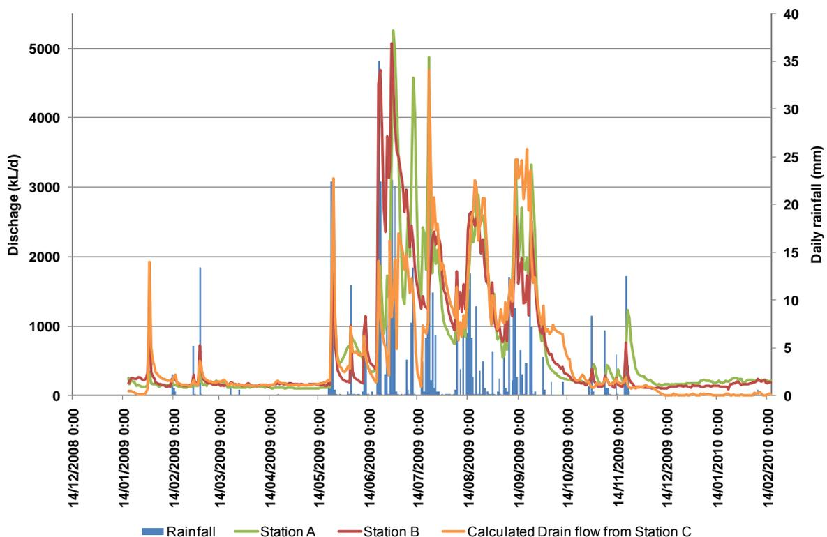
Figure 22 Calculated upper and lower drain discharges
