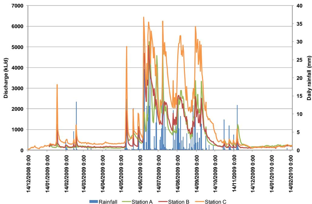
Figure 21 Raw daily discharge from Stations A, B and C
