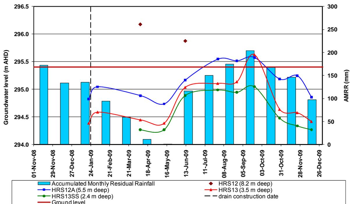
Figure 13 Comparison bores hydrograph with normalised AMRR
