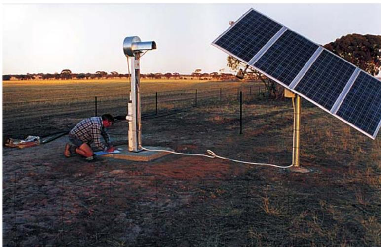
Figure 4 Solar panels powering an electric motor above the production bore at the Bodallin site
