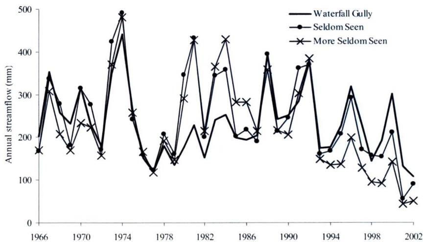
Figure 4. Observed annual streamflows of the Waterfall Gully, Seldom Seen and More Seldom Seen catchments
