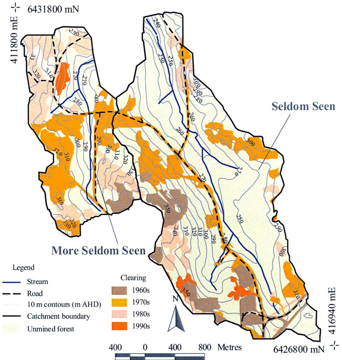
Figure 35. History of clearing for mining in the Seldom Seen catchments
