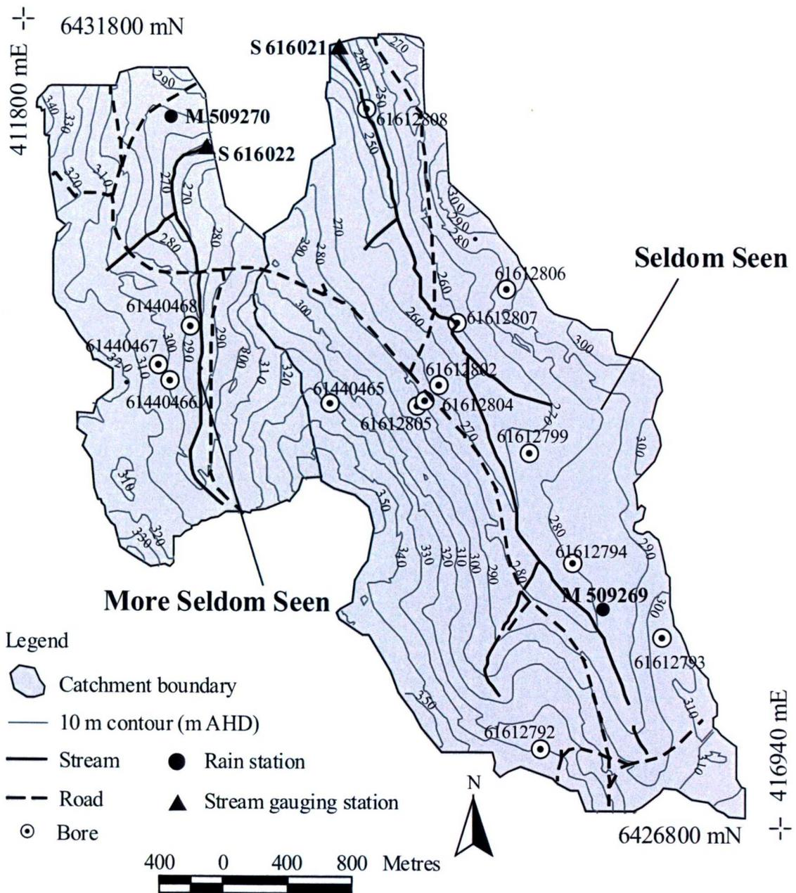
Figure 36. Topography and piezometer locations
