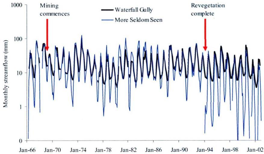
Figure 3. Monthly streamflows of the More Seldom Seen and Waterfall Gully catchments
