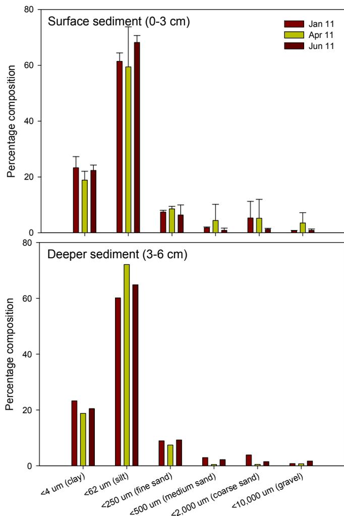
Figure 40 Particle size results for sediment near the KSW. For surface sediment (top) the average of three cores plus standard deviation is displayed.
