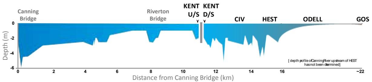
Figure 4 Distance from the weir and approximate channel depth at Canning River sampling sites.
