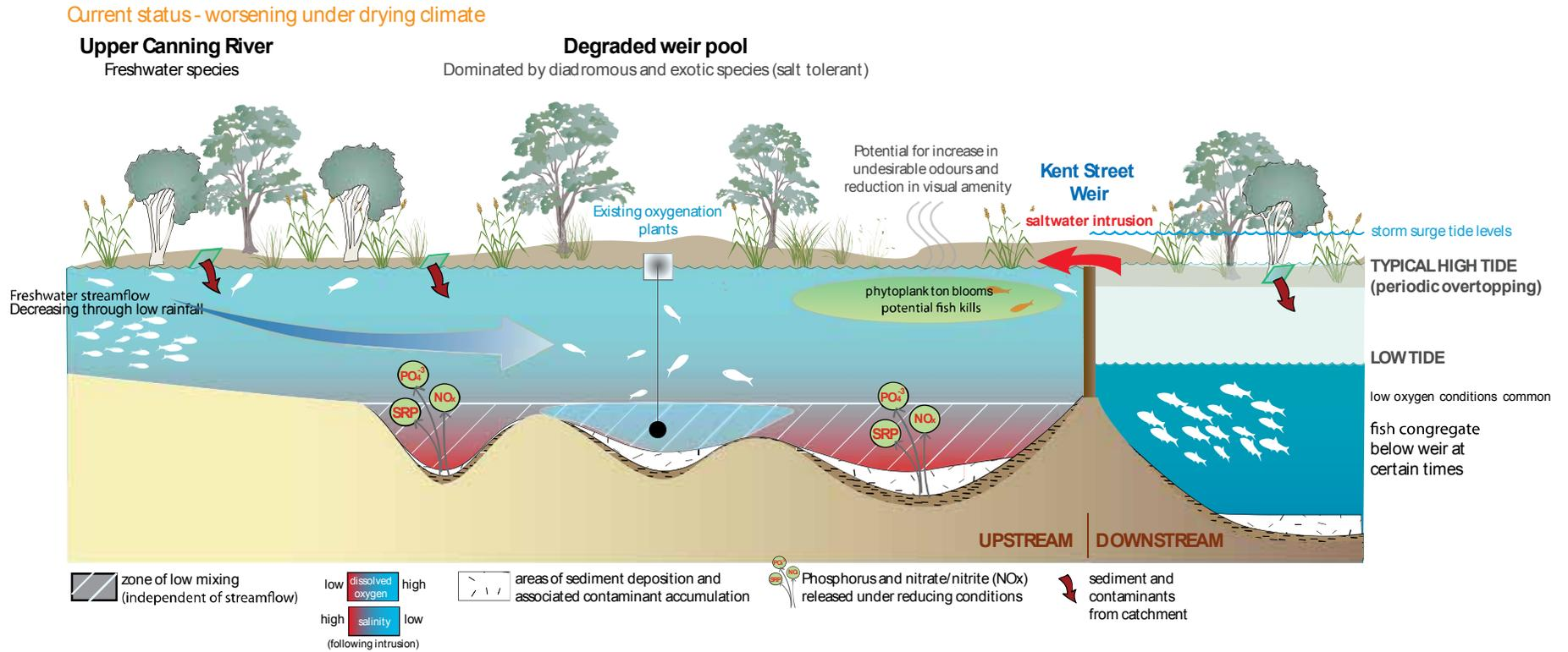
Figure 43 Conceptual diagram: KSW pool highlighting current water quality issues and impediments to flushing (existing oxygenation plant included).
