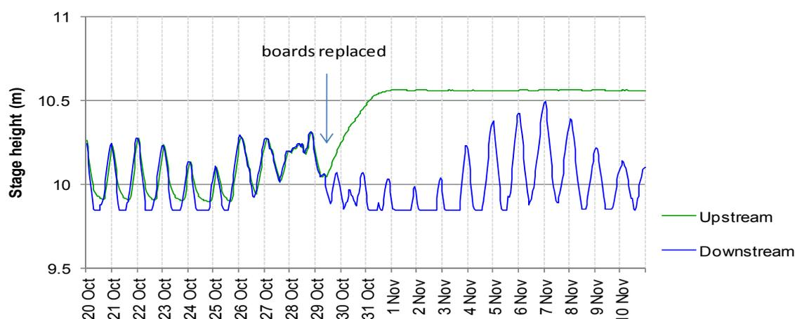
Figure 17 Water levels in the Canning River upstream and downstream of the KSW before and after replacement of the weir boards in 2009.
