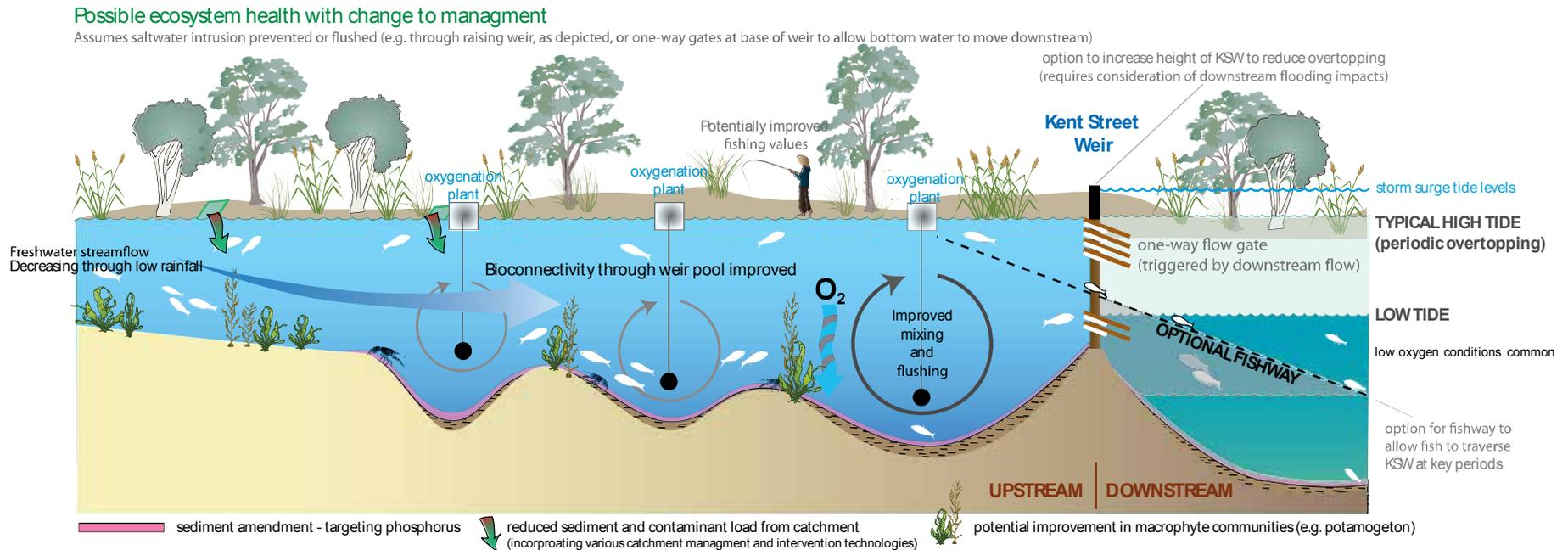
Figure 44 Conceptual diagram: KSW pool environment following implementation of management scenarios (assuming salt water upstream of KSW can be prevented or flushed quickly)
