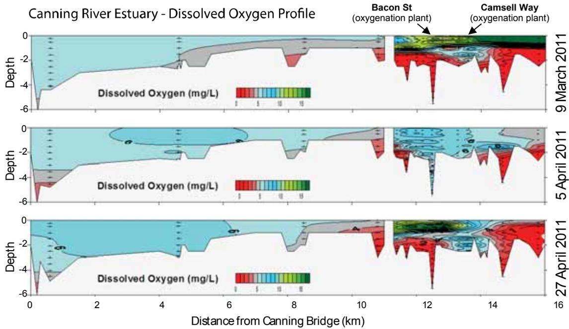
Figure 32 Examples of supersaturated oxygen layer above anoxic conditions throughout most of the Canning River study area above the KSW.
