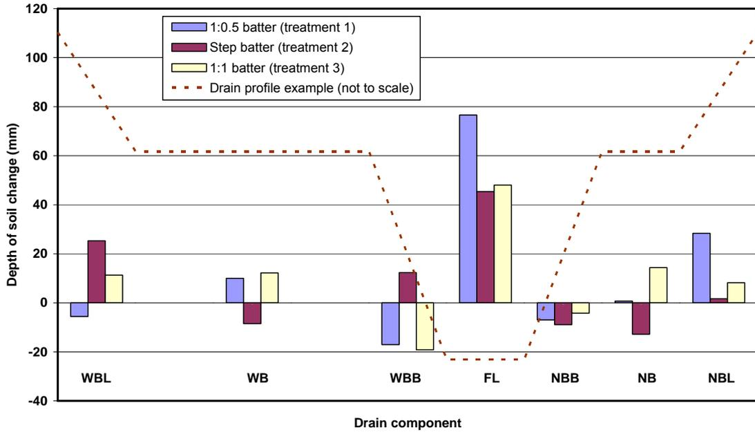
Figure 12 The average change in soil depth by drain component and treatment from survey 1 to 2
