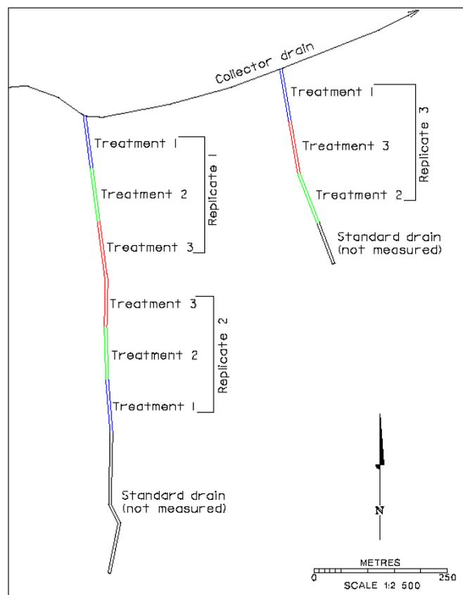
Figure 5 Layout drains and placement of treatments within each of the three replicates
