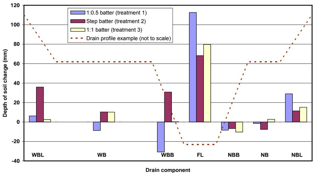
Figure 13 The average change in soil depth by drain component and treatment from survey 1 to 3
