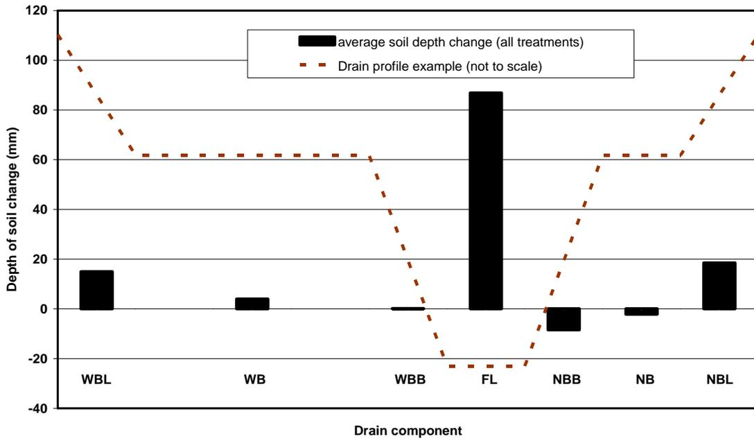
Figure 17 Average change in soil depth by drain component for all treatments from surveys 1 to 3
