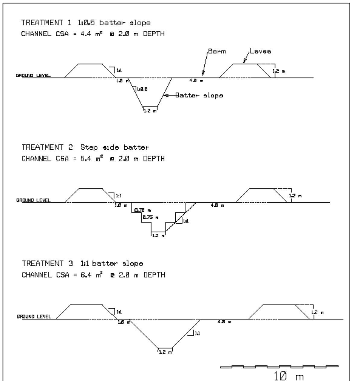
Figure 6 The three drain channel treatments
