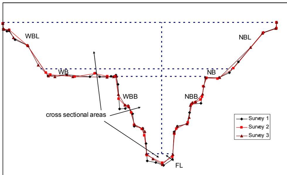
Figure 11 Profile of step batter drain showing cross sectional areas of drain components
