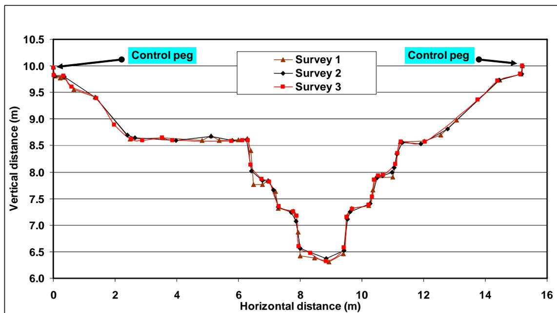
Figure 8 Cross section surveys at 25 m above downstream end of treatment 2 in replicate 1
