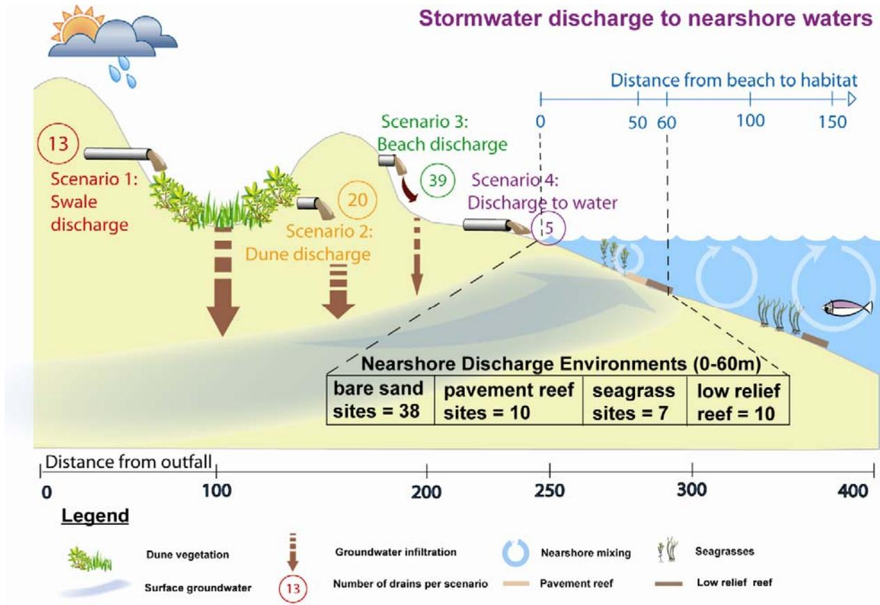
**Figure A 1. Conceptual model: fate of stormwater discharge in the Swan Coastal Region**
