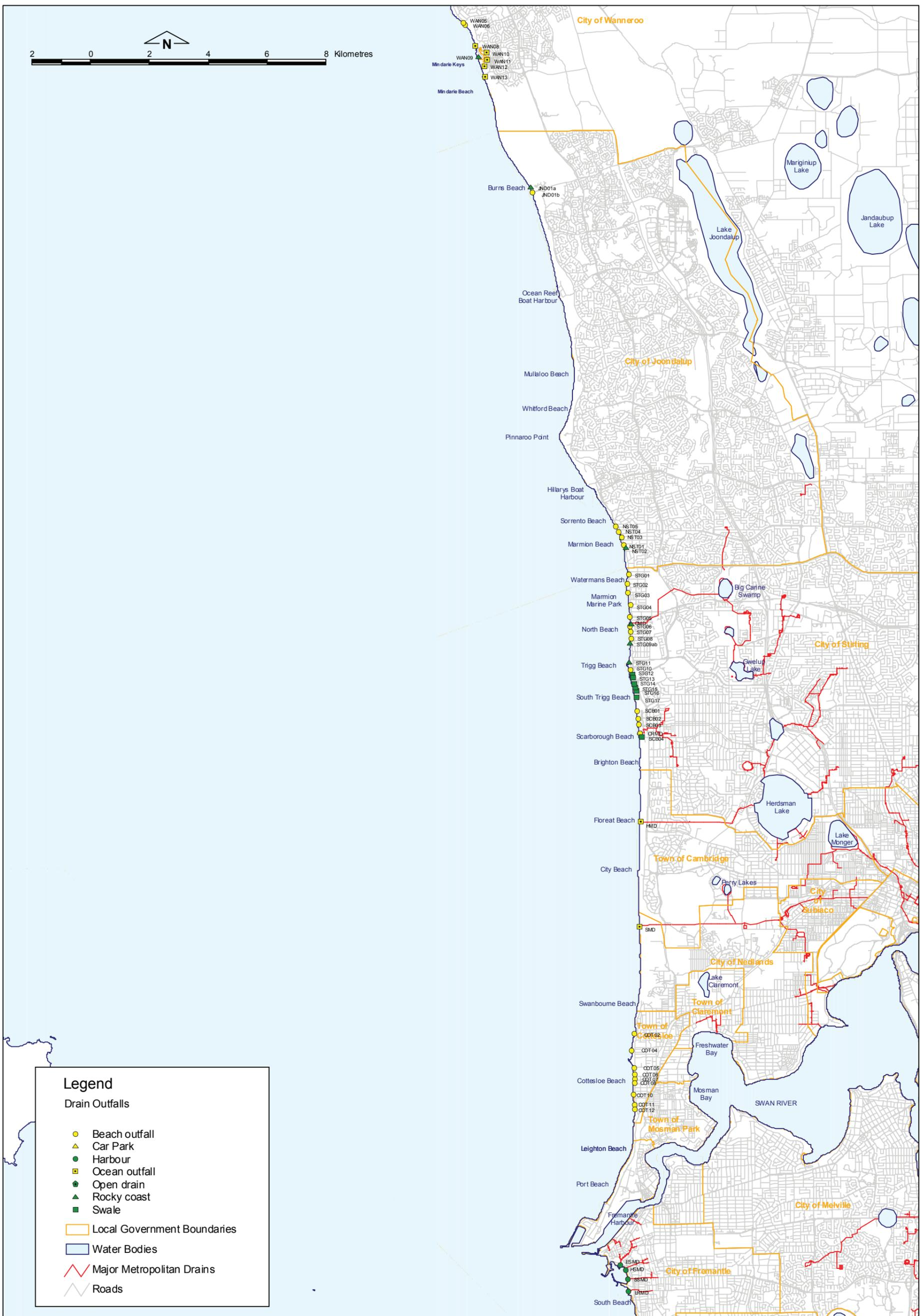
Figure A 2 Location of stormwater drains north of the Swan River: Wanneroo (WAN), Joondalup (JND), north Stirling (NST), Stirling (STG), Carine Main Drain (CMD), Scarborough (SCB), Colin Road Main Drain (CRMD), Herdsman Main Drain (HMD), Subiaco Main Drain (SMD), Cottesloe (COT), Essex Street MD (ESMD), Howard Street MD (HSMD), South Street MD (SSMD) and Lefroy Road MD (LRMD).
