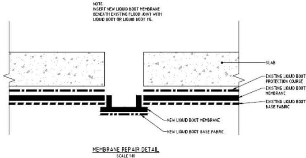
**FIGURE 2. POST CONCRETE REPAIR METHOD**
