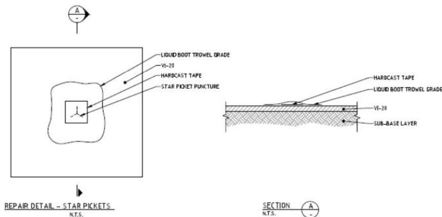
**FIGURE 1. REPAIR METHOD FOR STAR PICKETS**
