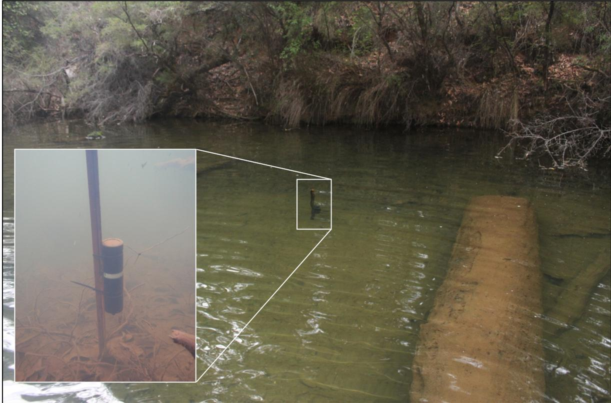
Figure 3 VEMCO VR2W 180kHz hydrophones in place at site HARV-07
