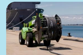
RAPID REEL™ Deployment, retrieval and storage system expediting shore power and flat fuel hose handling.
