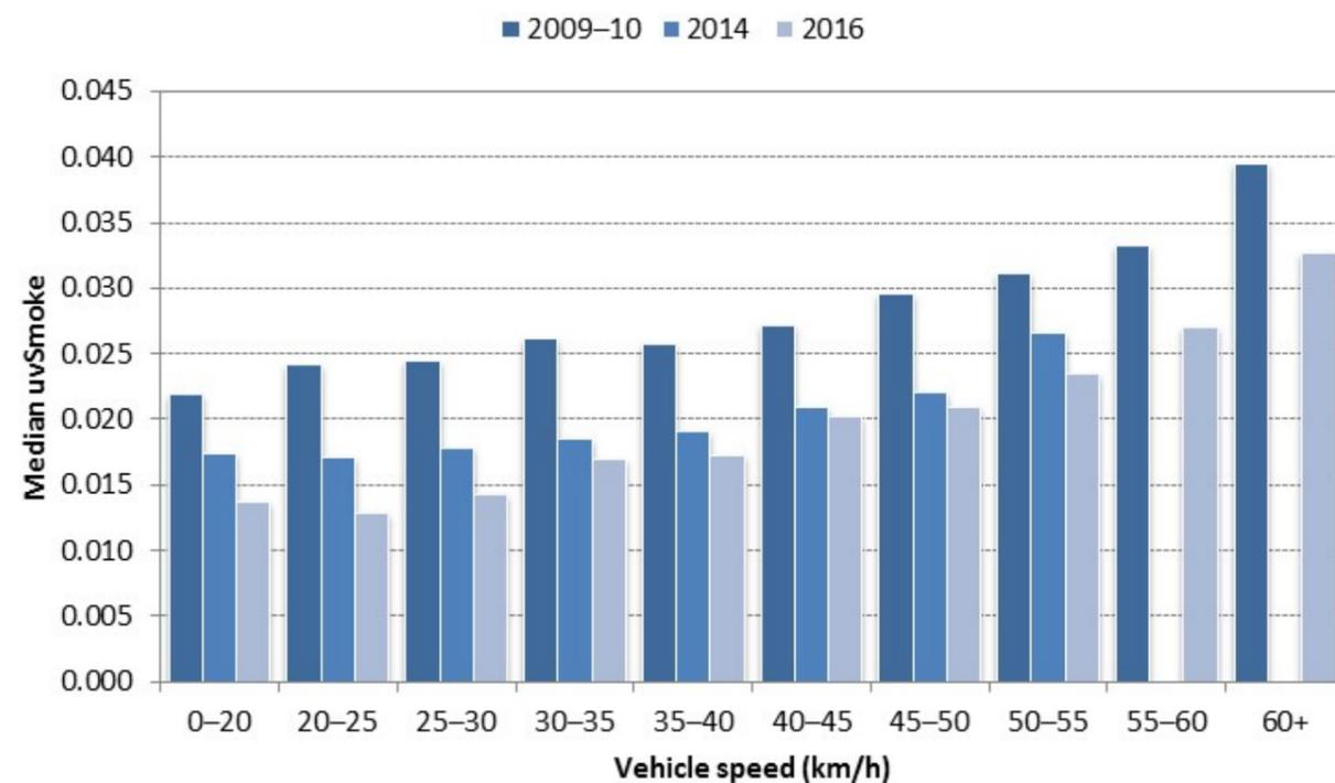
Figure 5: Median emissions over time per vehicle speed<sup>4</sup>
