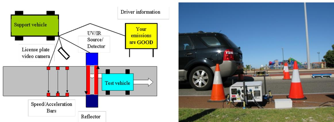
**Figure 2: Schematic diagram of the RSD monitoring equipment<sup>1</sup> (left) and RSD source/detector and reflector in operation<sup>2</sup> (right)**
