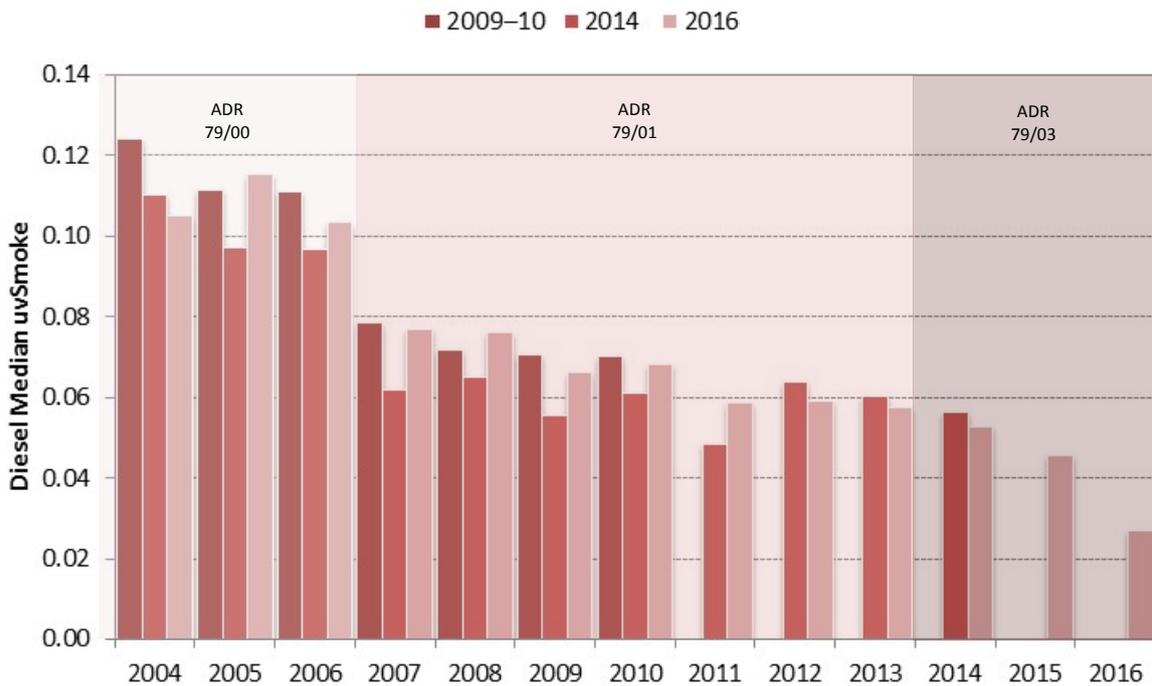
Figure 14: Median smoke emissions over time per year of manufacture
