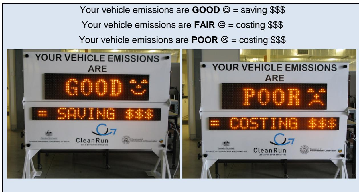
The score that appears on the smart sign is the lowest from all tested emissions. If any substance is rated as POOR, the vehicle receives a POOR. Similarly, if any substance is rated FAIR, the vehicle gets a FAIR. Only if all measured substances receive a GOOD rating will the vehicle be rated as GOOD.
